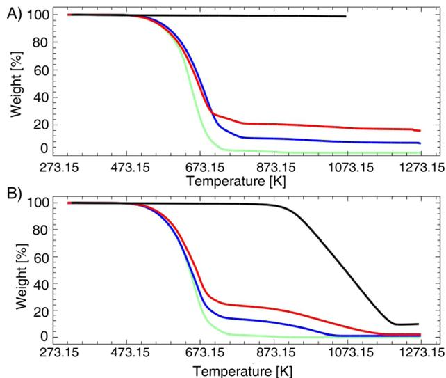
Fig. 5 Thermogravimetric (TGA) curves, recorded under combustional (B) versus pyrolytic (N<sub>2</sub>) (A) conditions, for the neat paraffin (green), 10 wt% (blue), 20 wt% (red) Fe@MWCNT composites, and pristine Fe@MWCNTs (black).
