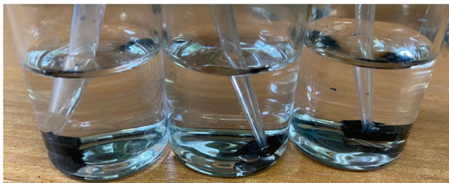
Fig. 3 Photograph of a paraffin + 20 wt% Fe@MWCNT composite after a 24 h treatment with 1 M aqueous solutions of NaCl, NaOH, and HCl (from left to right) confirming the composite's durability in the corroding environments.
