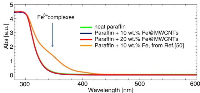
Fig. 7 Ultraviolet-visible light (UV-Vis) spectra of samples treated by a strongly aggressive medium composed from H<sub>2</sub>O<sub>2(aq)</sub> (30%), CH<sub>3</sub>COOH (99.5%), and H<sub>2</sub>SO<sub>4(aq)</sub> (96%), (v/v/v = 5 : 5 : 0.1) recorded after one month: neat paraffin (green), 10 wt% Fe@MWCNTs (blue), 20 wt% Fe@MWCNTs (red), Fe-paraffin from ref. 50 (orange).
