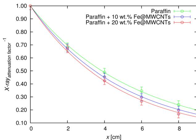
Fig. 12 Dependence of the X-ray<sub>attenuation factor</sub><sup>-1</sup> for different thicknesses (2, 4, 6, and 8 cm) for the pure paraffin and paraffin-based composites with 10 wt% and 20 wt% addition of Fe@MWCNTs at the 70 kV anode voltage. The symbols present the experimentally-achieved data, while the lines present the eqn (7) fitting data.
