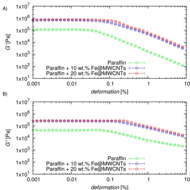
Fig. 8 Storage ( $G'$ ) (A) and loss ( $G''$ ) (B) moduli as a function of deformation for various mass fractions of nanotubes in nanocomposites at a constant temperature  $T = 309.75$  K and an oscillation frequency of 1 Hz.
