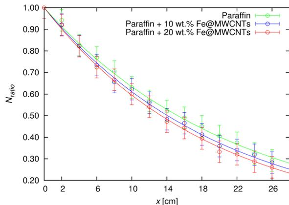
**Fig. 10** Ratio of the number of detected photons in the G–M counter for each of the examined layer thicknesses (from 2 to 26 cm with a 2-cm-step) versus the number of photons collected without any layer on the paraffin-based composite thicknesses with 10 wt% and 20 wt% addition of Fe@MWCNTs. The symbols and lines represent the experimental and eqn (5) fitting data, respectively.
