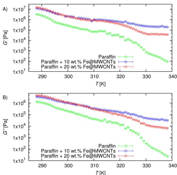
Fig. 9 Storage ( $G'$ ) (A) and loss ( $G''$ ) (B) moduli as a function of temperature for various mass fractions of nanotubes in nanocomposites at a constant deformation of 0.01% and an oscillation frequency of 1 Hz.
