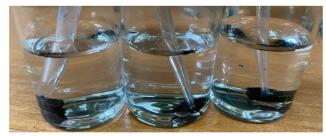
Fig. 3 Photograph of a paraffin + 20 wt% Fe@MWCNT composite after a 24 h treatment with 1 M aqueous solutions of NaCl, NaOH, and HCl (from left to right) confirming the composite's durability in the corroding environments.
