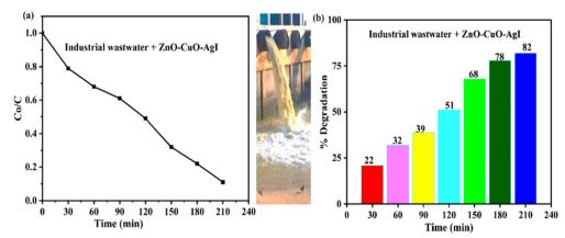
Fig. 16 Plots of (a)  $C_0/C$  versus time, and (b) % degradation versus time of wastewater analysis of the ZnO-AgI-CuO nanocomposite.
