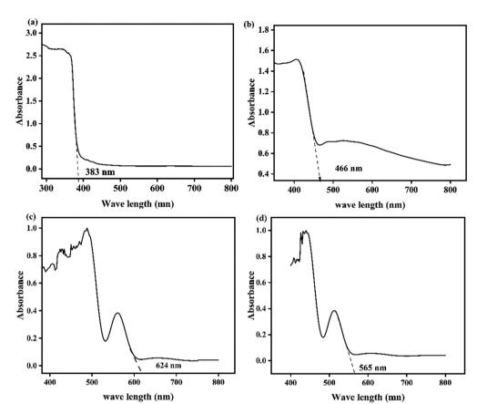
UV-vis analysis of (a) ZnO, (b) AgI, (c) CuO, and (d) the ZnO-AgI-CuO nanocomposite
