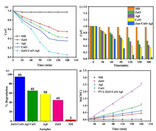
Fig. 11 (a)  $C/C_0$  versus time in min, (b)  $C/C_0$  versus time in min at each 30 min interval, (c) highest % degradation, and (d) kinetic rate of MB as a function of time using 10 mg of MB and 110 mg of ZnO-AgI-CuO nanocomposite under visible light irradiation.
