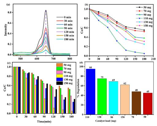
Fig. 13 (a) UV spectra, (b) and (c) 110 mg of catalyst load concentration, and (d) % degradation efficiency of the ZnO-AgI-CuO nanocomposite.
