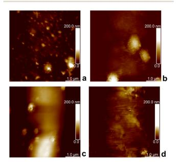
Fig. 3 PF-QNM topography height images of P2HPG-Tyr microgels on mica substrate (a), (b) and glass substrate (c), (d), swollen in Q-H<sub>2</sub>O (a), (c), and PBS buffer (b), (d)
