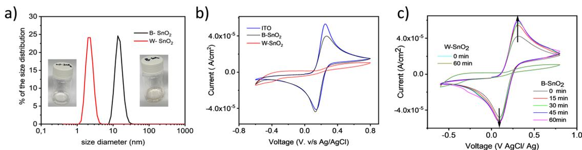
Fig. 7 (a) Dynamic light scattering of SnO<sub>2</sub> particles (b) cyclic voltammograms of different SnO<sub>2</sub> films on ITO in comparison with bare ITO (c) cyclic voltammogram of SnO<sub>2</sub> films at different time intervals.
