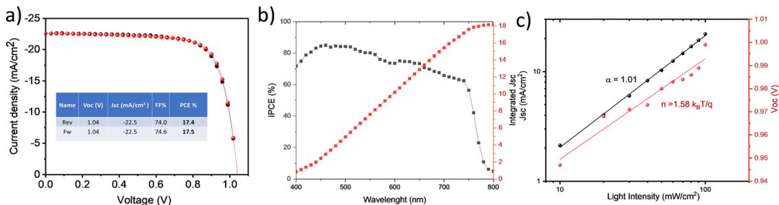
Fig. 8 (a) Champion JV curve of W-SnO<sub>2</sub> with KF (b) IPCE spectra of the best cell (c) J<sub>sc</sub> and V<sub>OC</sub> vs. light intensity curve.
