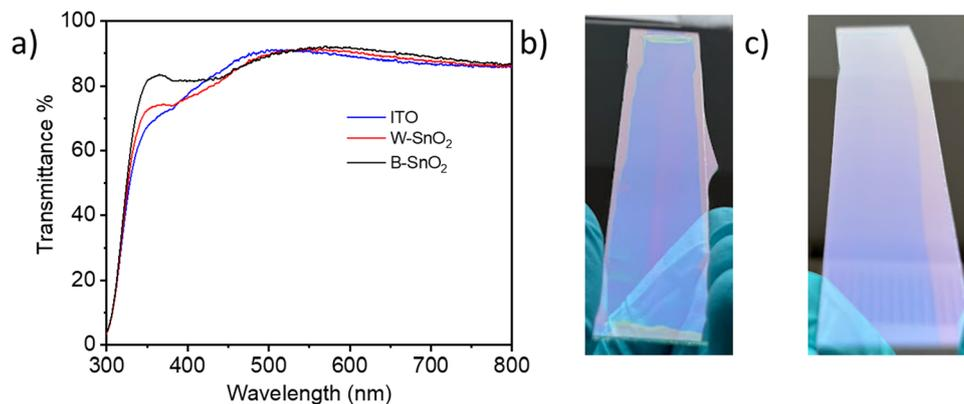
Fig. 2 (a) Transmittance spectra of slot die coated  $\text{SnO}_2$  films on ITO-glass substrates. Photographic images of the corresponding films ( $14 \text{ cm} \times 3 \text{ cm}$ ): (b)  $\text{W-SnO}_2$  (c)  $\text{B-SnO}_2$ .
