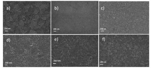
Fig. 3 Scanning electron microscopy surface images of (a) ITO substrate (b) W-SnO<sub>2</sub> on ITO (c) B-SnO<sub>2</sub> on ITO. (d)-(f) MAPbI<sub>3</sub> films deposited on (a)-(c) respectively.
