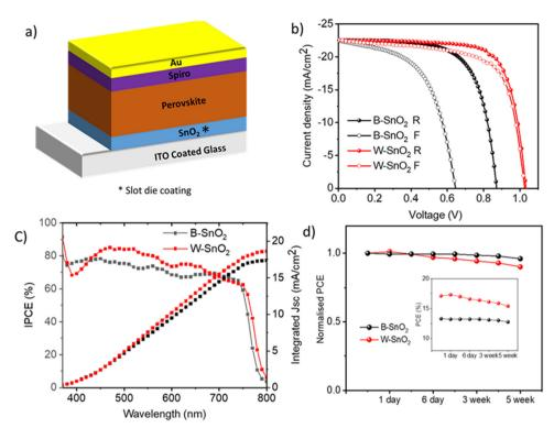
Fig. 5 (a) N-i-p solar cell architecture; (b) champion JV curves for devices with slot-die coated SnO<sub>2</sub> as electron transport layers; (c) IPCE spectra (d) normalized storage stability (inset actual stability over several weeks).
