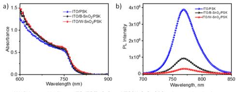
Fig. 4 (a) UV-Vis spectra of MAPbI<sub>3</sub> perovskite films on ITO, ITO/B-SnO<sub>2</sub> and ITO/W-SnO<sub>2</sub>. (b) Steady-state photoluminescence spectra the same films.
