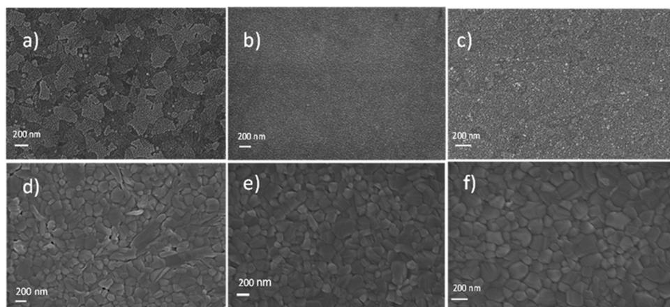
Fig. 3 Scanning electron microscopy surface images of (a) ITO substrate (b)  $\text{W-SnO}_2$  on ITO (c)  $\text{B-SnO}_2$  on ITO. (d)–(f)  $\text{MAPbI}_3$  films deposited on (a)–(c) respectively.
