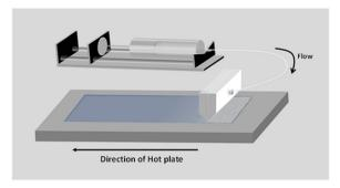
Fig. 1 Schematic representation of slot-die coating of SnO<sub>2</sub> solution.
