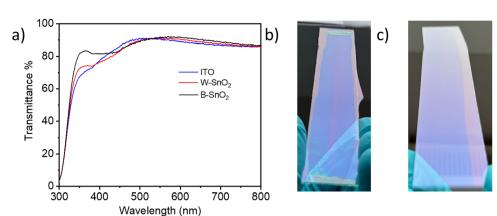
Fig. 2 (a) Transmittance spectra of slot die coated SnO<sub>2</sub> films on ITO-glass substrates. Photographic images of the corresponding films (14 cm × 3 cm): (b) W-SnO<sub>2</sub> (c) B-SnO<sub>2</sub>.
