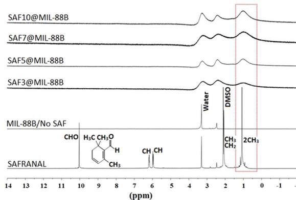
Fig. 3 <sup>1</sup>H NMR spectra of pure MIL-88B(Fe) and SAF@MIL-88B(Fe) nanostructures containing 3, 5, 7, and 10% SAF as compared with that of pure SAF, demonstrating the continued existence of SAF within the MIL-88B(Fe) nanostructures.
