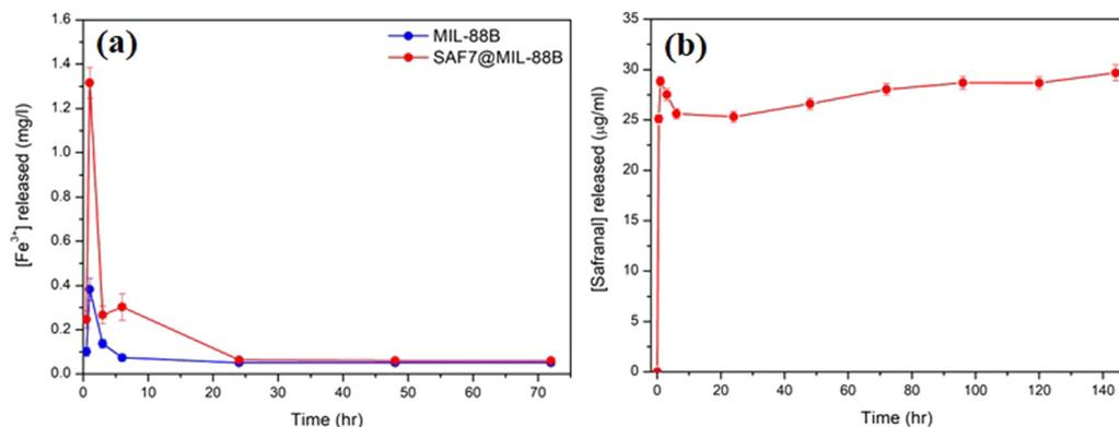
Fig. 7 (a) ICP analysis of the release of Fe<sup>3+</sup> ions from pure MIL-88B(Fe) and SAF7@MIL-88B(Fe) after incubating in 1X PBS for up to 72 hours. (b) UV-VIS analysis of the release of Safranal from SAF7@MIL-88B(Fe) after incubating in 1× PBS for up to 144 hours.
