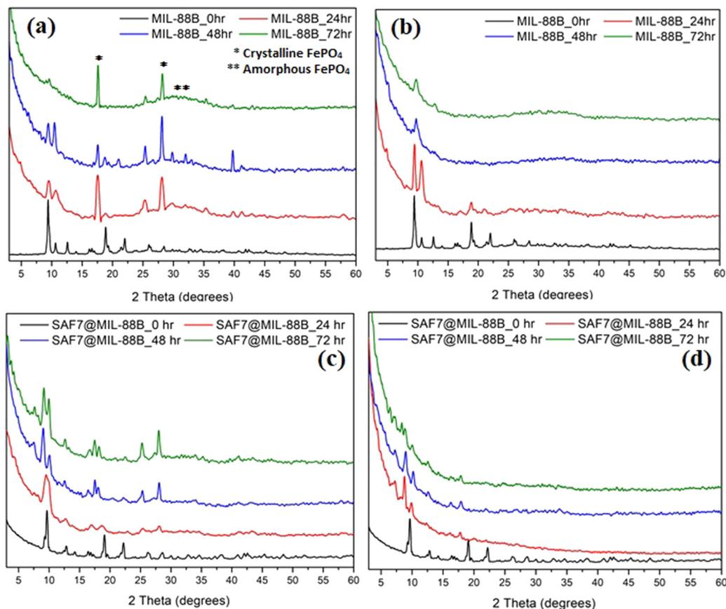
Fig. 5 XRD patterns of MIL-88B(Fe)(a), (b) and SAF7@MIL-88B(Fe) (c), (d) after incubation in PBS (a), (c) and RPMI (b), (d) media for 0, 24, 48 and 72 hours at  $37^\circ\text{C}$ .
