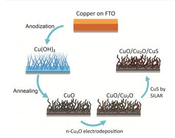
Scheme 1 Summary of the experimental procedure to produce nanostructured films of CuO/Cu<sub>2</sub>O/CuS.
