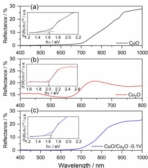
Fig. 3 Diffuse reflectance spectrum and Tauc plot of (a) CuO, (b) Cu<sub>2</sub>O and (c) CuO/Cu<sub>2</sub>O -0.1 V films.
