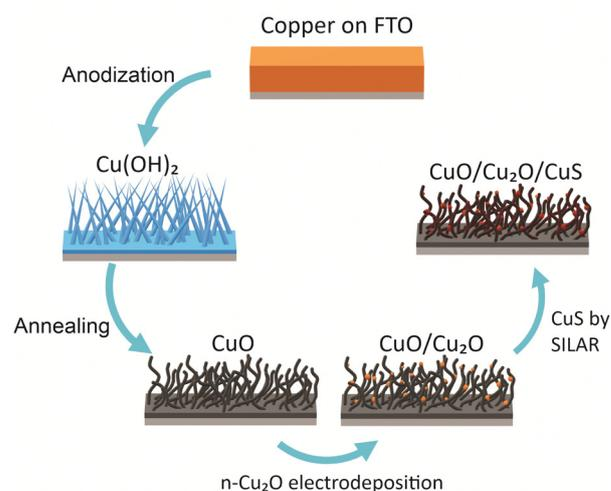
**Scheme 1** Summary of the experimental procedure to produce nanostructured films of CuO/Cu<sub>2</sub>O/CuS.
