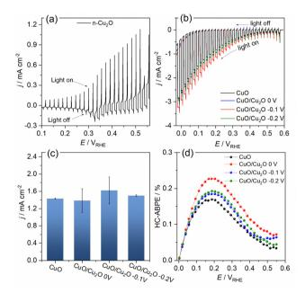
Fig. 4 Linear sweep voltammograms at 5 mV s<sup>-1</sup> under 1.5G pulsed illumination (100 mW cm<sup>-2</sup>) of (a) Cu<sub>2</sub>O and (b) CuO, CuO/Cu<sub>2</sub>O 0 V, CuO/Cu<sub>2</sub>O -0.1 V and CuO/Cu<sub>2</sub>O -0.2 V in 0.5 mol L<sup>-1</sup> Na<sub>2</sub>SO<sub>4</sub> solution (pH 6). (c) Mean and standard deviation of the photocurrent density values obtained at 0.1 V<sub>RHE</sub>. (d) HC-ABPE efficiency for CuO and CuO/Cu<sub>2</sub>O films.
