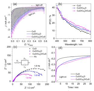
Fig. 5 (a) Linear sweep voltammograms at 5 mV s<sup>-1</sup>, (b) IPCE efficiency at 0.2 V<sub>RHE</sub> and (c) Nyquist plots at 0.2 V<sub>RHE</sub> for CuO, CuO/Cu<sub>2</sub>O -0.1 V and CuO/Cu<sub>2</sub>O/CuS films. (d) Stability test (photocurrent transient) at 0.35 V<sub>ERH</sub> for CuO and CuO/Cu<sub>2</sub>O/CuS films. Experiments carried out in 0.5 mol L<sup>-1</sup> Na<sub>2</sub>SO<sub>4</sub> solution (pH 6) under 1.5G (100 mW cm<sup>-2</sup>) illumination.
