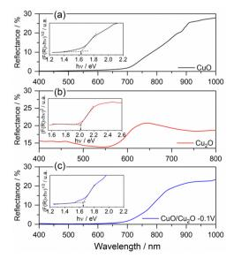
Fig. 3 Diffuse reflectance spectrum and Tauc plot of (a) CuO, (b) Cu $_2$ O and (c) CuO/Cu $_2$ O -0.1 V films.
