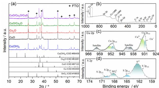
Fig. 2 (a) XRD patterns of  $\text{Cu}(\text{OH})_2$ ,  $\text{CuO}$ ,  $\text{Cu}_2\text{O}$ ,  $\text{CuO}/\text{Cu}_2\text{O}$ , and  $\text{CuO}/\text{Cu}_2\text{O}/\text{CuS}$  samples. XPS spectra of  $\text{CuO}/\text{Cu}_2\text{O}/\text{CuS}$  sample: (b) survey, (c) high resolution  $\text{Cu } 2p$  and (d) high resolution  $\text{S } 2p$ .
