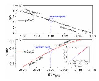
Fig. 6 Linear voltammogram under pulsed illumination (5 mV  $\rm s^{-1}$  and pulse frequency 1 Hz) in the conductivity transition region for (a) p-CuO and (b) n-Cu<sub>2</sub>O in 0.5 mol L<sup>-1</sup> Na<sub>2</sub>SO<sub>4</sub> solution (pH 6).
