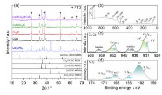
Fig. 2 (a) XRD pattens of Cu(OH)<sub>2</sub>, CuO, Cu<sub>2</sub>O, CuO/Cu<sub>2</sub>O, and CuO/ Cu<sub>2</sub>O/CuS samples. XPS spectra of CuO/Cu<sub>2</sub>O/CuS sample: (b) survey, (c) high resolution Cu 2p and (d) high resolution S 2p.
