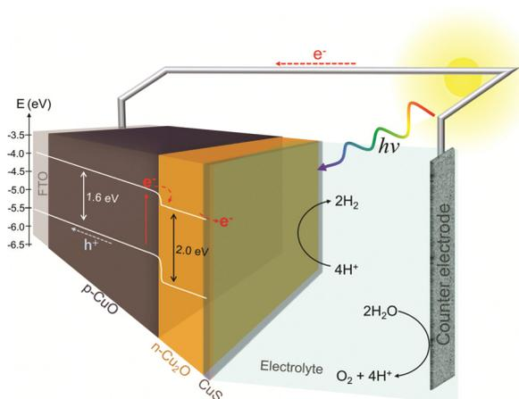
Fig. 7 Schematic band diagram of FTO/CuO/Cu<sub>2</sub>O/CuS for the PEC water splitting.
