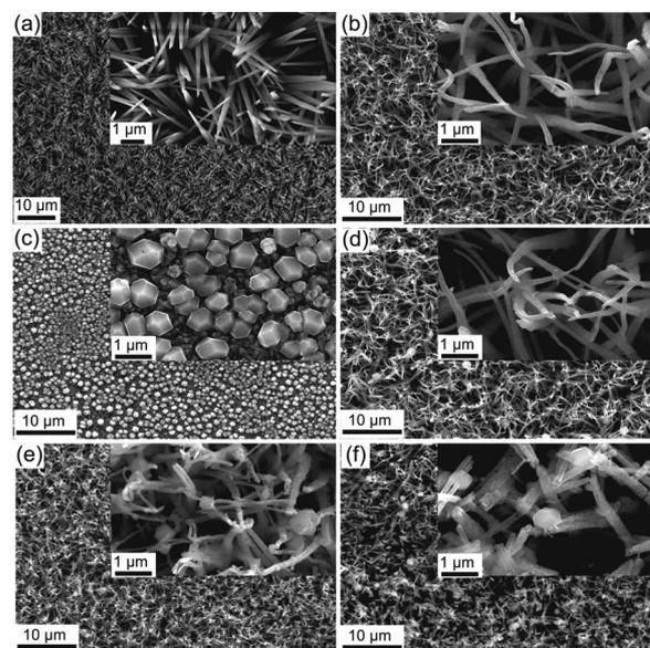
Fig. 1 SEM surface images of (a) Cu(OH)<sub>2</sub> nanoneedles, (b) CuO nanowires, (c) Cu<sub>2</sub>O polyhedral particles, (d) CuO/Cu<sub>2</sub>O 0 V, (e) CuO/Cu<sub>2</sub>O -0.1 V and (f) CuO/Cu<sub>2</sub>O -0.2 V.
