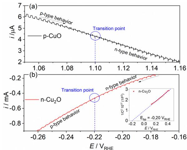
Fig. 6 Linear voltammogram under pulsed illumination ( $5 \text{ mV s}^{-1}$  and pulse frequency 1 Hz) in the conductivity transition region for (a) p-CuO and (b) n-Cu<sub>2</sub>O in  $0.5 \text{ mol L}^{-1} \text{ Na}_2\text{SO}_4$  solution (pH 6).
