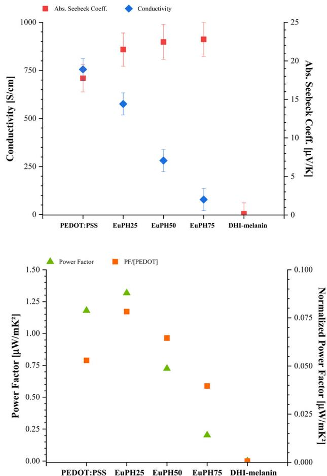
Fig. 3 Top panel: Seebeck coefficient (left axis) and conductivity (right axis). Bottom panel: power factor (left axis) and power factor normalized to the PEDOT content (right axis).
