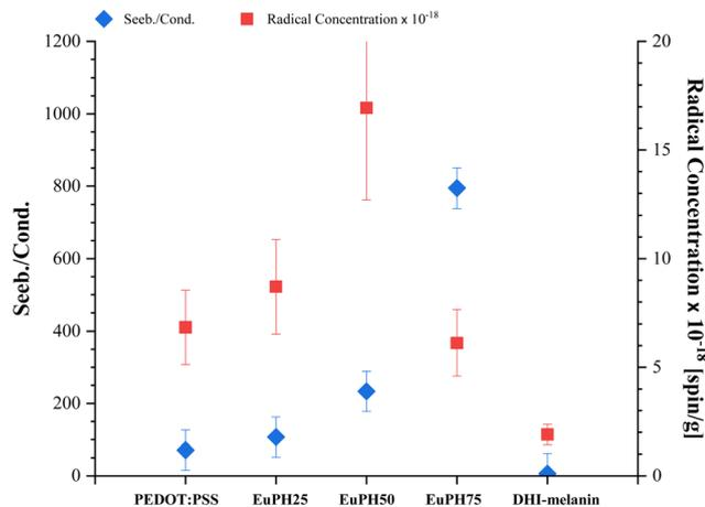
Fig. 8 Seebeck over conductivity ratio (left axis) and radical concentration (right axis).
