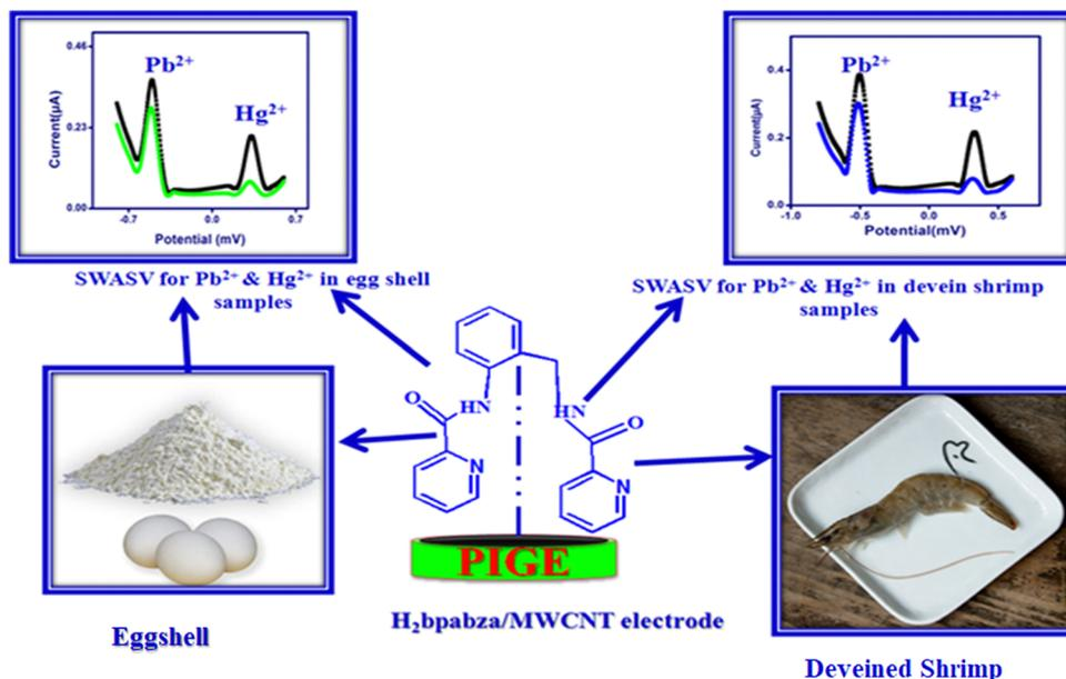
Scheme 2 Mechanism of the  $H_2bpabza/MWCNT$  electrode for detection of  $Pb^{2+}$  and  $Hg^{2+}$ .
