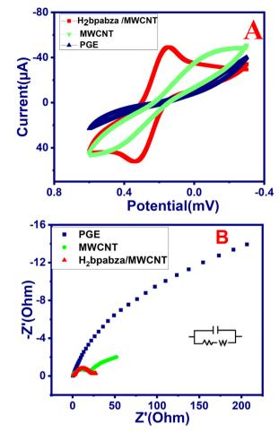
Fig. 5 Electrochemical characterization for  $H_2$ bpabza/MWCNT: (A) cyclic voltammetry (CV) and (B) EIS for  ${\rm Fe(CN)_6}^{2-/3-}$  containing 0.1 M acetate buffer, scan rate: 50 mV s $^{-1}$ .
