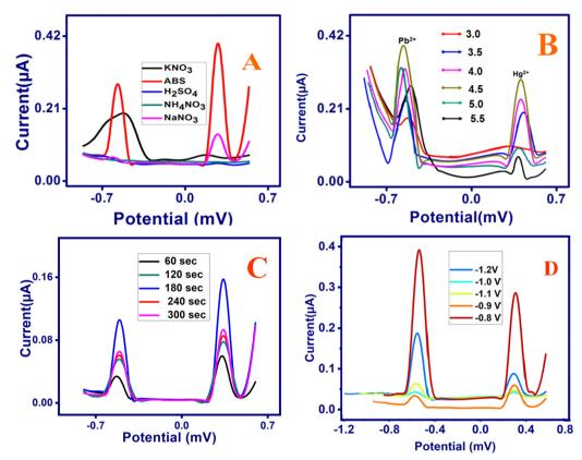
Fig. 7 Optimization of experimental conditions. Influence of (A) supporting electrolytes, (B) pH, (C) deposition time, and (D) deposition potential on the voltammetric response of the  $H_2$ bpabza/MWCNT-modified electrode for 50  $\mu$ g  $L^{-1}$  of  $Pb^{2+}$  and  $Hg^{2+}$ , deposition potential: -0.8 V, frequency 25 Hz; amplitude, 25 mV; increment potential 4 mV.
