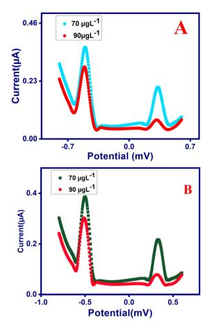
Fig. 11 Stripping analysis of Pb<sup>2+</sup> and Hg<sup>2+</sup> (70 and 90  $\mu$ g L<sup>-1</sup>, respectively) in (A) deveined shrimp and (B) eggshell samples on the H<sub>2</sub>bpabza/ MWCNT electrode in 0.1 M acetate buffer. Scan rate: 50 mV s<sup>-1</sup>
