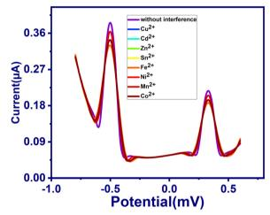
Fig. 10 SWASV of  $H_2$ bpabza/MWCNT in 0.1 M acetate buffer containing 90  $\mu$ g  $L^{-1}$  Pb<sup>2+</sup> and  $Hg^{2+}$  with the addition of 50  $\mu$ g  $L^{-1}$  Cu<sup>2+</sup>, Cd<sup>2+</sup>, Zn<sup>2+</sup>, Sn<sup>2+</sup>, Fe<sup>2+</sup>, Ni<sup>2+</sup>, Mn<sup>2+</sup>, and Co<sup>2+</sup> at a scan rate of 50 mV s<sup>-1</sup>.
