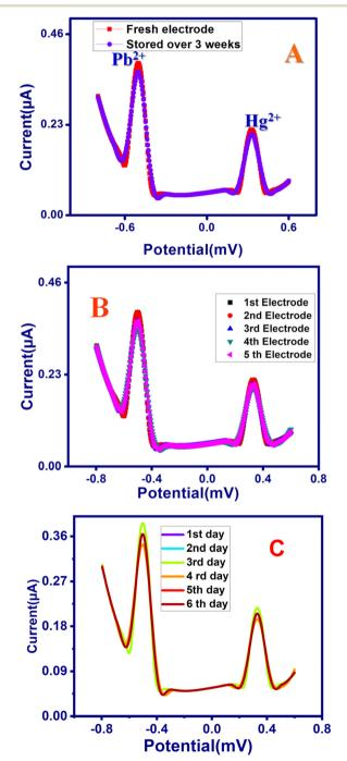
Fig. 9 SWASV for  $H_2$ bpabza/MWCNT: (A) stability of fresh electrodes and electrodes stored for 3 weeks and (B) reproducibility for different electrodes. (C) Reusability in 0.1 M acetate buffer for 90  $\mu$ g L $^{-1}$  Pb $^{2+}$  and  $Hg^{2+}$  at a scan rate of 50 mV s $^{-1}$ .
