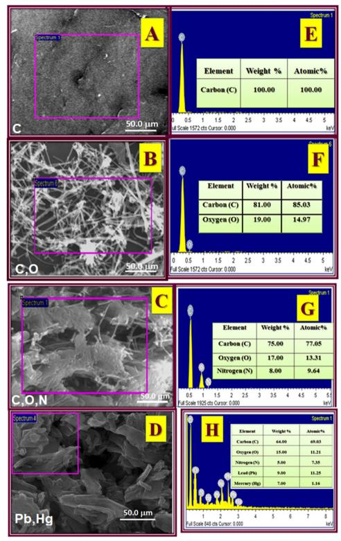
Fig. 4 SEM with EDAX images of (A) and (E) PGE, (B) and (F) MWCNT, (C) and (G) H<sub>2</sub>bpabza/MWCNT, and (D) and (H) [Pb<sup>2+</sup> and Hg<sup>2+</sup>-H<sub>2</sub>bpabza]/ MWCNT electrodes.
