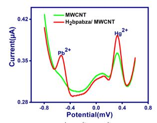
Fig. 6 SWASV for 90  $\mu g$  L<sup>-1</sup> of Pb<sup>2+</sup> and Hg<sup>2+</sup> on the MWCNT and H<sub>2</sub>bpabza/MWCNT-modified electrodes in 0.1 M acetate buffer, pH 4.5. Scan rate: 50 mV s<sup>-1</sup>
