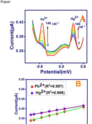
Fig. 8 (A) SWASV responses and (B) the corresponding calibration plot of the  $H_2$ bpabza/MWCNT electrode in the detection of  $Pb^{2+}$  and  $Hg^{2+}$  over a concentration range of 2, 10.3, 30, 50.3, 70.3, 90.4, and 140  $\mu g \, L^{-1}$  for  $Pb^{2+}$  and  $Hg^{2+}$  by deposition for 180 s in 0.1 M acetate buffer (pH 4.5). Deposition potential: -0.8 V; frequency 25 Hz; amplitude 25 mV; increment potential 4 mV.
