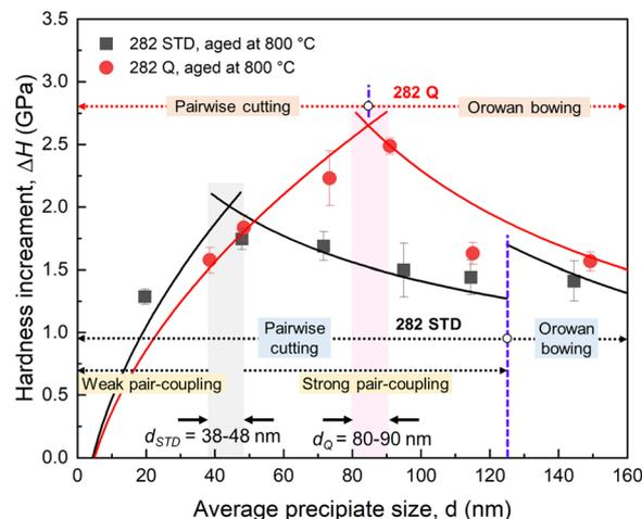
Fig. 14 Relationship between hardness increment ( $\Delta H$ ) as a function of average precipitate size ( $d$ ) for alloys STD and Q exposed to 800 °C for various durations. Experimental data points are derived from hardness measurements, while the solid lines represent the theoretical calculations.
