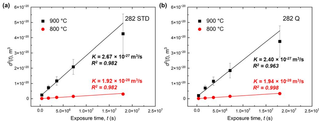
Fig. 13 Plots of average precipitate size, ( $d^3(t)$ ), versus exposure time ( $t$ ) for alloy STD (a) and alloy Q (b) for temperatures of 800 °C and 900 °C. The coarsening rate constants are determined from the best linear fit of the experimental data.
