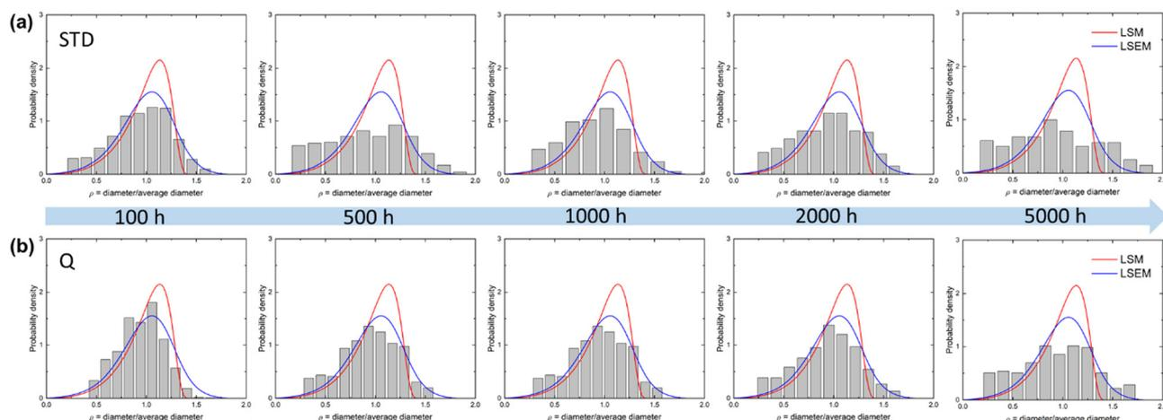
**Fig. 6** The evolution of scaled PSDs for  $\gamma'$  precipitates after exposure to 900 °C for different durations, compared with the prediction of the LSW model (red line) and the LSEM model (precipitate volume fraction = 20%, blue line) (a) alloy STD and (b) alloy Q.
