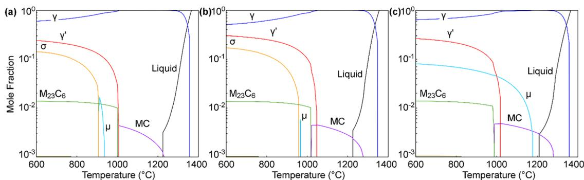
Fig. 1 Thermo-Calc phase prediction for mole fraction between 0.001 and 1 and temperature between 600 °C and 1400 °C for alloys (a) STD, (b) P, and (c) Q.
