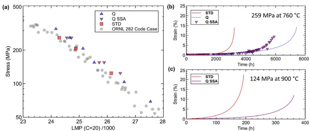
Fig. 10 (a) Larson–Miller parameter plot for alloys STD, Q and the H282 code case.<sup>32</sup> (b) and (c) Creep curves for creep testing at 760 °C and 259 MPa and 900 °C and 124 MPa, respectively.
