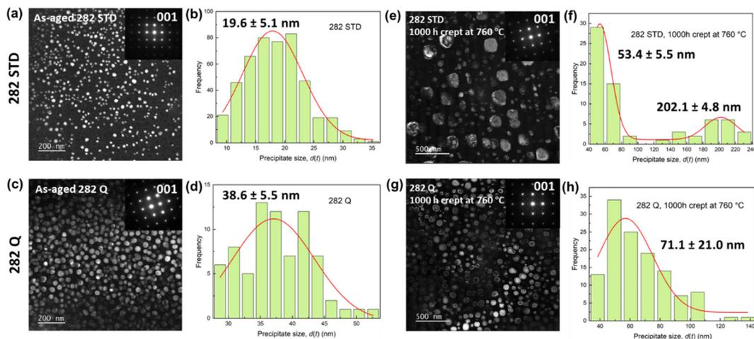
Fig. 4 TEM DF images and  $\gamma'$  precipitate size distributions of the alloys STD (a)–(d) and Q (e)–(h) in their as aged conditions and their 1000 h crept at 259 MPa and 760 °C conditions, respectively.
