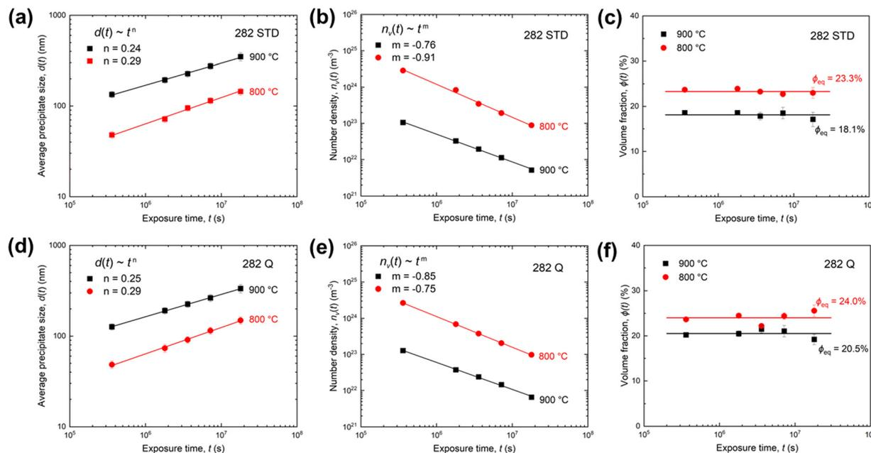
Fig. 7 The temporal evolution of (a) average size ( $d(t)$ ), (b) number density ( $n_v(t)$ ), and (c) volume fraction ( $\phi(t)$ ) of  $\gamma'$  precipitates in alloys STD and Q exposed to 800 °C and 900 °C. Solid lines in the above figures represent the linear fits and average values of the experimental data, respectively.
