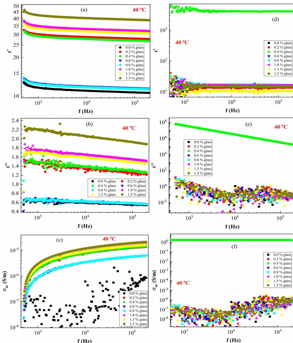
Fig. 7 Dielectric constants ( $\epsilon'$  and  $\epsilon''$ ) and conductivity ( $\sigma_{AC}$ ) of PEVA/conductive glass powder composite membranes with the composition (60%  $B_2O_3$  – 10% CdO – 15%  $Na_2O$  – 15% NaF doped with 5% CuO) as functions of frequency at a constant temperature (40 °C) (a)–(c) before radiation, and (d)–(f) after radiation.
