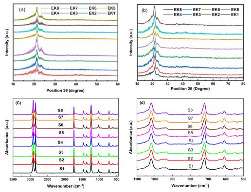
Fig. 1 XRD patterns of the PEVA composites (a) before and (b) after irradiation. (c) FT-IR spectra and (d) magnified IR spectra at lower wavenumbers (500-1100 cm<sup>-1</sup>) of PEVA mixed with different amounts of conductive ground glass particles (0, 0.2, 0.4, 0.6, 0.8, 1, 1.3 and 1.5 wt%)
