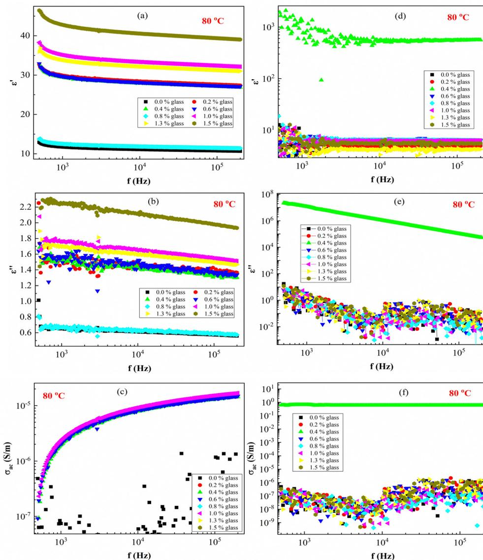
Fig. 8 Dielectric constants ( $\epsilon'$  and  $\epsilon''$ ) and conductivity ( $\sigma_{AC}$ ) of composite membranes of PEVA/glass powder composition (60%  $B_2O_3$  – 10% CdO – 15%  $Na_2O$  – 15% NaF doped with 5% CuO) as functions of frequency at a constant temperature of 80 °C: (a)–(c) before radiation and (d)–(f) after radiation.
