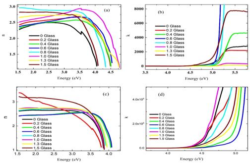
Fig. 6 Refractive indices of the PEVA/glass powder composite membranes with the composition (60% B2O3 – 10% CdO – 15% Na2O – 15% NaF doped with 5% CuO): (a) refractive index and (b) extinction coefficient before irradiation; (c) refractive index and (d) extinction coefficient after irradiation.
