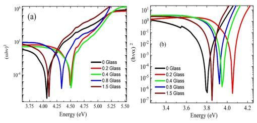
Fig. 5 Optical bandgap energies of the prepared PEVA/glass powder composite membranes with the composition 60% B<sub>2</sub>O<sub>3</sub>  $\pm$  10% CdO + 15% Na<sub>2</sub>O + 15% NaF doped with 5% CuO: (a) before irradiation and (b) after irradiation.
