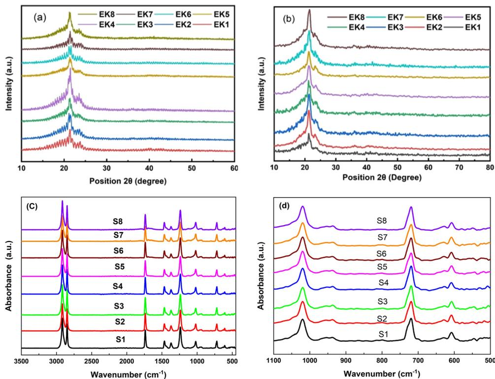
Fig. 1 XRD patterns of the PEVA composites (a) before and (b) after irradiation. (c) FT-IR spectra and (d) magnified IR spectra at lower wavenumbers (500–1100  $\text{cm}^{-1}$ ) of PEVA mixed with different amounts of conductive ground glass particles (0, 0.2, 0.4, 0.6, 0.8, 1, 1.3 and 1.5 wt%).
