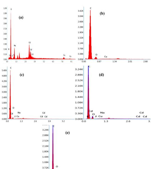
Fig. 3 EDX analysis of selected PEVA composite membranes containing different amounts of conductive ground glass powder particles (0, 0.2, 0.4, 0.6, 0.8, 1, 1.3 and 1.5 wt%): (a) EKO, (b) EK1, (c) EK3, (d) EK6, and (e) EK8
