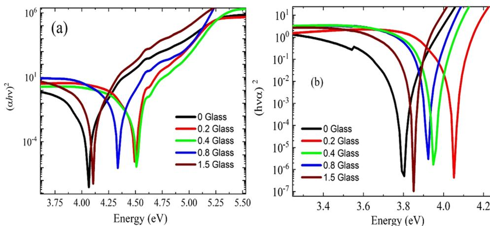
Fig. 5 Optical bandgap energies of the prepared PEVA/glass powder composite membranes with the composition 60%  $B_2O_3$  + 10% CdO + 15%  $Na_2O$  + 15% NaF doped with 5% CuO: (a) before irradiation and (b) after irradiation.
