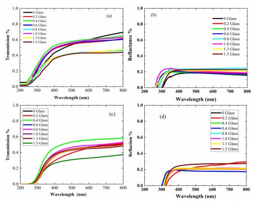
Fig. 4 Optical properties of glass-powder-incorporated PEVA composite membranes with the composition  $60\% B_2O_3 + 10\% CdO + 15\% Na_2O + 15\% NaF doped with 5% CuO: (a) transmission and (b) reflection before irradiation; (c) transmission and (d) reflection after irradiation.$
