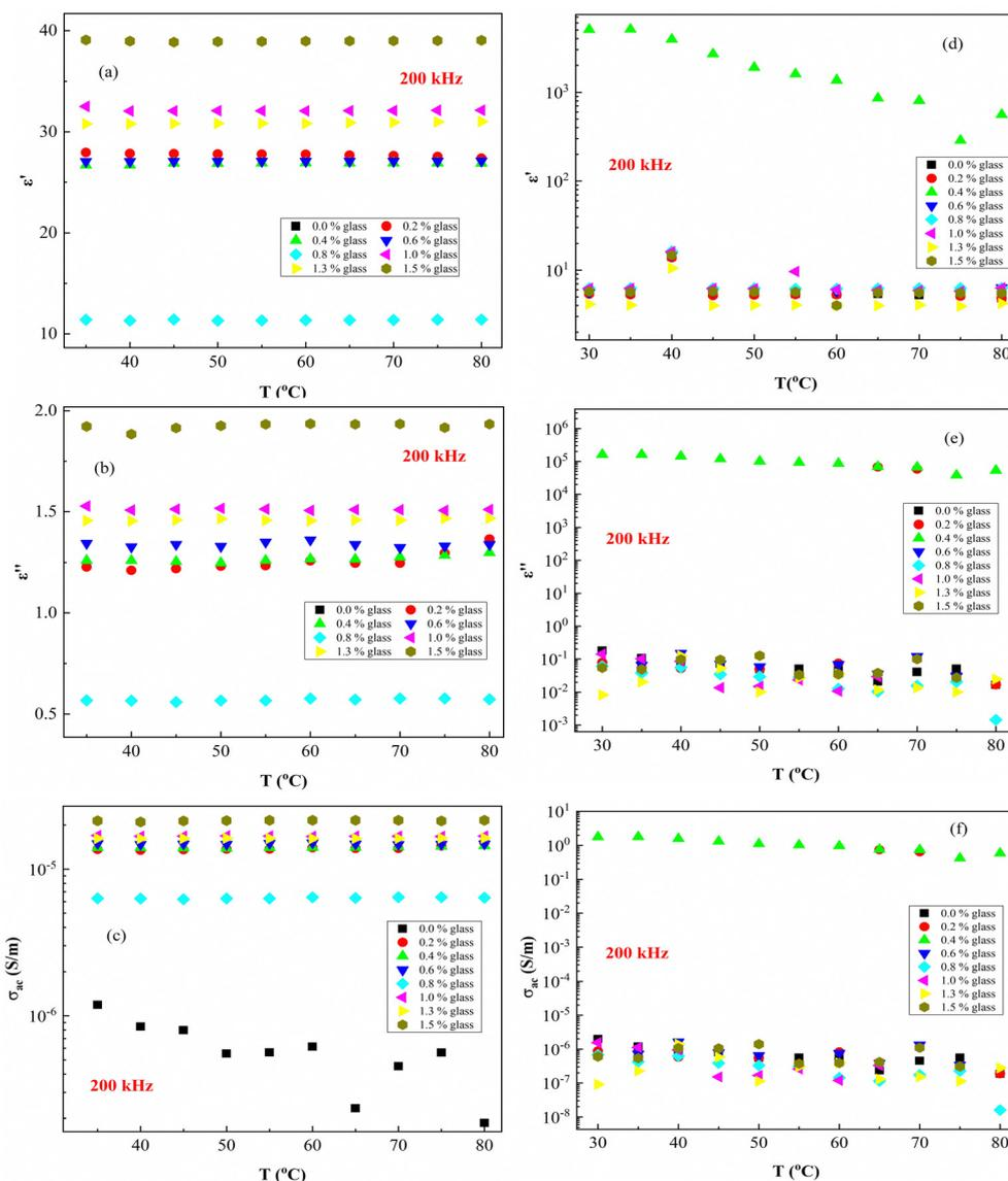
Fig. 9 Dielectric constants ( $\epsilon'$  and  $\epsilon''$ ) and conductivity ( $\sigma_{AC}$ ) of composite membranes with PEVA/conductive glass powder composition (60%  $B_2O_3$  – 10% CdO – 15%  $Na_2O$  – 15% NaF doped with 5% CuO) as functions of temperature at a fixed frequency of 200 kHz before irradiation (a), (b), and (c) and after irradiation (d), (e), and (f).
