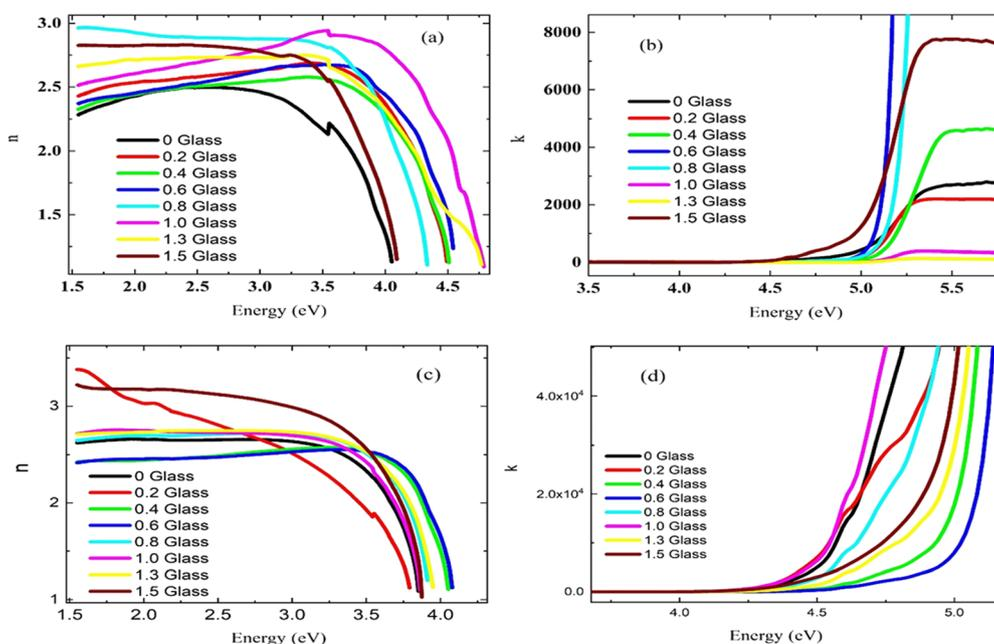
**Fig. 6** Refractive indices of the PEVA/glass powder composite membranes with the composition (60%  $B_2O_3$  – 10%  $CdO$  – 15%  $Na_2O$  – 15%  $NaF$  doped with 5%  $CuO$ ): (a) refractive index and (b) extinction coefficient before irradiation; (c) refractive index and (d) extinction coefficient after irradiation.
