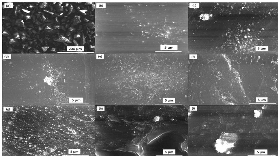
Fig. 2 FE-SEM images of PEVA samples mixed with different amounts of conductive ground glass powder particles (0, 0.2, 0.4, 0.6, 0.8, 1, 1.3 and 1.5 wt%): (a) glass only, (b) EK1, (c) EK2, (d) EK3, (e) EK4, (f) EK5, (g) EK6, (h) EK7, and (i) EK8.
