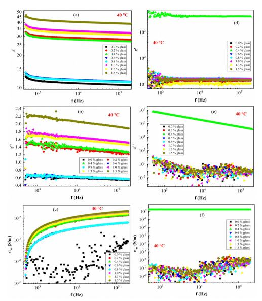
Fig. 7 Dielectric constants ( $\epsilon'$  and  $\epsilon''$ ) and conductivity ( $\sigma_{AC}$ ) of PEVA/conductive glass powder composite membranes with the composition (60%  $B_2O_3 - 10\%$  CdO - 15% Na<sub>2</sub>O - 15% NaF doped with 5% CuO) as functions of frequency at a constant temperature (40 °C) (a)–(c) before radiation, and (d)–(f) after radiation.
