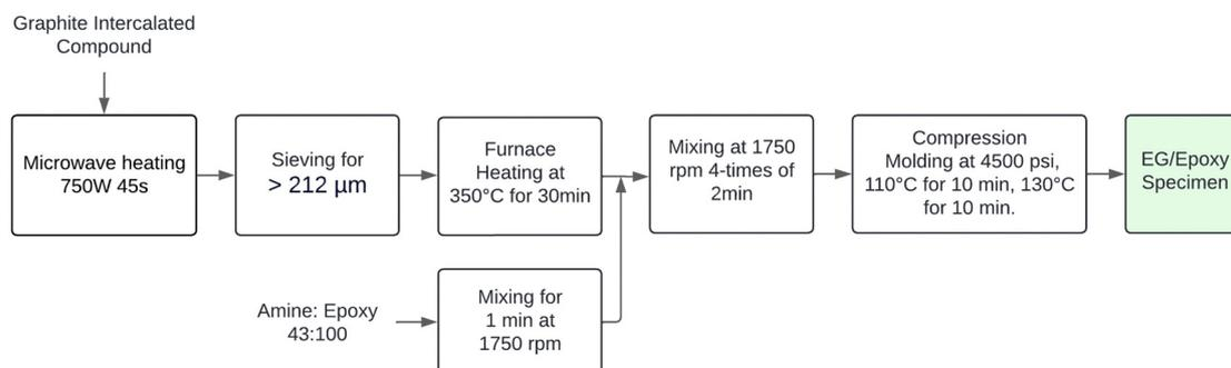
Fig. 2 Preparation procedure scheme for composite specimens.
