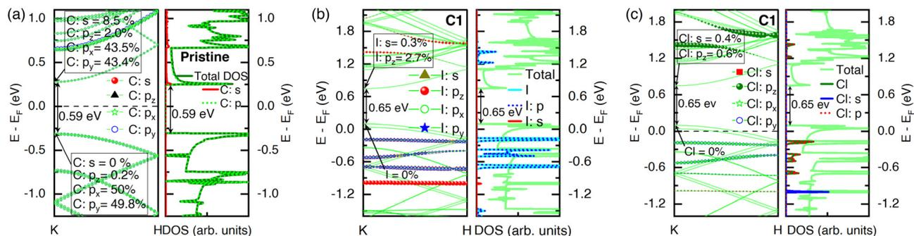
**Fig. 3** The orbital projected band structure and density of states (DOS) of (a) a pristine (8,0) SWCNT bundle. Each sub-orbital contribution on the band structure and DOS for (b) iodine and (c) chlorine atoms of ICl molecules when they were doped in a vertical orientation inside the tube with very close spacing (C1).
