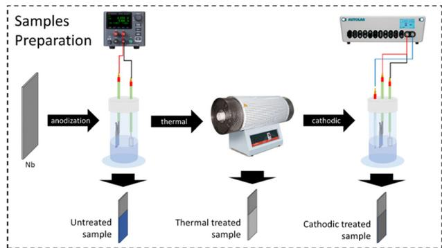
Fig. 1 Scheme of the procedure used to obtain the different samples.
