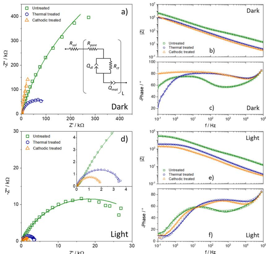
Fig. 5 (a) Nyquist, (b) Bode  $|Z|$  and (c) Bode Phase plots for samples in the dark, and (d) Nyquist, (e) Bode  $|Z|$  and (f) Bode phase plots for samples with illumination. The Bode phase is normalized to  $R_{sol} = 0$ .
