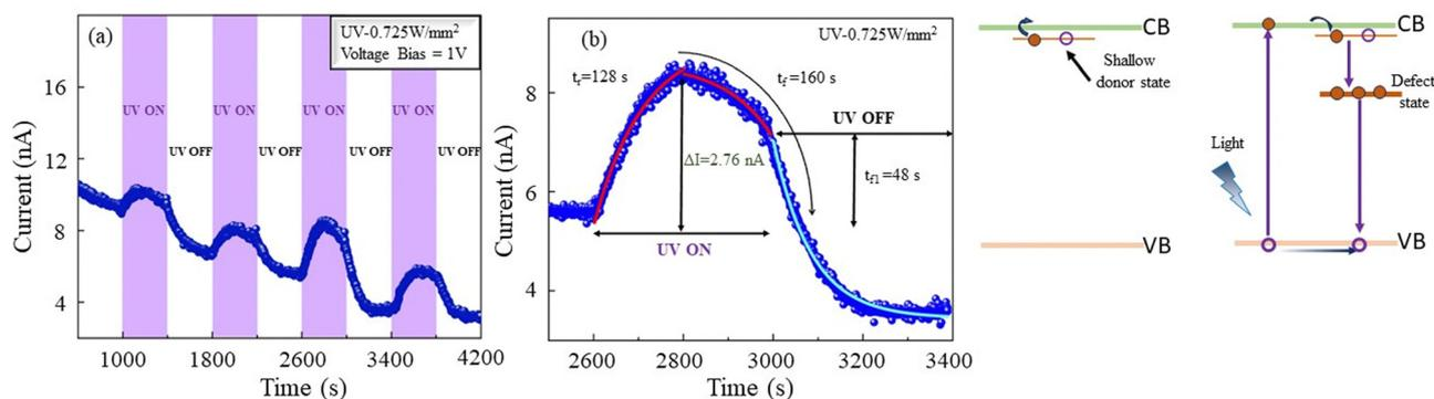
**Fig. 4** The effect of UV light on the Al/indigo/Al device. (a) Five cycles of UV on/off measurements with a UV light intensity of  $0.725 \text{ W mm}^{-2}$ . (b) One random cycle of UV on–off measurements with a UV light intensity of  $0.725 \text{ W mm}^{-2}$  for detailed analysis of NPC followed by PPC. (c) A schematic diagram of the effect of defect states on capturing the electrons excited due to the exposure to light.
