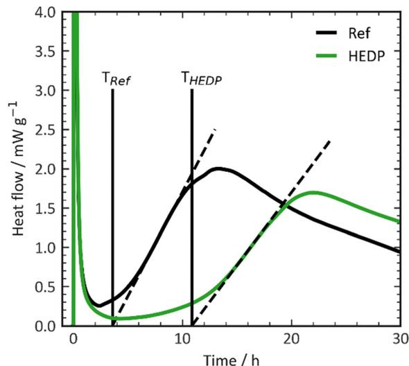
Fig. 1 Heat flow curves from calorimetry without and with 5 mmol L<sup>-1</sup> HEDP displaying dormant period and slope of the silicate reaction.
