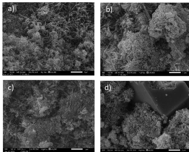
Fig. 9 Morphologies of the hydrated cement pastes at maximum heat flow of the C<sub>3</sub>S reaction. (a) EDTMP, (b) HEDP, (c) reference (d) AMPA.
