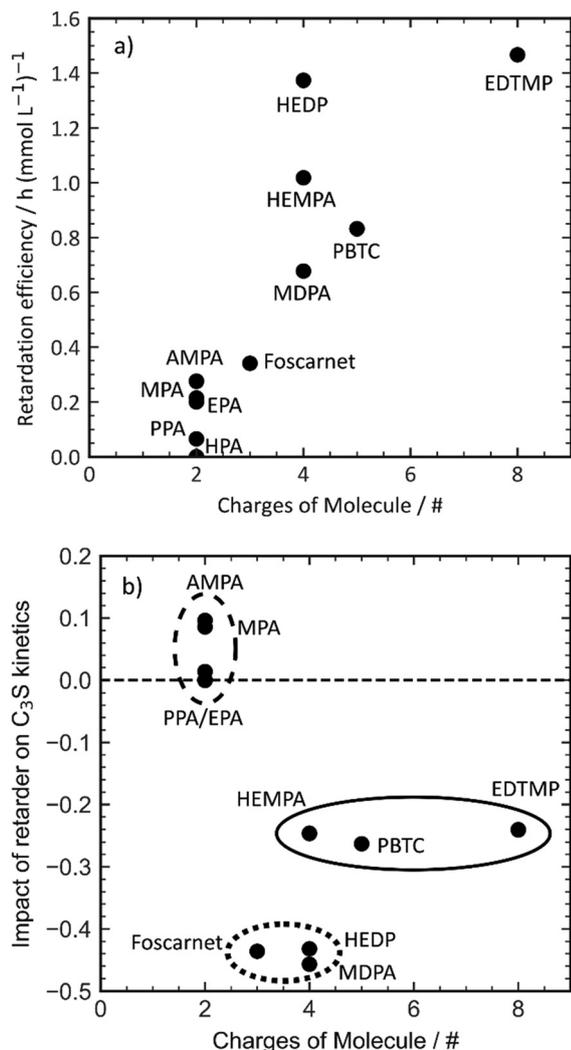
Fig. 3 Impact of charges of retarders on the (a) retardation efficiency and (b) C<sub>3</sub>S kinetics.
