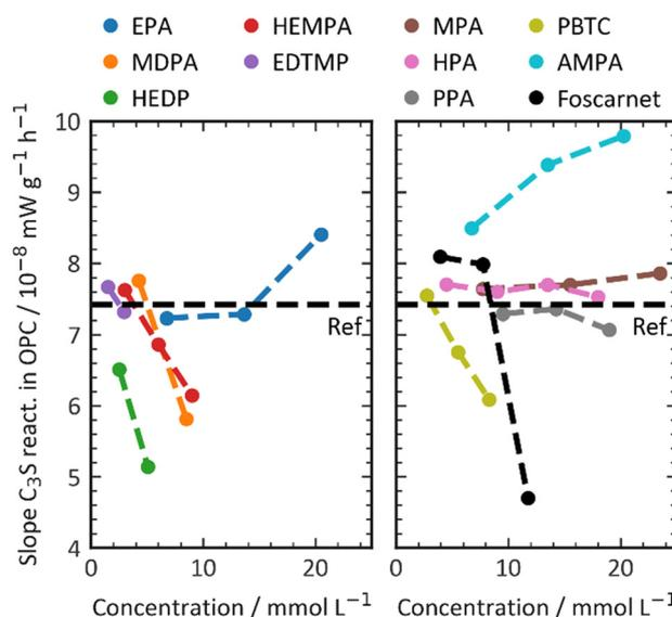
Fig. 5 Impact of the retarder on the C<sub>3</sub>S kinetics at the accelerating period of the silicate reaction.
