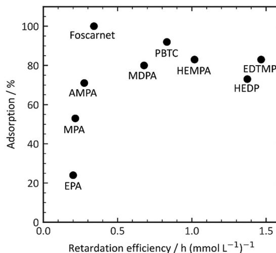
Fig. 4 Correlation of retarder adsorption and efficiency.
