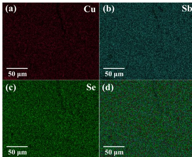
Fig. 4 The uniform distribution of (a) Cu (copper), (b) Sb (antimony), and (c) Se (selenium) and (d) overall distribution of Cu, Sb and Se elements throughout the area in the as-grown  $\text{CuSbSe}_2$  single crystal.
