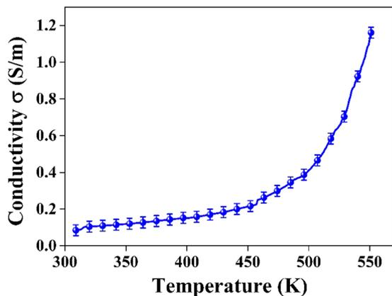
Fig. 11 Electrical conductivity ' $\sigma$ ' variation with temperature ' $T$ ' for the CuSbSe<sub>2</sub> single crystal.
