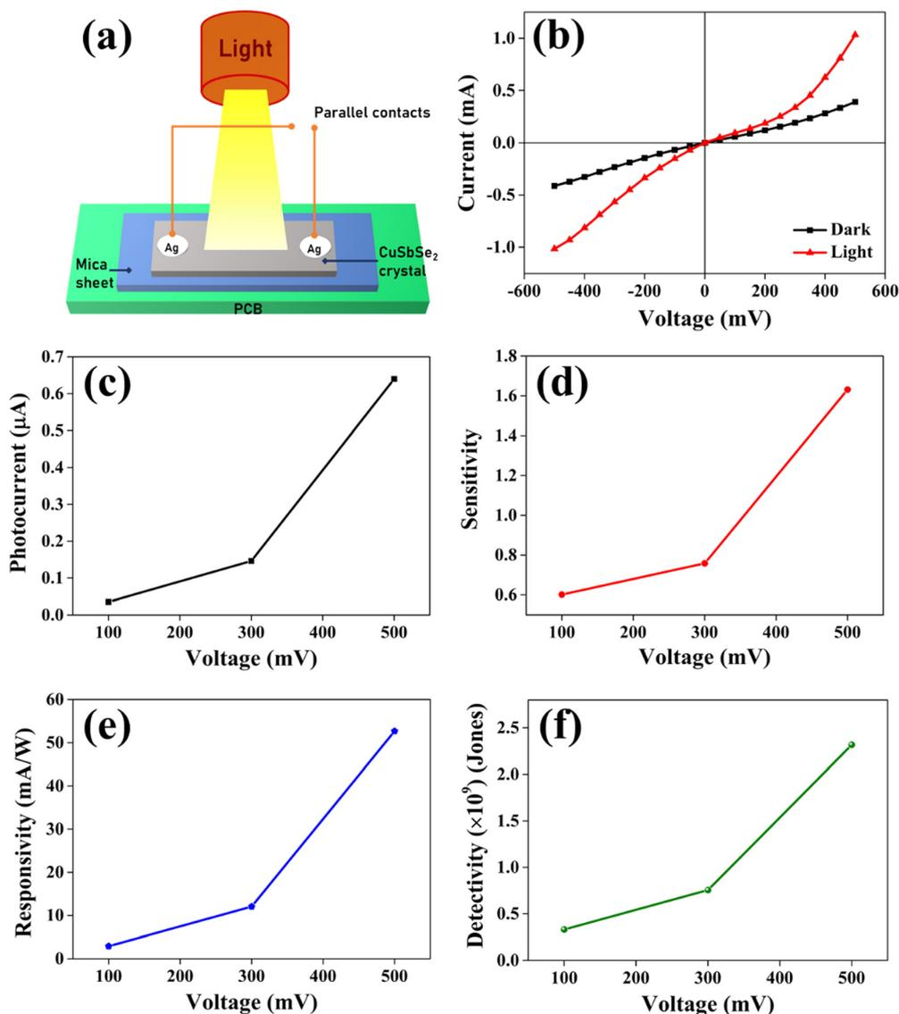
Fig. 17 (a) Schematic view of a CuSbSe<sub>2</sub> single crystal based photodetector. (b) *I*–*V* characteristics of a photodetector under dark and illuminated conditions for the parallel to planar configuration and the variation of (c) photocurrent, (d) sensitivity, (e) responsivity and (f) detectivity as a function of voltage at a light intensity of 50 mW cm<sup>-2</sup>.
