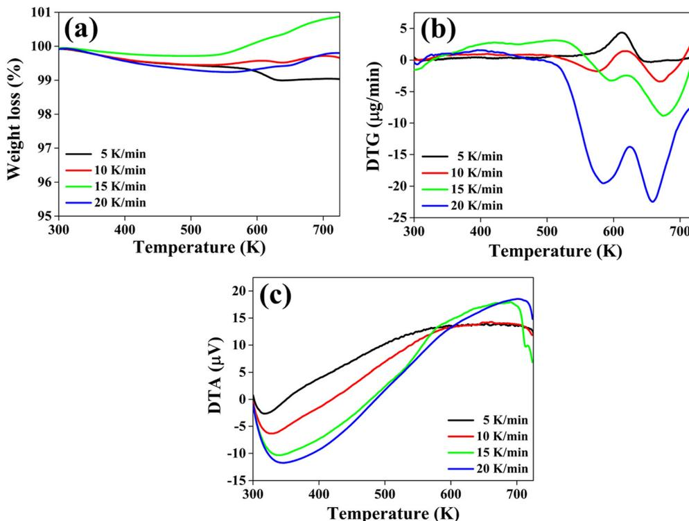
Fig. 14 (a) The TG, (b) DTG, and (c) DTA curves of the grown CuSbSe<sub>2</sub> single crystal.
