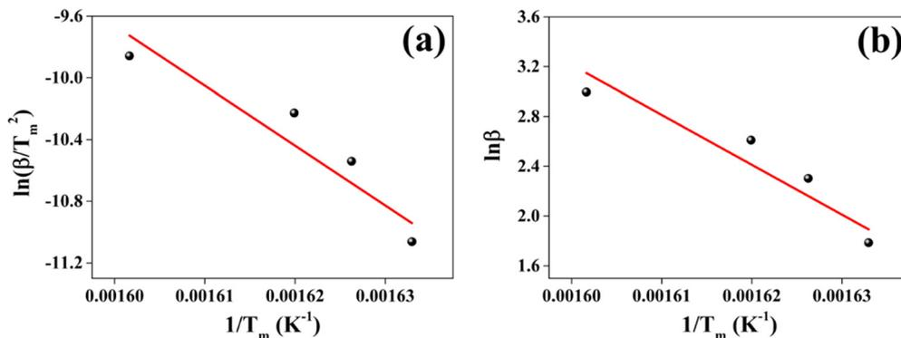
Fig. 15 (a) The Kissinger plot and (b) FWO plot of the grown  $\text{CuSbSe}_2$  single crystal.
