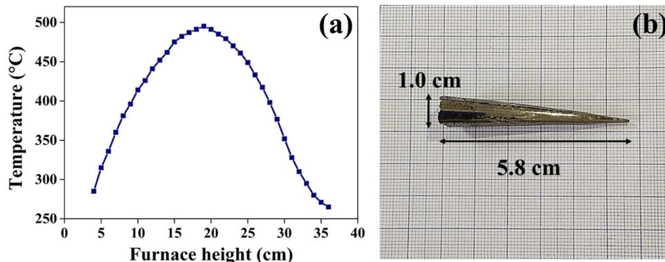
Fig. 1 (a) Axial temperature profile of the growth furnace and (b) the grown  $\text{CuSbSe}_2$  ingot crystal.
