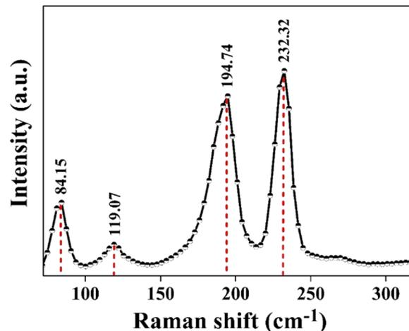
Fig. 7 The Raman spectrum of the grown CuSbSe<sub>2</sub> single crystal.
