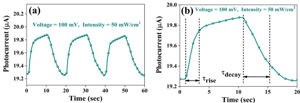
Fig. 18 (a) Pulse photoresponse at a 100 mV bias voltage and (b) magnified image of a single pulse for a 100 mV bias voltage of the CuSbSe<sub>2</sub> photodetector.
