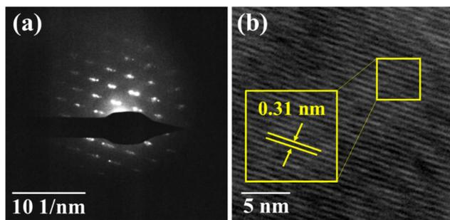
Fig. 6 (a) SAED pattern and (b) fringe pattern of the as-grown CuSbSe<sub>2</sub> single crystal.
