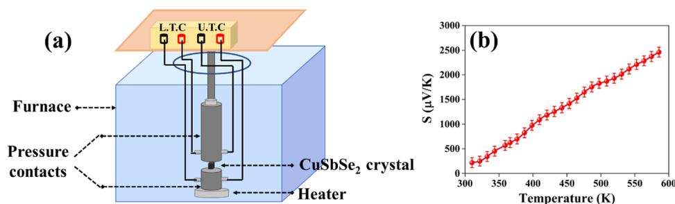
Fig. 10 (a) Schematic representation of the measurement setup to measure the Seebeck coefficient and (b) temperature dependent Seebeck coefficient of the as-grown CuSbSe<sub>2</sub> single crystal.
