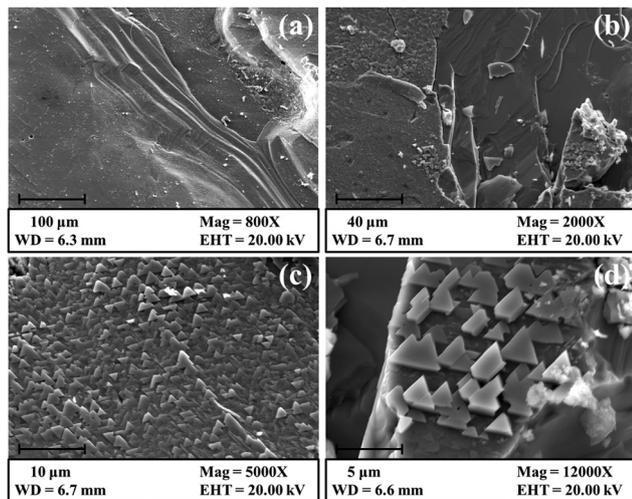
Fig. 5 FESEM photographs of the as-grown CuSbSe<sub>2</sub> single crystal taken at different magnifications.
