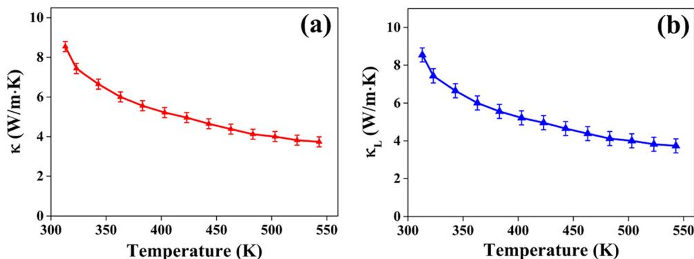
Fig. 13 The variation of (a) total thermal conductivity ' $\kappa_{\text{total}}$ ' and (b) lattice thermal conductivity ' $\kappa_L$ ' with temperature  $T$  for the  $\text{CuSbSe}_2$  single crystal.
