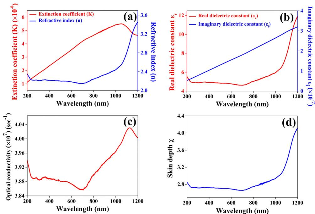
Fig. 9 Plots of (a) extinction coefficient and refractive index, (b) real and imaginary dielectric constants, (c) optical conductivity and (d) skin depth as a function of wavelength for the  $\text{CuSbSe}_2$  single crystal.
