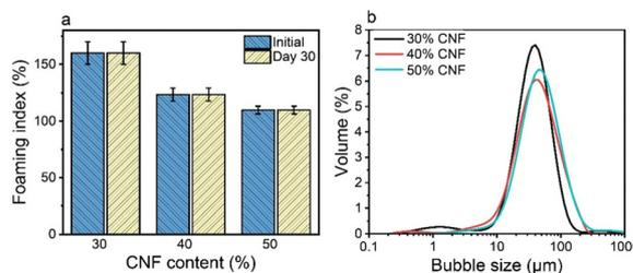
**Fig. 3** Foamability and foam stability of the foams stabilized by CTAB–LNPs (5 mg g<sup>-1</sup>) with the addition of CNFs (30 to 50 wt% relative to the total solid mass). (a) Foaming indices at the initial stage and on day 30. (b) Bubble size distribution of the foams, measured on day 3 after foaming.
