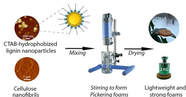
**Scheme 1** A general view of this work. The CTAB-hydrophobized LNPs for durable Pickering foam formation with the presence of CNFs, which were further dried for making lightweight and strong solid foams. Note that the schematic drawing of CTAB-coated LNPs is not drawn to scale.
