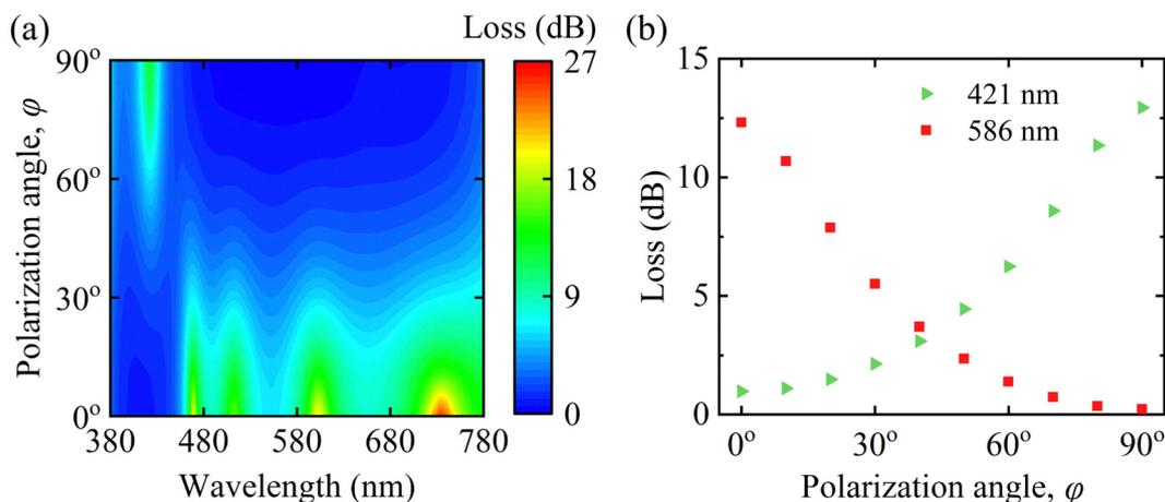
Fig. 10 (a) Loss profile due to change of  $\phi$  from 0° to 90° at operating wavelengths from 380 nm to 780 nm of our proposed dielectric grating metasurface. (b) Loss at the wavelengths of 421 and 586 nm for varying  $\phi$ . Here, we considered the resonance wavelengths at  $\phi$  values of 0° and 90°.
