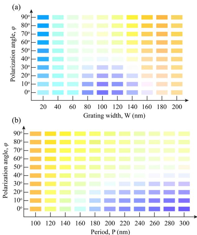
Fig. 7 (a) A color palette of our proposed structure for varying  $W$  and  $\phi$ . We adopted a range of  $W$  from 20 to 200 nm. Here, we rotated the  $\phi$  from  $0^\circ$  to  $90^\circ$ . (b) A color palette of our proposed dielectric metasurface structure for varying  $P$  and  $\phi$ . We adopted a range of  $P$  from 100 to 300 nm. Here, we rotated the  $\phi$  from  $0^\circ$  to  $90^\circ$ .
