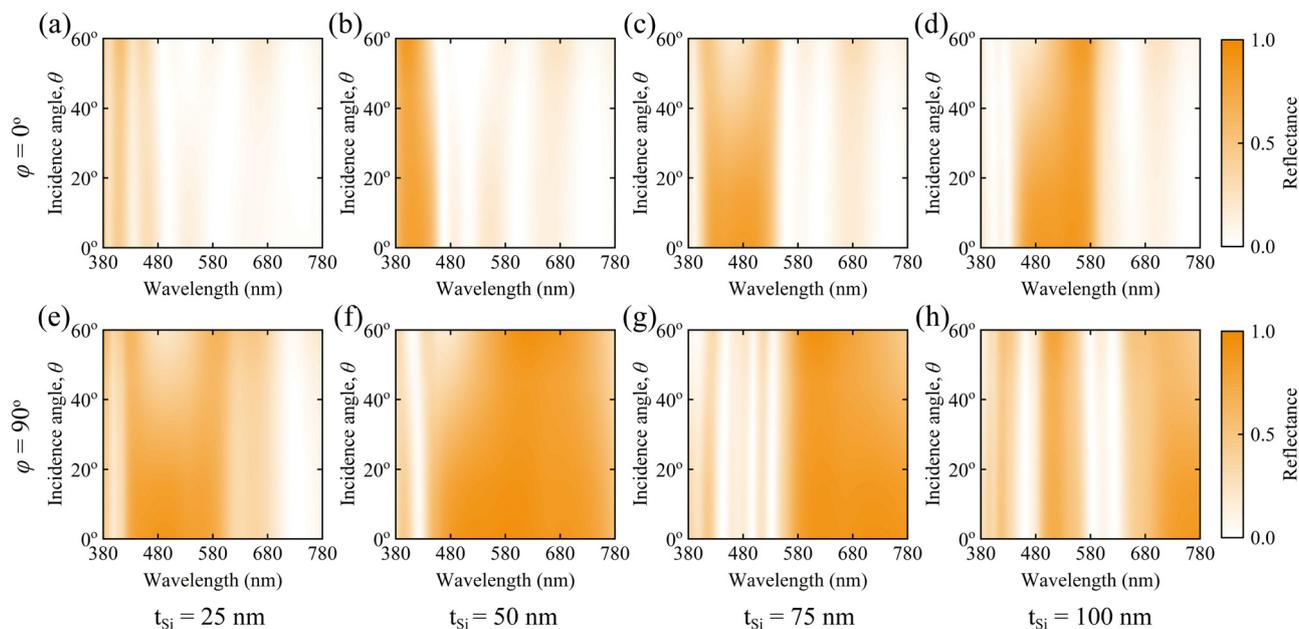
**Fig. 9** Reflectance spectra for different thicknesses of Si layer of our proposed grating dielectric metasurface with varying  $\theta$  values for the  $\varphi$  of (a)–(d)  $0^\circ$  and (e)–(h)  $90^\circ$ . In this case,  $t_{\text{Si}}$  increases from 25 to 100 nm, and the  $\theta$  increases from  $0^\circ$  to  $60^\circ$ .
