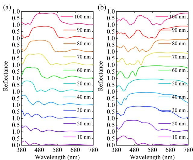
Fig. 4 Reflectance spectra of the dielectric metasurface structure for different  $t_{\text{Si}}$  values at (a)  $\varphi = 0^\circ$  and (b)  $\varphi = 90^\circ$ . Other structural parameters were kept constant.
