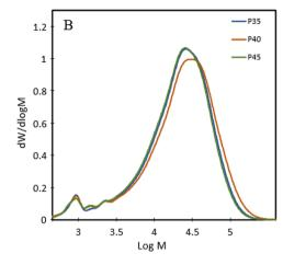
(A) FTIR spectra (spectra have been shifted vertically for clarity), and (B) GPC traces of TPUs.
