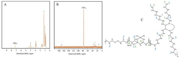
Fig. 2 (A) <sup>1</sup>H NMR spectra, (B) <sup>13</sup>C NMR spectra, and (C) NMR peak designations for P40
