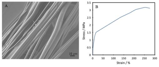
Fig. 12 (A) SEM image of spun P40 fibres, and (B) representative tensile stress-strain plot of spun P40 fibre yarns.
