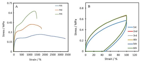
(A) Representative tensile stress-strain plots of TPUs, and (B) cyclic tensile plots of P40 with 1-minute rest between cycles.
