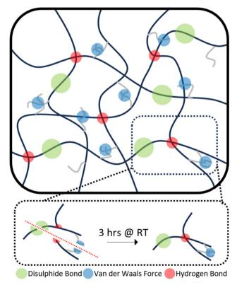
Scheme 2 Synergistic self-healing mechanism of TPUs.
