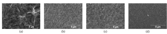
Fig. 2 SEM images of P(VDF-TrFE) (a) and composite films with various concentration of ZnO particles [10 (b), 20 (c), 30 wt% (d)].
