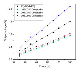
Fig. 4 Output voltage of 20  $\mu$ m-thick P(VDF-TrFE) and various ZnO composites at different forces.
