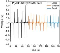
Fig. 7 Output voltage of sensing robot arm for P(VDF-TrFE) and 20% ZnO composite with small (blue), medium (orange), and large (black) tube.
