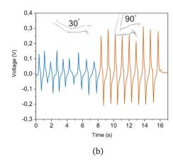
Fig. 10 Piezoelectric sensor fabricated by spray coating and attached to the elbow (a), and output voltage obtained from moving the elbow in two different approaches (b).
