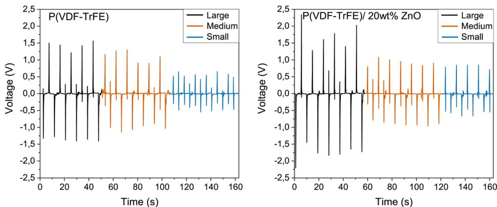
Fig. 7 Output voltage of sensing robot arm for P(VDF-TrFE) and 20% ZnO composite with small (blue), medium (orange), and large (black) tube.
