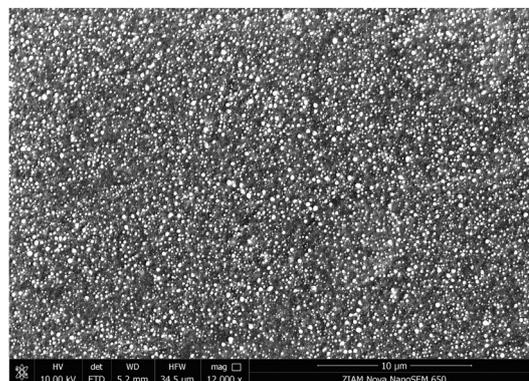
Fig. 9 SEM image of the spray coated 20% ZnO composite film.
