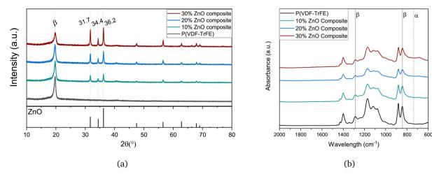
Fig. 1 XRD (a) and FTIR (b) graph of P(VDF-TrFE) and composite films with various concentration of ZnO particles (10, 20, 30 wt%).
