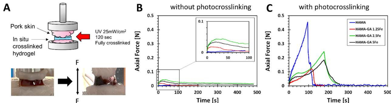
Fig. 11 Measurement of tissue adhesion force of hydrogel samples: HAMA30, HAMA-GA 1.25Fe, HAMA-GA 2.5Fe and HAMA-GA 5Fe ( $n = 4$ ). (A) The tack test setup using porcine muscles. (B) Hydrogel samples without photocrosslinking. (C) Hydrogel samples with photocrosslinking.
