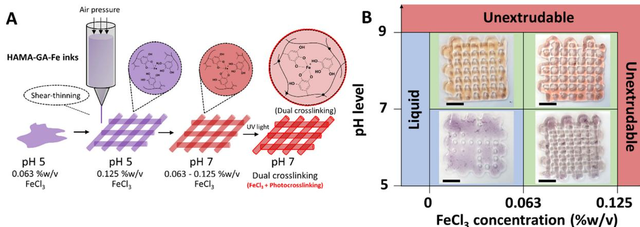
Fig. 7 3D printing of HAMA–GA–Fe biomaterial inks. (A) The illustration of 3D printed structures, which the printability of inks depends on the sol–gel transition caused by pH level (5 and 4) and  $\text{FeCl}_3$  concentrations (0.063 and 0.125% w/v). The stability of the printed structures was enhanced by photocrosslinking after printing. (B) Printability of HAMA–GA by varying pH level and  $\text{FeCl}_3$  concentrations. Scale bar = 1 cm.
