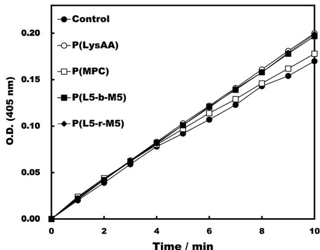
Fig. 3 Activation test of Plm in the presence of polymers. [LysAA units in polymer] = 0.175 mg mL<sup>-1</sup>, [Plm] = 0.05 mg mL<sup>-1</sup>, [S-2251] = 0.35 mmol L<sup>-1</sup>, [t-PA] = 0.04 μg mL<sup>-1</sup>.
