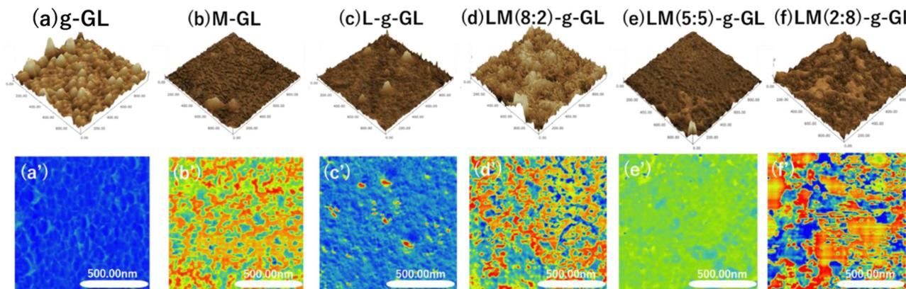
**Fig. 8** Height (a)–(f) and phase (a')–(f') images of surface-treated glass substrate, LysAA, and LysAA-co-MPC grafted polymer by AFM. Scanning area ( $1.0 \mu\text{m}^2$ ), cantilever spring constant ( $1.7 \text{ N m}^{-1}$ ), height (0–30 nm), phase (0–90 degree). The closer the height image is black, the higher the relative height. Phase images have higher relative viscoelasticity the closer to red they are, and vice versa for blue. Green is in between.
