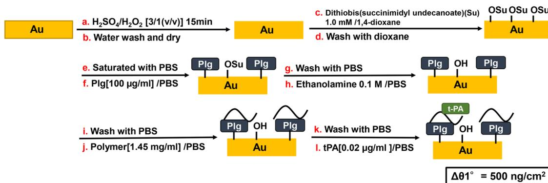
Scheme 5 Au substrate preparation and SPR measurement procedure.
