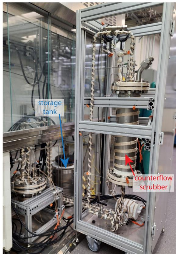
Fig. 2 Molten hydroxide (NaOH-KOH eutectic) showing interior before insulation. The external salt storage tank is shown on the left. This figure was modified from the original by McFarlane *et al.*<sup>89</sup> and reprinted with permission.
