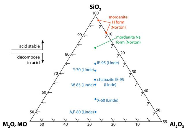
**Fig. 11**  $\text{SiO}_2\text{-Al}_2\text{O}_3\text{-M}_x\text{O}$  ( $M$  = alkali or alkaline earth,  $x$  = 1 or 2) ternary diagram for zeolite minerals that shows the acid stability<sup>8</sup> (this drawing was modified from ORNL drawing 78-15097<sup>152</sup>).
