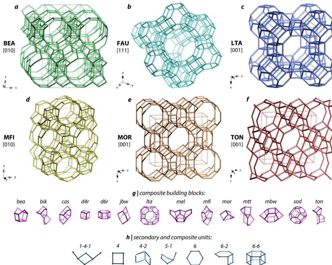
**Fig. 10** Crystal structure schematics for (a) BEA, (b) FAU, (c) LFA, (d) MFI, (e) MOR, and (f) TON zeolites. The main unit cell structures are shown at the top and (g) composite building blocks as well as (h) secondary and composite units present within these zeolites are shown below the main structures. Reproduced in part with permission from Riley *et al.*<sup>119</sup> Copyright 2022 American Chemical Society. Reproduced in part with permission from Baerlocher *et al.*<sup>151,152</sup>
