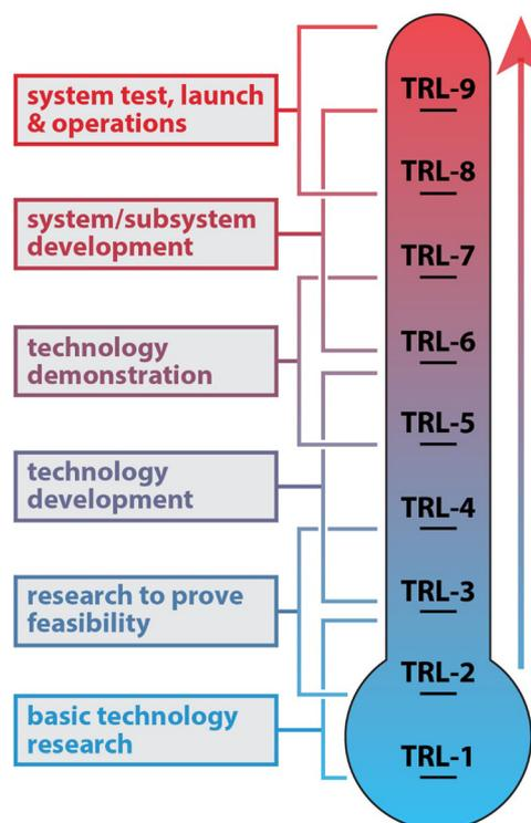
Fig. 5 Technology readiness level (TRL) diagram.<sup>112,113</sup>
