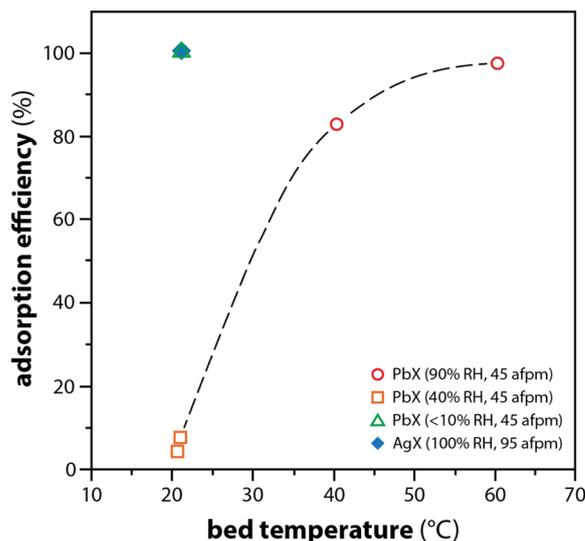
Fig. 4 Comparison of I<sub>2(g)</sub> adsorption efficiency as a function of temperature for PbX and Ag. AFPM refers to actual feet per minute (face velocity). This graphic was modified from the original by Maeck and Pence<sup>16</sup> and Staples *et al.*<sup>106</sup>
