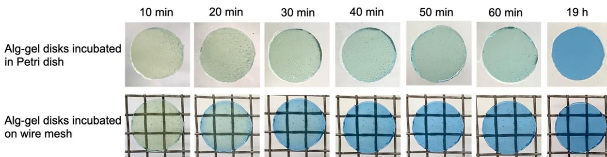
Fig. 3 pH changes of Alg-gel disks incubated in a Petri dish and on a wire mesh containing BTB over time ( $t = 0$  refers to the time when carbonated water was added). The diameter of Alg-gel disks was  $\sim 17.5$  mm, and the thickness was  $3.46 \pm 0.26$  mm.
