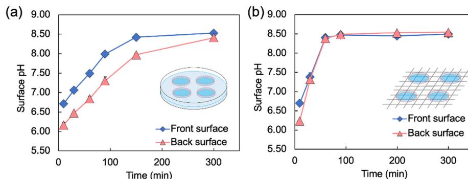
Fig. 4 Changes in the surface pH of Alg-gel disks incubated (a) in a Petri dish\* and (b) on a wire mesh over time ( $t = 0$  refers to the time when carbonated water was added). The thickness of the Alg-gel disks was  $3.46 \pm 0.26$  mm. Values are expressed as the mean  $\pm$  SE obtained from  $n = 3-4$ . \* This result has been reproduced from previous our study.<sup>19</sup>
