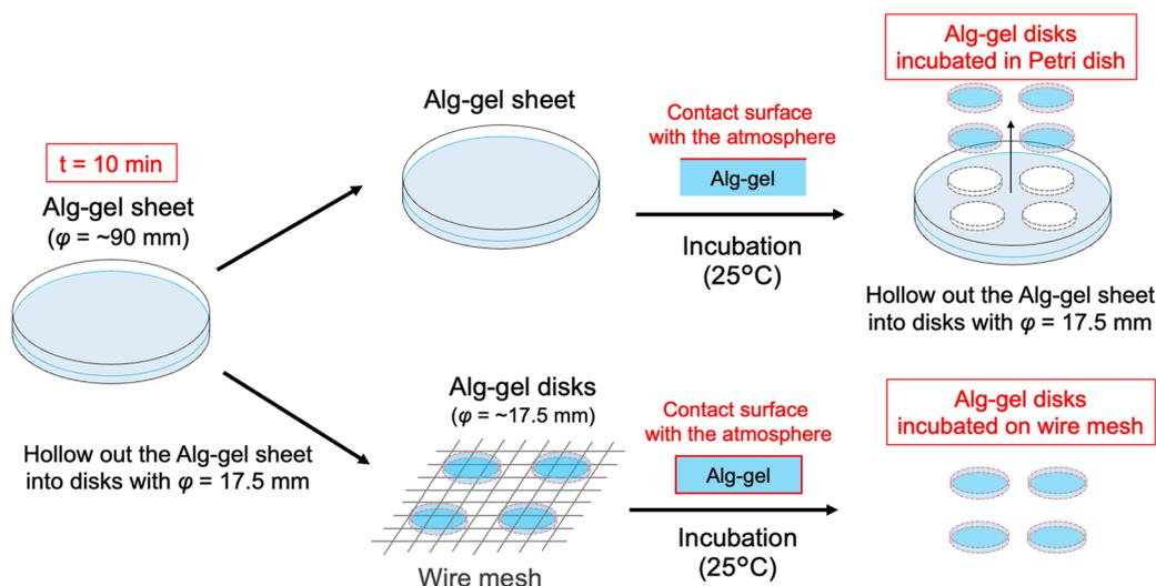
Fig. 2 Schematic of Alg-gel disks incubated in a Petri dish and on a wire mesh.  $t = 0$  refers to the time as carbonated water was added.
