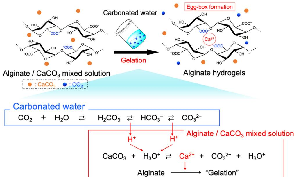
Fig. 1 The gelation mechanism of alginate hydrogels prepared with CaCO<sub>3</sub> and carbonated water.
