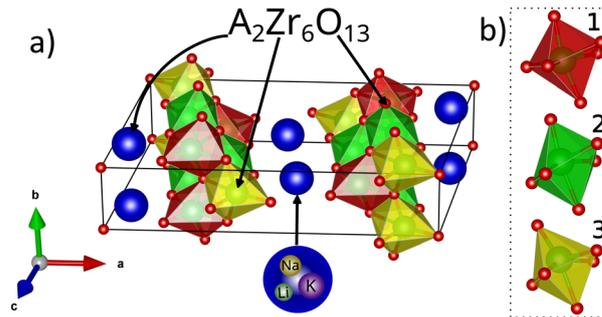
Fig. 1 (a) Monoclinic  $\text{A}_2\text{Zr}_6\text{O}_{13}$  ( $\text{A} = \text{Li}^+$ ,  $\text{Na}^+$ , and  $\text{K}^+$ ) in the conventional  $C2/m$  space group representation, and (b) various  $[\text{ZrO}_2]$  octahedra. The numbers and colors denote equivalent  $[\text{ZrO}_2]$  octahedra. Blue, red, and green spheres represent  $\text{A}^+$ ,  $\text{O}^{2-}$ , and  $\text{Zr}^{4+}$  ions, respectively.
