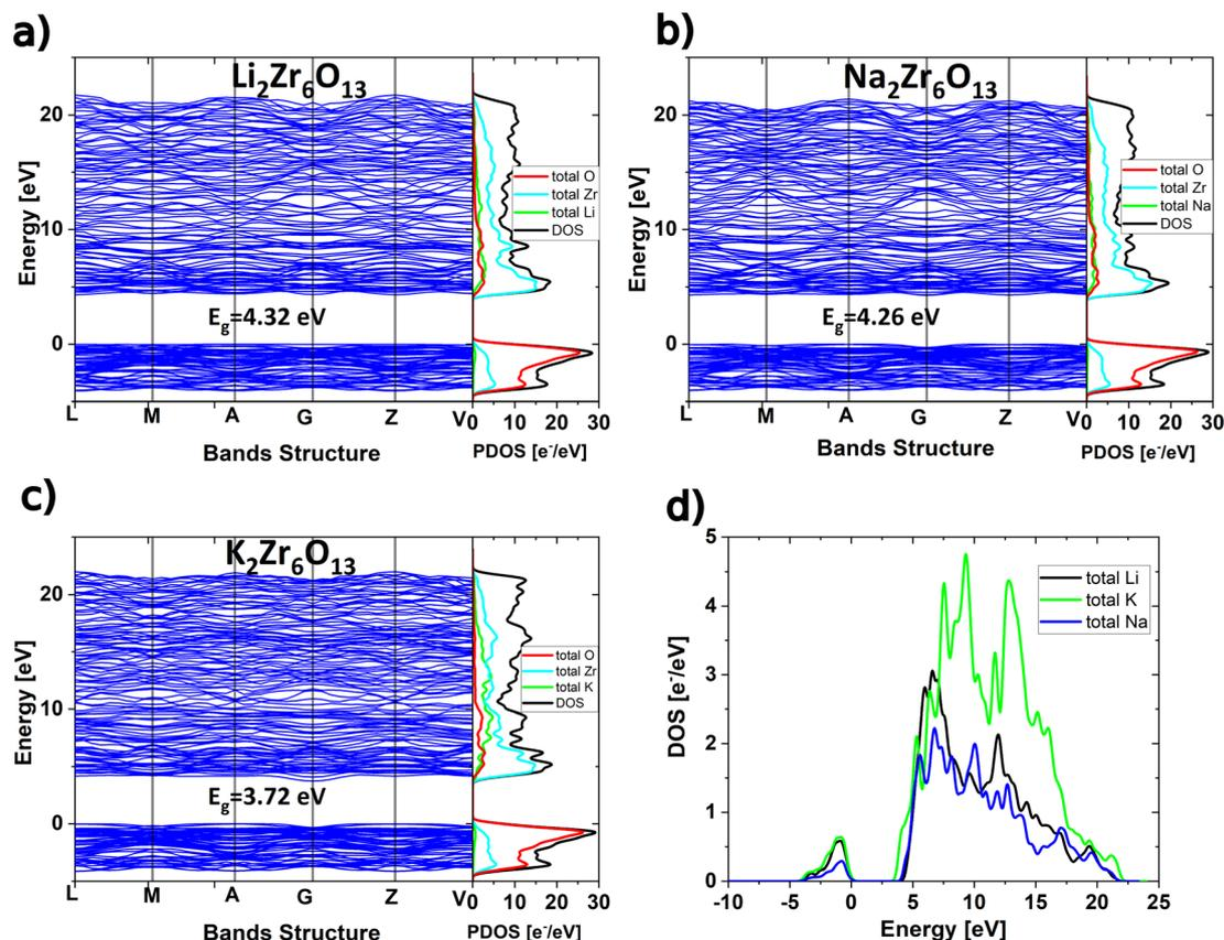
Fig. 2 Band structure and density of states of (a)  $\text{Li}_2\text{Zr}_6\text{O}_{13}$ , (b)  $\text{Na}_2\text{Zr}_6\text{O}_{13}$ , and (c)  $\text{K}_2\text{Zr}_6\text{O}_{13}$  compounds, respectively. (d) DOS of Alkali ions in each  $\text{A}_2\text{Zr}_6\text{O}_{13}$ .
