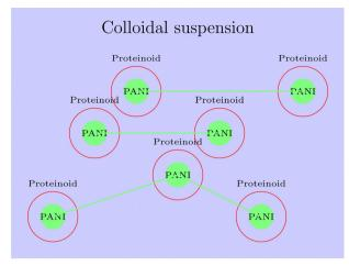
Fig. 19 The diagram shows colloidal suspensions of PANI nanoparticles and proteinoid microspheres. PANI nanoparticles are green, proteinoid proteinoids are red. Blue indicates colloidal suspension. The composite's PANI nanoparticle connections form a conductive network. This diagram shows how to efficiently create colloidal suspensions of PANI nanoparticles encapsulated and interconnected by proteinoid microspheres, which improves electrical characteristics and has several applications.
