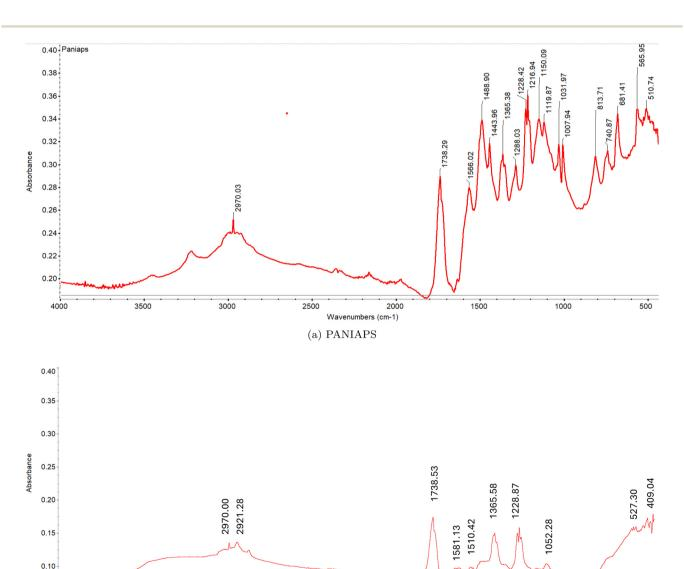
Fig. 20 FT-IR spectra of PANI synthesized using (a) ammonium persulfate (PANIAPS) and (b) ferrous nitrate (PANInitrate) as oxidizing agents.
