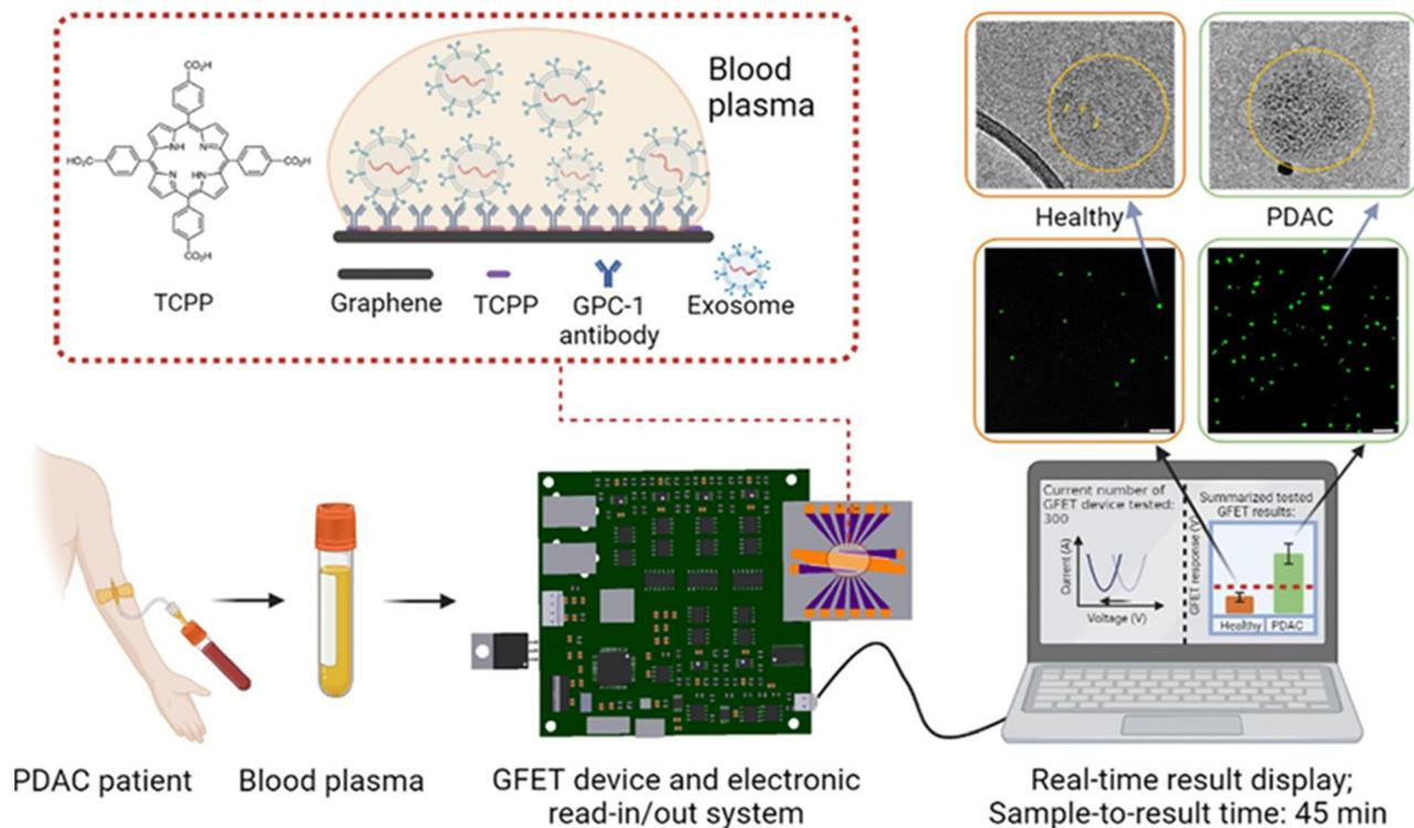
**Fig. 3** Schematics of detection of PDAC exosomes using graphene-based sensors (GFETs with portable electronics and real-time detection results). The total detection time from applying blood plasma on the GFETs to results is less than 45 min. Reproduced with permission.<sup>45</sup> Copyright 2023 American Chemical Society.
