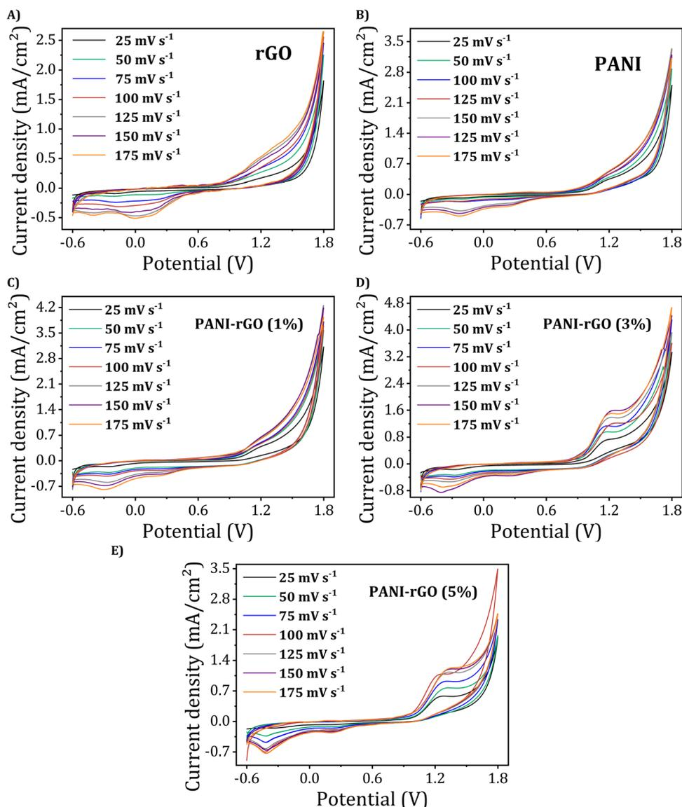
Fig. 12 Cyclic voltammograms of (A) rGO, (B) PANI, and PANI/rGO nanocomposites (C)–(E) at different scan rates.
