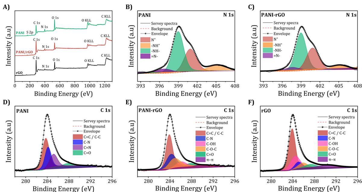
Fig. 11 XPS surveys with (A) the broad high-resolution spectrum of the (B and C) N 1s and (D-F) C 1s areas for pure PANI, rGO, and PANI/rGO nanocomposites (3 wt%).
