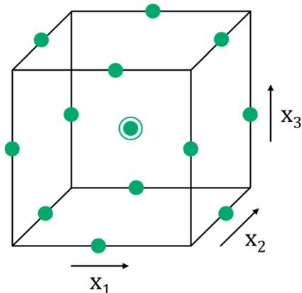
Fig. 2 Configuration of the Box-Behnkendesign for a three-factor system.
