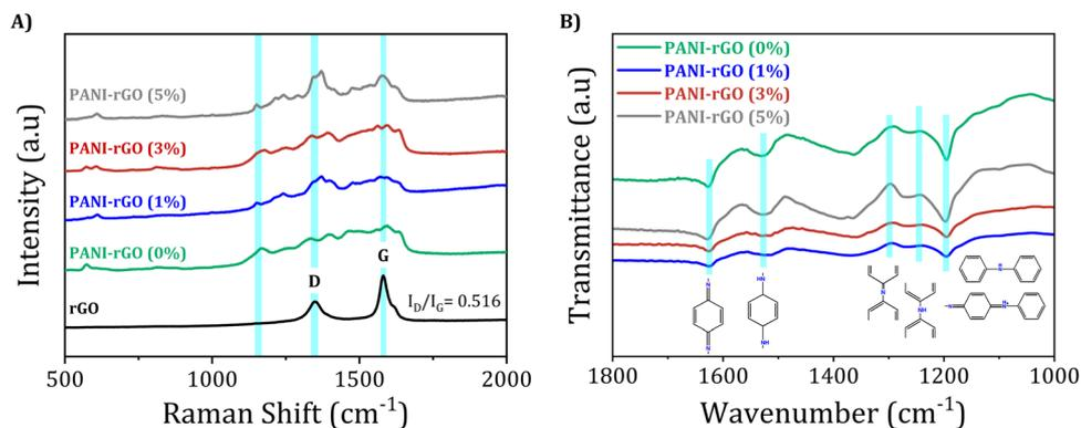
Fig. 9 (A) Raman spectra and (B) FT-IR spectrum of pure PANI, rGO, and PANI/rGO nanocomposites.
