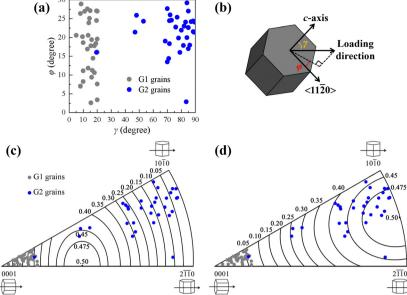
Fig. 3 (a)  $\gamma$  and  $\varphi$  angle distributions of G1 and G2 grains. (b) Schematic diagram of  $\gamma$  and  $\varphi$  angles. (c) and (d) Crystallographic orientations of G1 and G2 grains, plotted on the IPF map with contours of the (c) basal Schmid factor and (d) prismatic Schmid factor.
