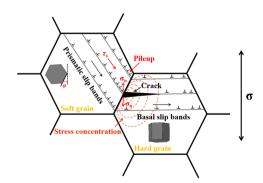
Fig. 7 Schematic diagram of dwell fatigue cracking involving dislocation pile up at the soft/hard GB. Stress concentration induces dislocation activation and normal stress  $(\sigma_n)$  on the basal plane of the hard grain. Combined with the applied stress ( $\sigma$ ), the normal stress leads to the crack nucleation.
