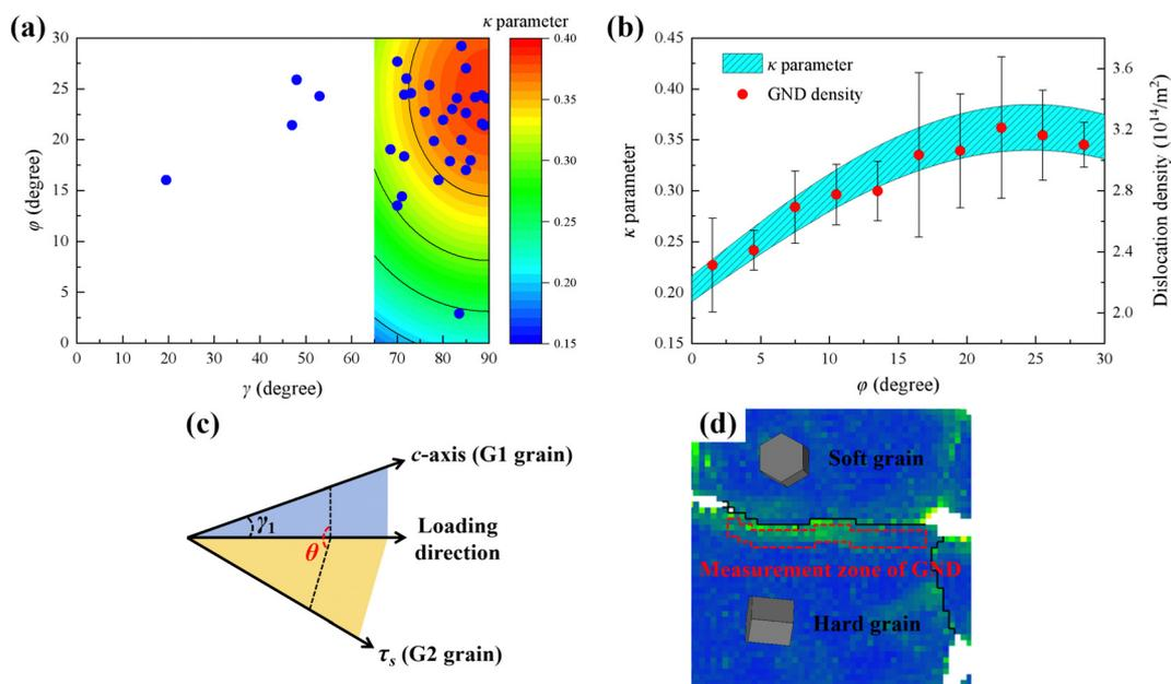
Fig. 6 (a)  $\kappa$  parameter of  $\alpha$  grains related to  $\gamma$  and  $\phi$  angles.  $\gamma$  and  $\phi$  angle distributions of G2 grains (blue solid circle) are plotted in (a). (b)  $\kappa$  parameter of  $\alpha$  grains with  $70^\circ \leq \gamma \leq 90^\circ$  and the mean GND density of hard grains near soft/hard GBs. (c) Schematic diagram of the dihedral angle  $\theta$ . (d) The measurement zone of GND. The mean standard error is used as the error bar.
