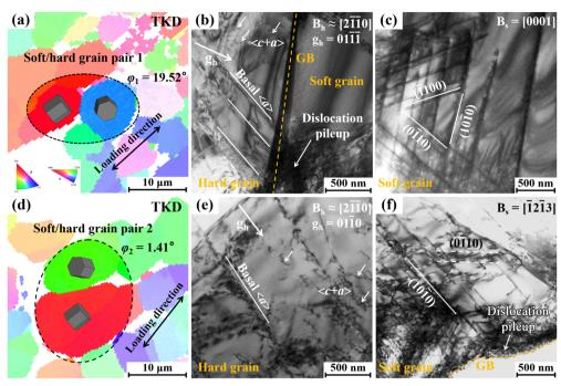
Fig. 5 (a) and (d) TKD-IPF maps of soft/hard grain pairs; crystallographic orientation is relative to the loading direction. Bright field TEM images of dislocation activities in (b) and (c) soft/hard grain pair 1 ( $\varphi_1 = 19.52^{\circ}$ ) and (e) and (f) soft/hard grain pair 2 ( $\varphi_2 = 1.41^{\circ}$ ). GBs are denoted by yellow dashed lines.
