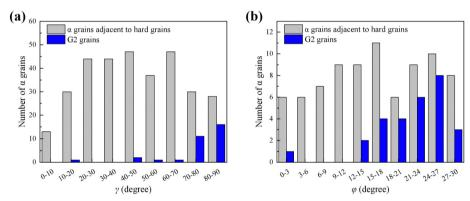
Fig. 4 (a)  $\gamma$  angle distribution of G2 grains and  $\alpha$  grains adjacent to uncracked hard grains. (b)  $\varphi$  angle distribution of G2 grains and  $\alpha$  grains adjacent to uncracked hard grains when  $65^{\circ} \le \gamma \le 90^{\circ}$ .
