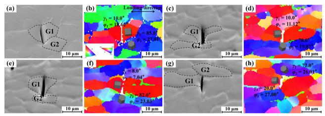
Fig. 2 (a), (c), (e) and (g) Raw SEM secondary electron images after crack initiation and the corresponding (b), (d), (f) and (h) EBSD-IPF maps. The crystallographic orientation is relative to the loading direction.
