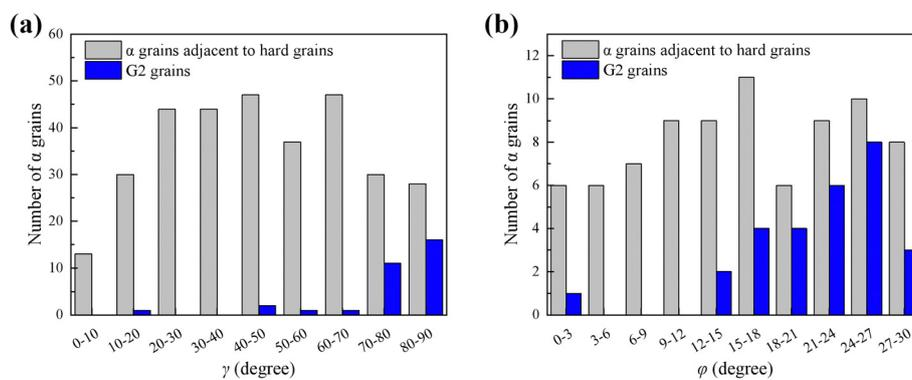
Fig. 4 (a)  $\gamma$  angle distribution of G2 grains and  $\alpha$  grains adjacent to uncracked hard grains. (b)  $\phi$  angle distribution of G2 grains and  $\alpha$  grains adjacent to uncracked hard grains when  $65^\circ \leq \gamma \leq 90^\circ$ .
