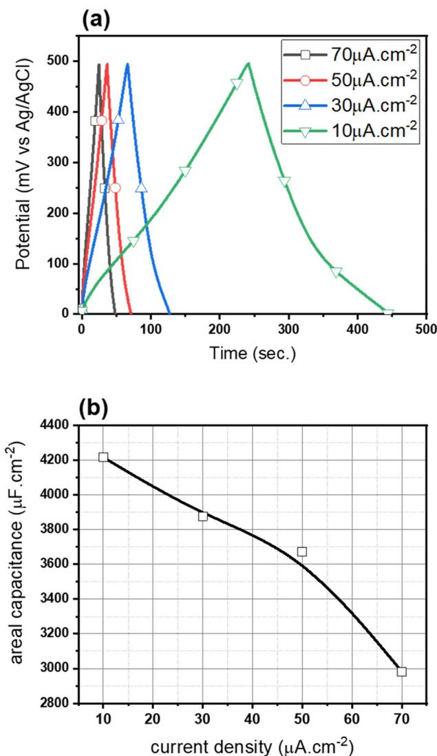
**Fig. 5** (a) Galvanostatic charge–discharge curves of TNT-R at different current densities from 10 to  $70 \mu\text{A cm}^{-2}$  and (b) the areal capacitance of TNT-R at different current densities from 10 to  $70 \mu\text{A cm}^{-2}$ .
