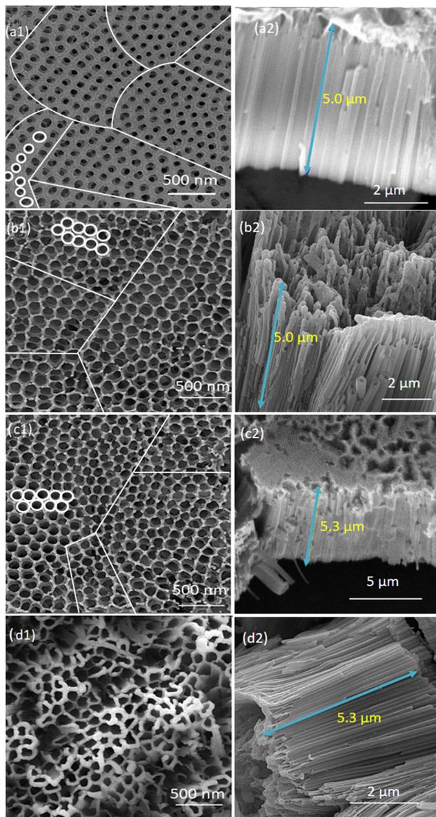
Fig. 2 FE-SEM image of  $\text{TiO}_2$  anodised for (a1) TNT-1h-30min, (b1) TNT-4h-30min, (c1) TNT-4h-1h and (d1) reduced  $\text{TiO}_2$ , and correlated cross section of  $\text{TiO}_2$  anodised for (a2) TNT-1h-30min, (b2) TNT-4h-30min, (c2) TNT-4h-1h, and (d2) reduced  $\text{TiO}_2$ .
