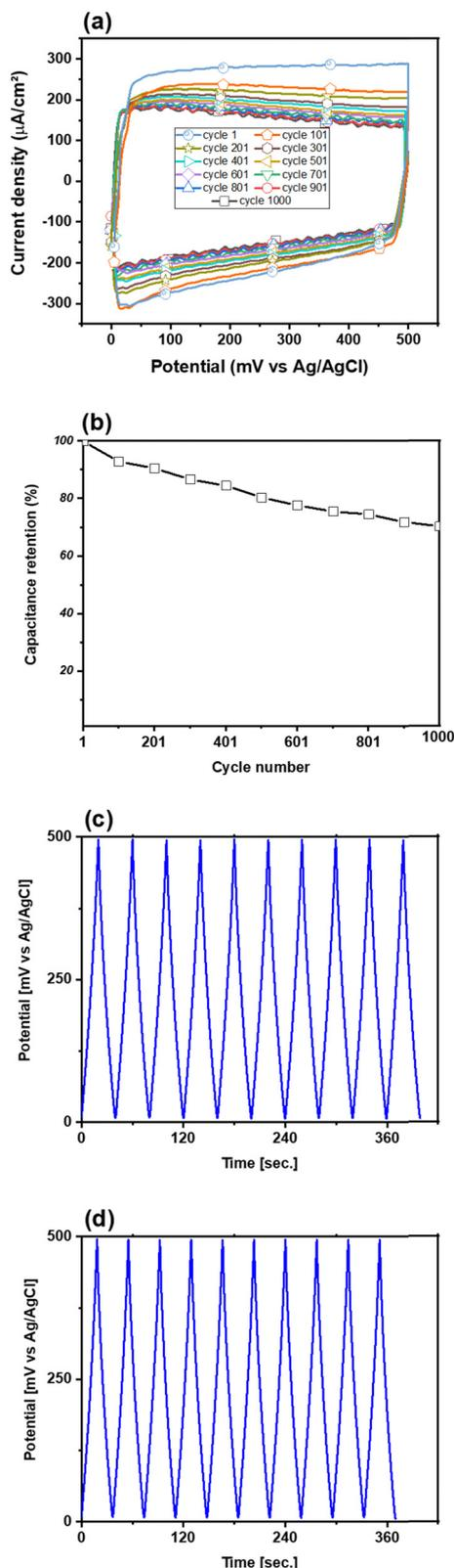
Fig. 7 (a) CV curves at a scan rate of  $80 \text{ mV s}^{-1}$  (1000 cycle number), (b) areal capacitance retention, (c) charge–discharge curve in the first 10 cycles and (d) charge–discharge curve in the last 10 cycles during 1000 cycles.
