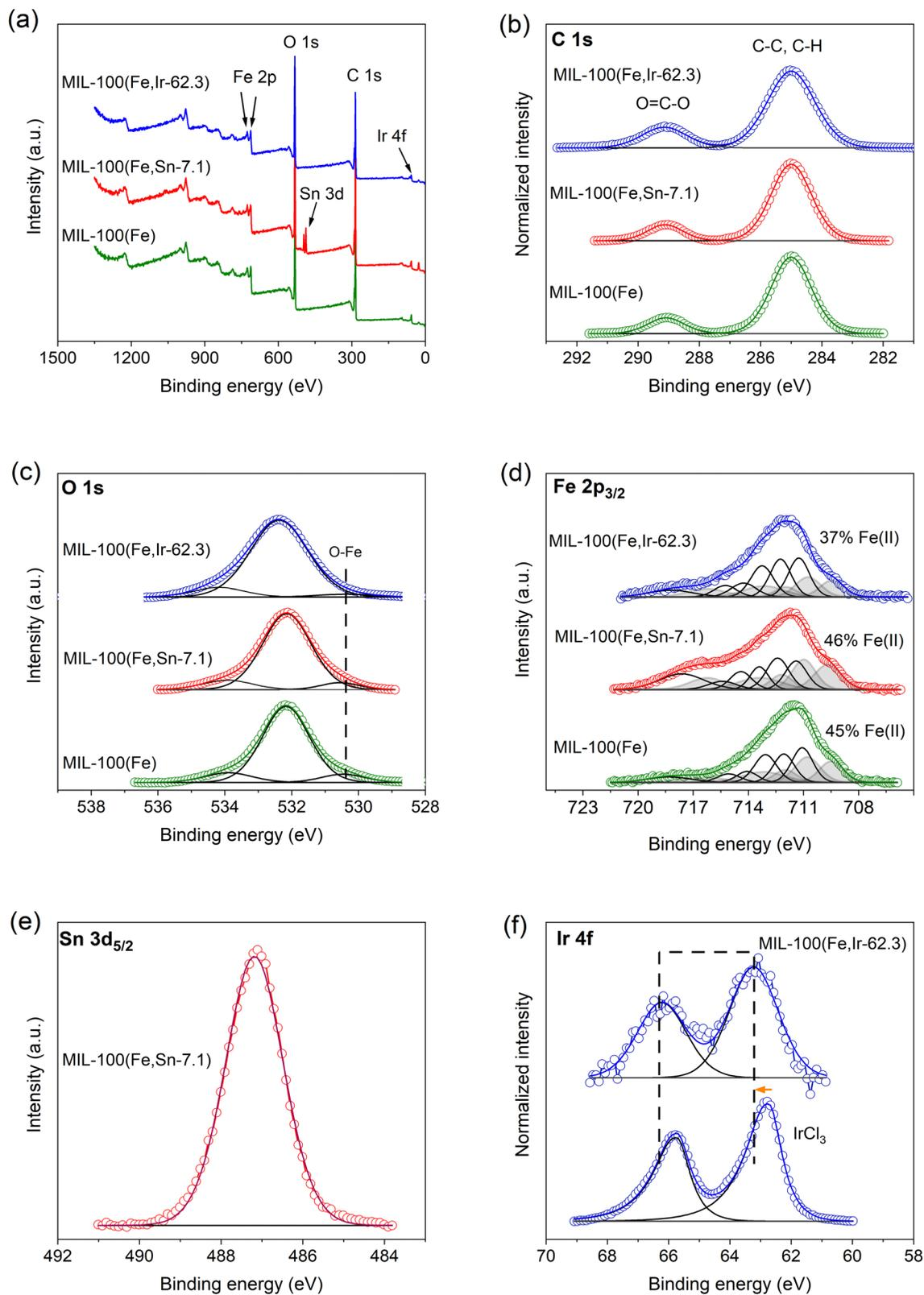
Fig. 8 XPS (a) survey spectra, (b) C 1s, (c) O 1s and (d) Fe 2p<sub>3/2</sub> spectra of MIL-100(Fe), MIL-100(Fe,Sn-7.1), and MIL-100(Fe,Ir-62.3). (e) Sn 3d<sub>5/2</sub> spectrum of MIL-100(Fe,Sn-7.1). (f) Ir 4f spectrum of MIL-100(Fe,Ir-62.3) compared to the reference IrCl<sub>3</sub>·xH<sub>2</sub>O.
