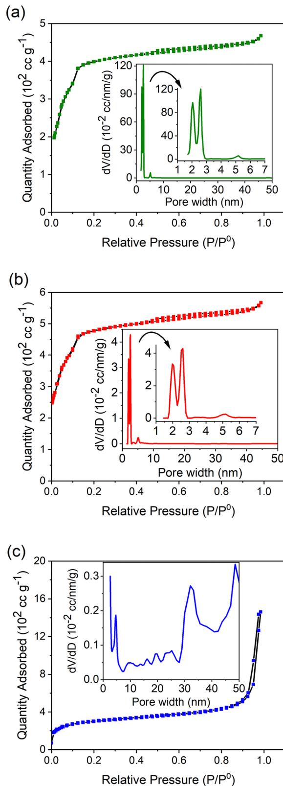
Fig. 7 Nitrogen adsorption-desorption isotherms of the (a) MIL-100(Fe), (b) MIL-100(Fe,Sn-7.1), and (c) MIL-100(Fe,Ir-62.3). The insets show the corresponding pore-size distribution curve calculated from the adsorption branch of the nitrogen isotherm.
