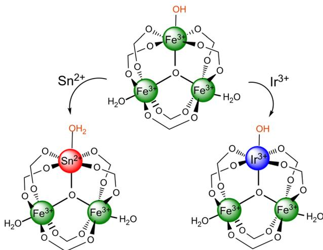
Scheme 1 MIL-100(Fe) (up-middle), MIL-100(Fe,Sn) (bottom-left), and MIL-100(Fe,Ir) (bottom-right).
