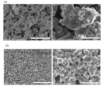
Fig. 3 SEM images of (a) LAM01 pristine powders annealed at 975  $^{\circ}$ C for 100 h in air and (b) LAM01 and 8YSZ powders mixed at a weight ratio of 1:1 and annealed at 975  $^{\circ}$ C for 100 h in air.
