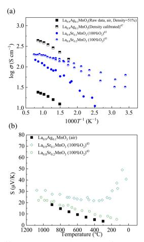
Fig. 5 (a) Electrical conductivity of Ag doped LaMnO $_3$  measured in air. The bulk conductivity of Ag doped LaMnO $_3$  was calibrated by density correction factors.  $^{47}$  (b) Absolute Seebeck coefficients of Ag doped LaMnO $_3$  measured in air. For comparison, those of LSM measured in 100% O $_2$  are also shown.  $^{43}$
