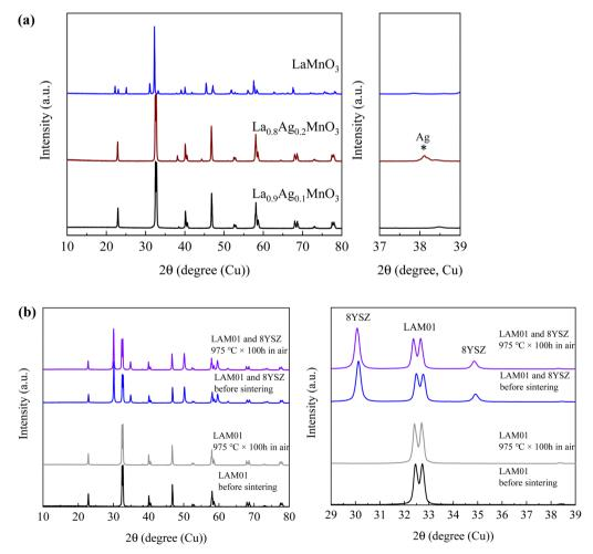
Fig. 1 XRD profiles of (a) Ag- and undoped LaMnO<sub>3</sub> and (b) LAM01 powder and mixed powder of LAM01 and 8YSZ before and after annealing at 975 °C.
