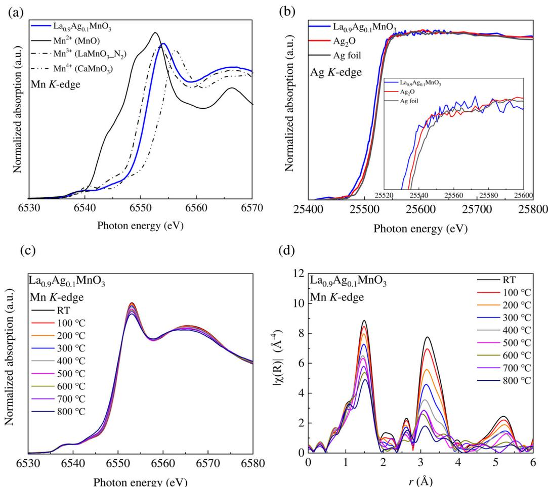
Fig. 4 (a) *Ex situ* Mn K-edge XANES spectra, (b) *ex situ* Ag K-edge XANES spectra of LAM01 at room temperature. (c) *in situ* Mn K-edge XANES spectra and (d) amplitude of Fourier transformed obtained from EXAFS oscillation of LAM01 from room temperature to 800 °C in air. The weighted spectra were Fourier transformed in a  $k$  space of 3 to 12  $\text{\AA}^{-1}$ .
