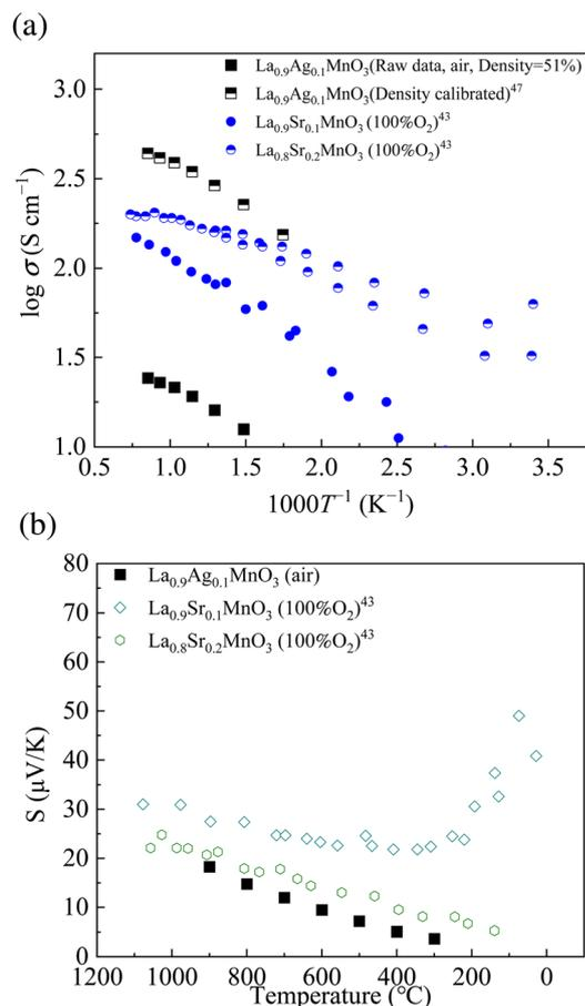
Fig. 5 (a) Electrical conductivity of Ag doped LaMnO<sub>3</sub> measured in air. The bulk conductivity of Ag doped LaMnO<sub>3</sub> was calibrated by density correction factors.<sup>47</sup> (b) Absolute Seebeck coefficients of Ag doped LaMnO<sub>3</sub> measured in air. For comparison, those of LSM measured in 100% O<sub>2</sub> are also shown.<sup>43</sup>
