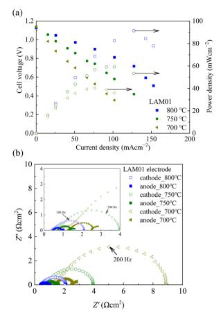
Fig. 6 (a) Power generation characteristic curves and (b) impedance profiles of the LAM01 cell baked at 925  $^{\circ}$ C.
