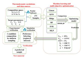
Fig. 1 Design workflow of L1<sub>2</sub>-strengthened SX-HEAs aided by machine learning and multi-objective optimization.
