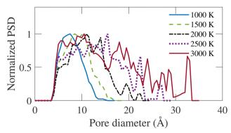
Fig. 9 Normalized pore size distribution (PSD) for annealed structures at different simulation temperatures ( $T_s$ ).
