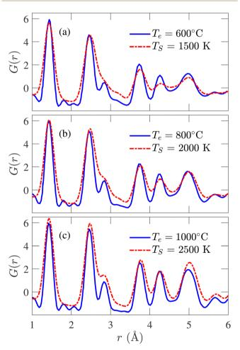
**Fig. 6** Comparison between simulated and experimental pair distribution functions (PDFs) obtained from X-ray diffraction for simulation temperature ( $T_S$ ) of (a) 1500 K, (b) 2000 K, and (c) 2500 K. The experimental results are reported by Forse *et al.* <sup>64</sup>
