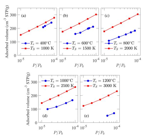
Comparison between the experimental and GCMC simulation generated argon adsorption isotherm at 77 K and low-pressure region for structures developed at different temperatures. The experimental data is reported by Dash et al.<sup>6</sup>
