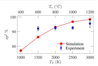
**Fig. 7** Comparison between  $\rm sp^2$ -hybridized atom percentage variations with simulation ( $T_{\rm S}$ ) and experiment ( $T_{\rm e}$ ) temperatures. The experimental data are reported by Gläsel *et al.*<sup>20</sup>
