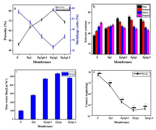
(a) Porosity and percentage shrinkage ratio, (b) solvent content, (c) (PWF) pure water flux, (d) contact angle
