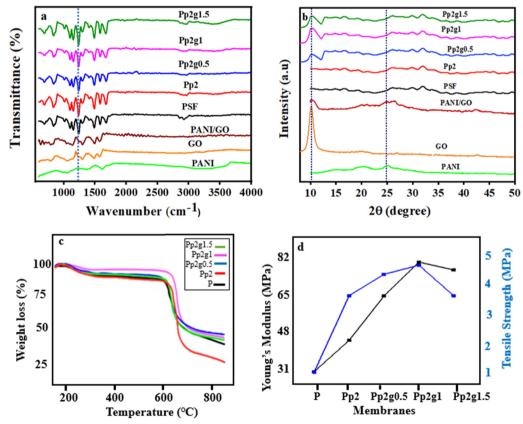
Fig. 4 (a) FTIR spectra of pure PSF, PSF/PANI, and PSF/PANI/GO nanocomposite membranes. (b) XRD diffractogram of PSF, PSF/PANI, and PSF/PANI/ GO nanocomposite membranes. (c) TGA of PSF, PSF/PANI, and PSF/PANI/GO nanocomposite membranes. (d) Tensile properties of PSF, PSF/PANI, and PSF/PANI/GO nanocomposite membranes.
