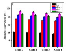
Fig. 6 (a) BSA rejection of pristine PSF P and composite membrane Pp2, Pp2g0.5, Pp2g1.5. (b) Flux recovery ratio of pristine PSF P and composite membrane Pp2, Pp2g0.5, Pp2g1, Pp2g1.5
