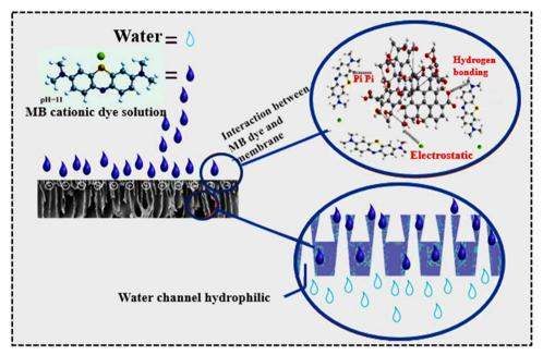
Fig. 7 Proposed diffusion mechanism through the PSF/PANI/GO nanocomposite membranes adsorptive removal of MB dye from a wastewater sample.
