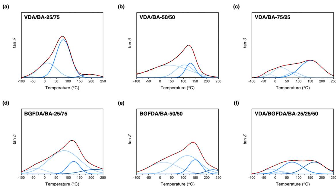
Fig. 2 Deconvolution of  $\tan \delta$  curves of acrylate networks. The red dashed line (---) denotes the original curve, and the black solid line (—) is the integrated result of deconvoluted curves. All y-axes are on the same scale.
