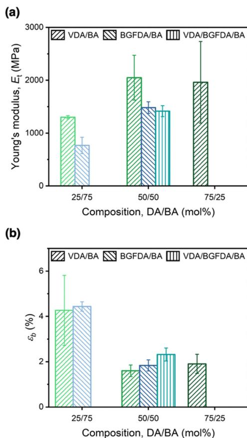
Fig. 4 (a) Young's modulus ( $E_t$ ) and (b) elongation at break ( $\varepsilon_b$ ) of acrylate networks. Error bars represent the standard deviations from triplicate measurements.
