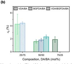
Fig. 4 (a) Young's modulus ( $E_t$ ) and (b) elongation at break ( $\varepsilon_b$ ) of acrylate networks. Error bars represent the standard deviations from triplicate measurements.
