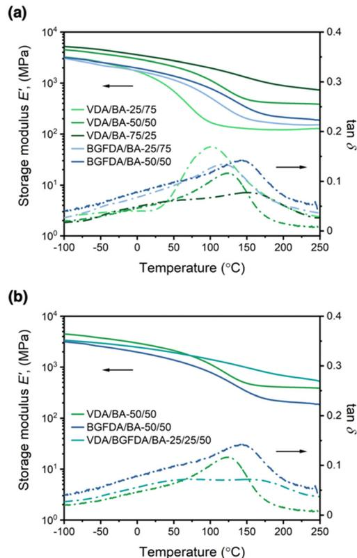
Fig. 1 Storage modulus (solid line, —) and  $\tan \delta$  (dashed line, ---) as a function of temperature for (a) varying diacrylate content and (b) varying diacrylate type with a total diacrylate content at 50 mol%.
