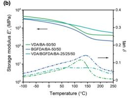
Fig. 1 Storage modulus (solid line, -) and  $\tan \delta$  (dashed line, ---) as a function of temperature for (a) varying diacrylate content and (b) varying diacrylate type with a total diacrylate content at 50 mol%
