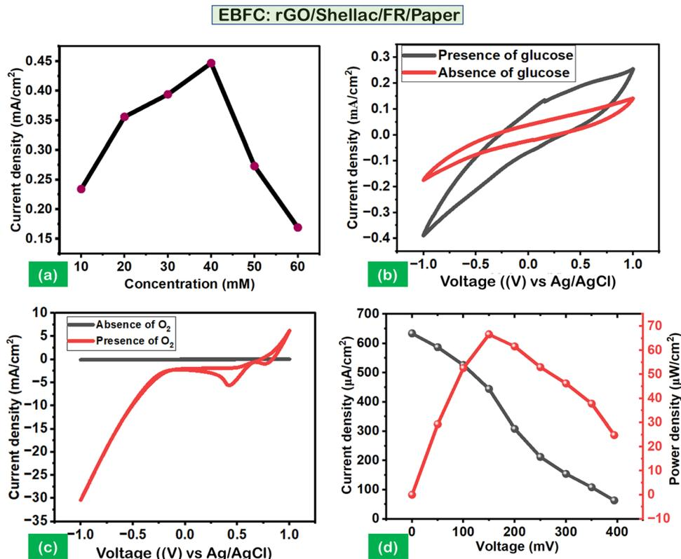
Fig. 7 Enzymatic biofuel cell (EBFC) using the biopolymer-assisted rGO electrodes on paper, (a) concentration study of fuel (glucose); (b) analysis of anodic modification by GO<sub>x</sub> with Ag/AgCl reference electrode; (c) analysis of cathodic modification by laccase, with Ag/AgCl, reference electrode and (d) power density (PD) analysis through polarization studies.
