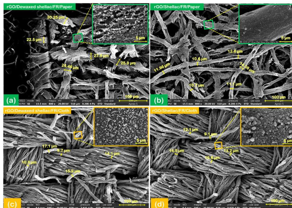
Fig. 3 Field emission scanning electron microscopy images: (a) LirGO/Dewaxed shellac/FR/Paper (Inset: 5  $\mu\text{m}$  and 100  $\mu\text{m}$  high-resolution images), (b) LirGO/Shellac/FR/Paper, (c) LirGO/Dewaxed shellac/FR/Cloth, and (d) LirGO/Shellac/FR/Cloth (all insets: 100  $\mu\text{m}$  high-resolution images, shown separately in ESI<sup>†</sup> (Fig. S19)).
