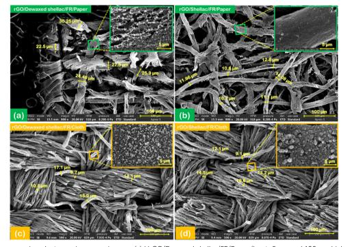
Fig. 3 Field emission scanning electron microscopy images: (a) LIrGO/Dewaxed shellac/FR/Paper (Inset: 5 μm and 100 μm high-resolution images), (b) LIrGO/Shellac/FR/Paper, (c) LIrGO/Dewaxed shellac/FR/Cloth, and (d) LIrGO/Shellac/FR/Cloth (all insets: 100 μm high-resolution images, shown separately in ESI† (Fig. S19)).
