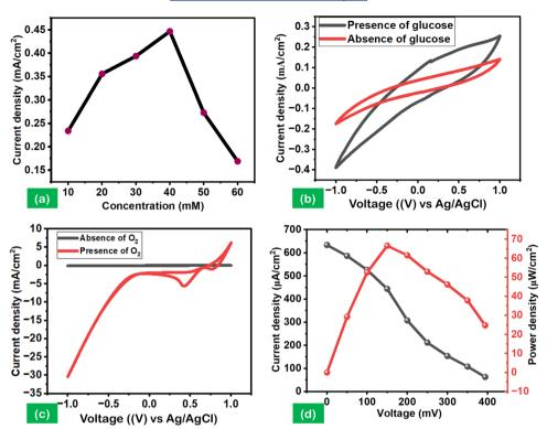
Fig. 7 Enzymatic biofuel cell (EBFC) using the biopolymer-assisted rGO electrodes on paper, (a) concentration study of fuel (glucose); (b) analysis of anodic modification by GO<sub>x</sub>, with Ag/AgCl reference electrode; (c) analysis of cathodic modification by laccase, with Ag/AgCl, reference electrode and (d) power density (PD) analysis through polarization studies.
