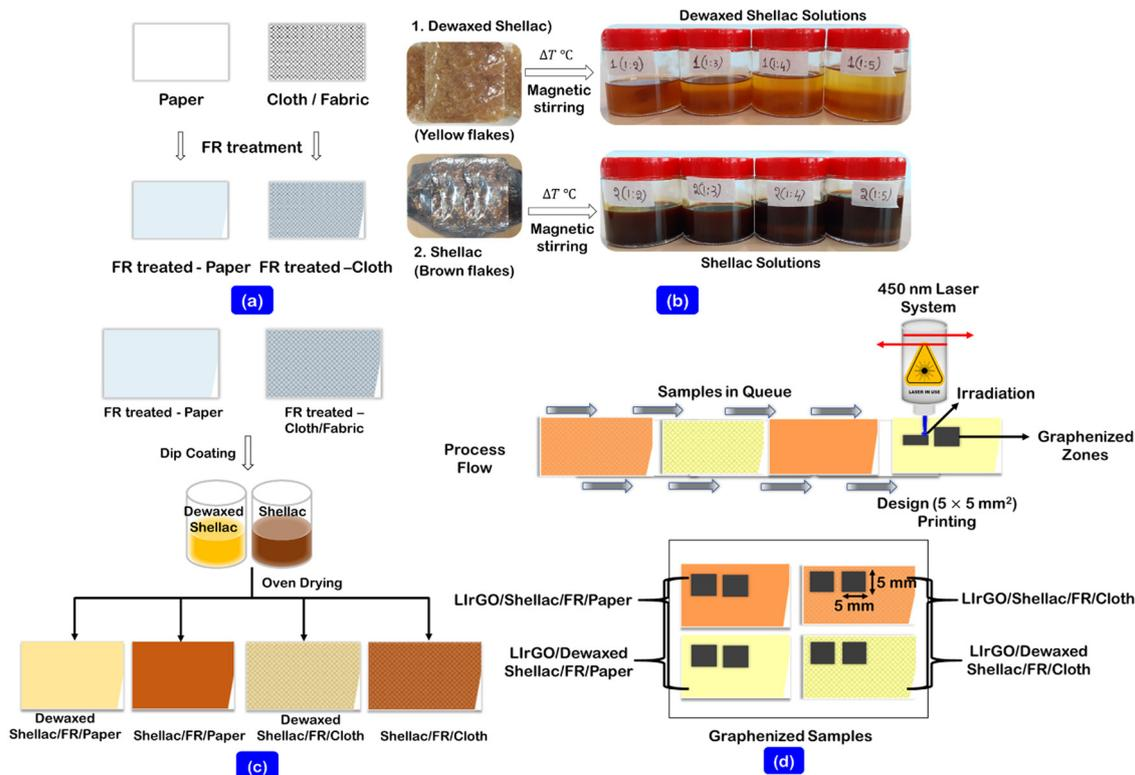
**Fig. 1** Prior treatments for paper and cloth substrates, (a) FR treatments for both substrates, (b) the preparation of uniform biopolymer (DS and S) solutions from raw flakes, (c) process of biopolymer coatings on both substrates, and (d) process flow of laser irradiations to obtain  $5 \times 5 \text{ mm}^2$  graphenized patterns on both the biopolymer-assisted substrates.
