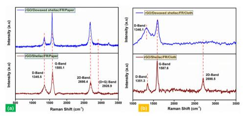
Fig. 6 Raman analysis in identifying structural disorders, (a) analysis of rGO developed on biopolymer-assisted paper samples and (b) analysis of rGO developed on biopolymer-assisted cloth samples.
