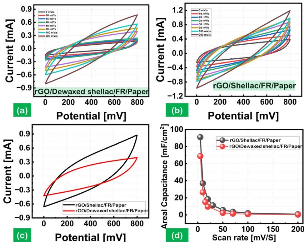
Fig. 8 Supercapacitor cyclic voltammetry (CV) analysis for the developed rGO patterns on paper substrates: (a) scan rate effect of the rGO device developed on Dewaxed Shellac/FR/Paper, (b) scan rate effect of the rGO device developed on Shellac/FR/Paper, (c) scan rate comparisons at  $50 \text{ mV s}^{-1}$  for both developed devices, and (d) areal capacitance analysis concerning the scan rate.
