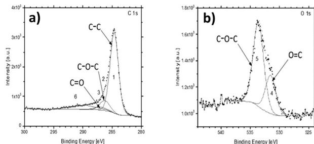
Fig. 3 High-resolution XPS spectra of pyrolyzed PEEK C 1s (a) and O 1s (b).
