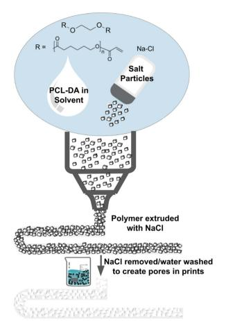
Fig. 1 DIW process to prepare biodegradable, SMP 4D printed structures using a cross-linkable polyester-based ink in which salt particles were used as a rheology modifier and sacrificial porogen.
