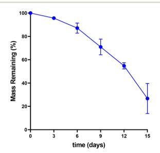
Fig. 6 Mass loss of accelerated degradation (0.2 M NaOH) study.
