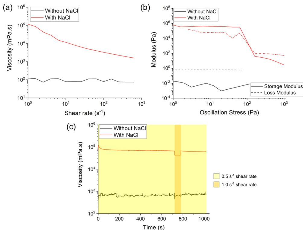
Fig. 2 Comparison of the properties of the polymer solution (no salt, black traces) and ink (with salt, red traces): (a) viscosity as a function of shear rate, (b) storage ( $G'$ ) and loss ( $G''$ ) moduli variations *versus* applied stress, and (c) a three interval thixotropy test varying shear rate across time.
