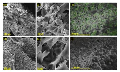
Fig. 4 SEM images of printed and cured samples: (a)-(c) before NaCl removal, and (d)-(f) after NaCl removal. (c) and (f) EDS mapping on SEM images (areen = chlorine)
