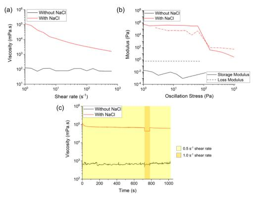
Fig. 2 Comparison of the properties of the polymer solution (no salt, black traces) and ink (with salt, red traces): (a) viscosity as a function of shear rate, (b) storage (G') and loss (G'') moduli variations versus applied stress, and (c) a three interval thixotropy test varying shear rate across time
