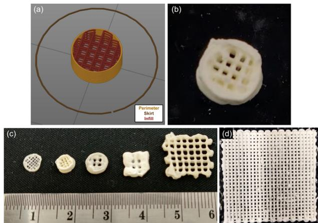
**Fig. 3** DIW printing of shape memory inks and characterization after curing: (a) Prusaslicer design of scaffold, (b) DIW printed scaffold, (c) print nozzle-size-dependent macropore variation, and (d) 50 mm × 50 mm geometry print.
