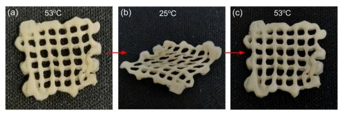
Fig. 5 Shape memory behavior of DIW printed PCL scaffolds: (a) sample after printing, curing, and washing; (b) shape fixity: sample in (a) after being heated to and deformed at 53 °C, then cooled to ambient tempearture; and (c) shape recovery of sample in (b) after heating at 53 °C.
