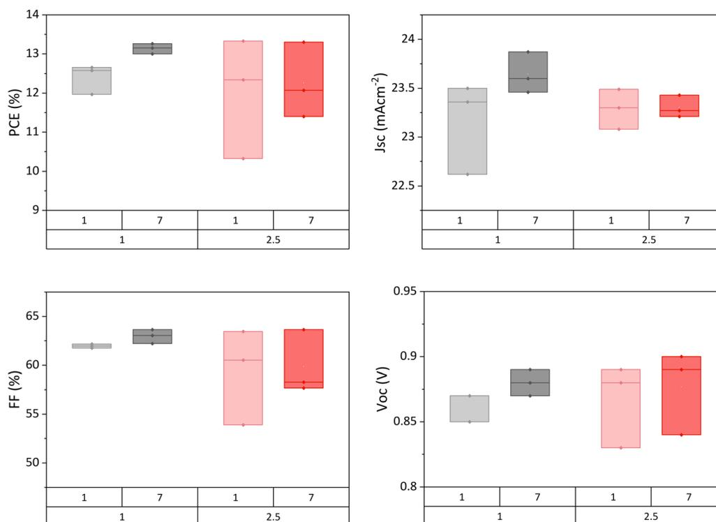
Fig. 6 Performance of GVL-MeOH AVA<sub>0.03</sub>MAPbI<sub>3</sub> devices annealed for 1 or 2.5 hours at  $45\text{ }^{\circ}\text{C}$  1 day and 7 days after fabrication. Four samples in each set.
