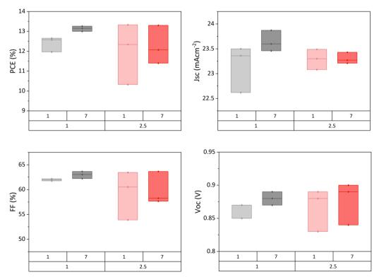
Fig. 6 Performance of GVL-MeOH AVA<sub>0.03</sub>MAPbl<sub>3</sub> devices annealed for 1 or 2.5 hours at 45 °C 1 day and 7 days after fabrication. Four samples in each set
