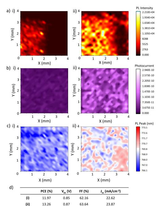
Fig. 3 (a) Photoluminescence maps, (b) Photocurrent maps, (c) PL peak position maps, and (d) PV performance parameters of a device 1 (i) and 8 (ii) days after fabrication.
