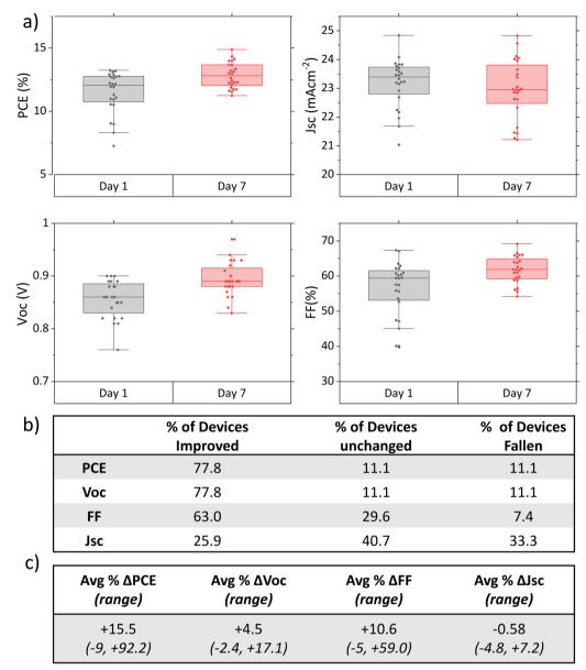
Fig. 2 (a) PV parameters of 27 GVL  $AVA_{0.03}MAPbl_3$  devices from various batches, 1 and 7 days after fabrication. (b) Table showing % of devices that experienced an improvement, no change, or fall in performance. (c) Table showing average and range % change in each PV parameter compared to initial values.
