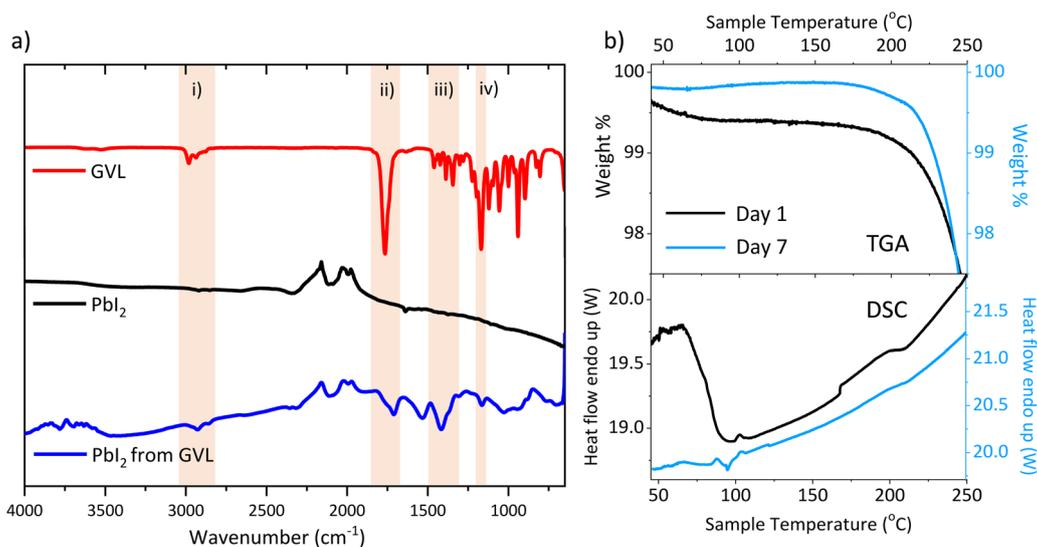
**Fig. 5** (a) FTIR of pure GVL, pure  $PbI_2$  and  $PbI_2$  after drying from GVL at 45 °C. Highlighted sections show notable characteristic GVL peaks, identified in Table S3 (ESI<sup>†</sup>). (b) TGA, derivative weight % and DSC of  $AVA_{0.03}MAPbI_3$  in  $ZrO_2$  24 h (i) and 7 days (ii) after annealing.
