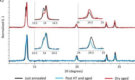
Fig. 1 (a) Diagrammatic representation of a CPSC cross section. (b) Normalised PCEs of GVL CPSCs before and after HT or dry ambient storage. Samples were measured 1 day and 7 days after fabrication, with HT on days 2-3. 14-18 samples in each set. (c) XRD of  $AVA_{0.03}MAPbl_3$  perovskites crystallised from GVL-based precursors in mesoporous ZrO2 scaffolds. Samples were examined directly after annealing (black) and again after exposure to dry ambient air (red) or 70% RH HT (blue)
