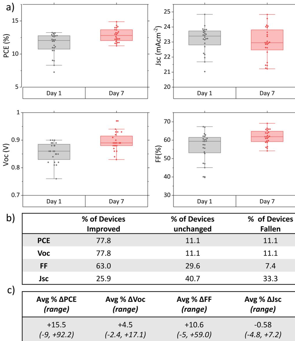
**Fig. 2** (a) PV parameters of 27 GVL AVA<sub>0.03</sub>MAPbI<sub>3</sub> devices from various batches, 1 and 7 days after fabrication. (b) Table showing % of devices that experienced an improvement, no change, or fall in performance. (c) Table showing average and range % change in each PV parameter compared to initial values.
