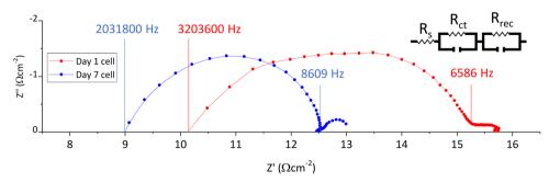
Fig. 4 Nyquist plots of a cell on days 1 and 7, with relevant frequencies labelled for the start and end points of the large first arc.
