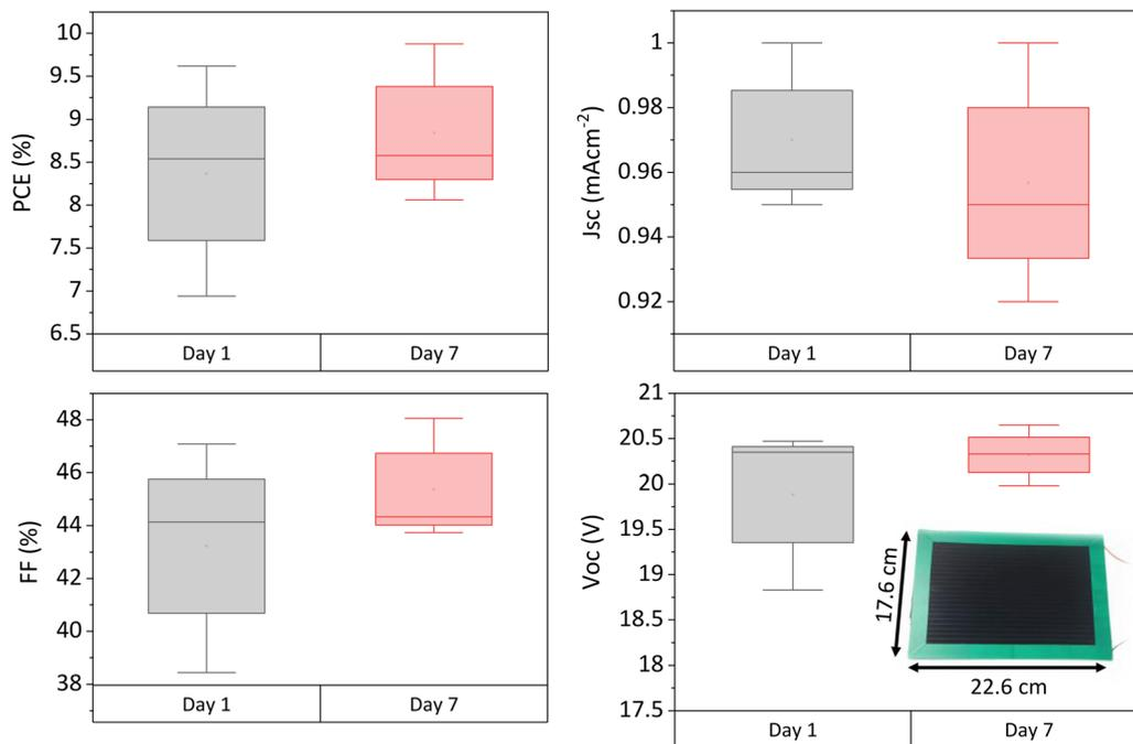
Fig. 7 Photovoltaic parameters of 220 cm<sup>2</sup> modules 1 and 7 days after infiltration. 3 modules tested. Inlaid photograph of a module with substrate measurements.
