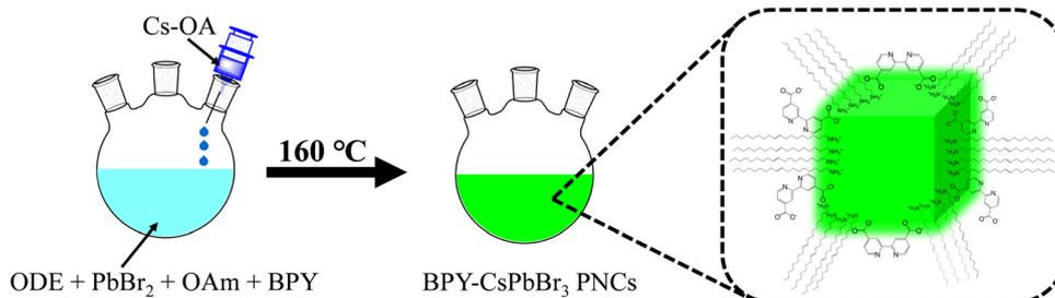
Scheme 1 Synthesis of BPY-CsPbBr<sub>3</sub> PNCs.
