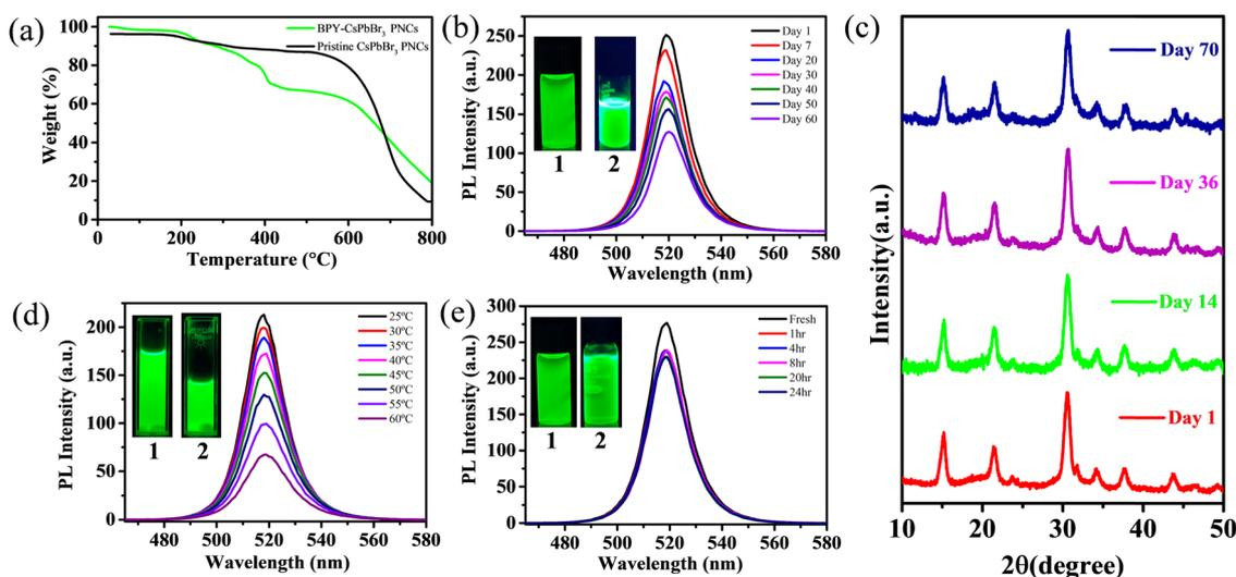
Fig. 4 (a) TGA of pristine and BPY-CsPbBr<sub>3</sub> PNCs; (b) time-dependent PL (inset shows the optical image 1 at day 1 and 2 at day 60); (c) time-dependent XRD pattern of BPY-CsPbBr<sub>3</sub> PNCs; (d) hydrothermal stability (inset shows the optical image 1 at room temperature and 2 at 60 °C); (e) photostability (inset shows the optical image 1 of fresh PNCs and 2 after 24 h of under UV light).
