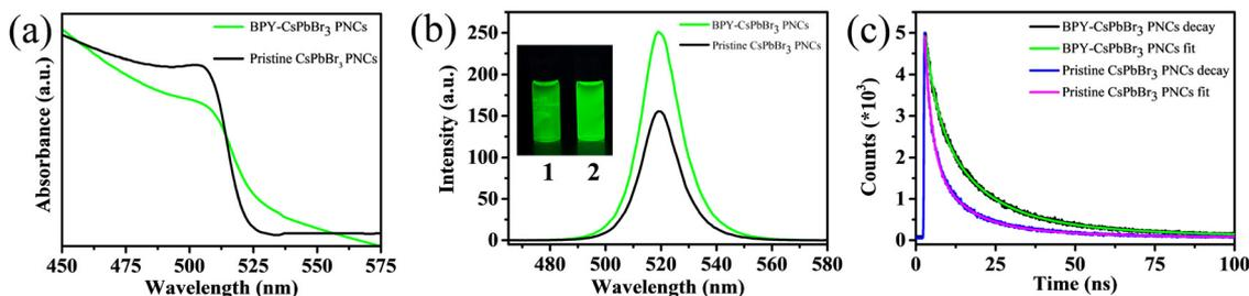
Fig. 2 (a) UV-Vis; (b) PL (inset shows the optical images of 1 pristine CsPbBr<sub>3</sub> PNCs and 2 BPY-CsPbBr<sub>3</sub> PNCs); (c) TCSPC spectra of pristine CsPbBr<sub>3</sub> PNCs and BPY-CsPbBr<sub>3</sub> PNCs.
