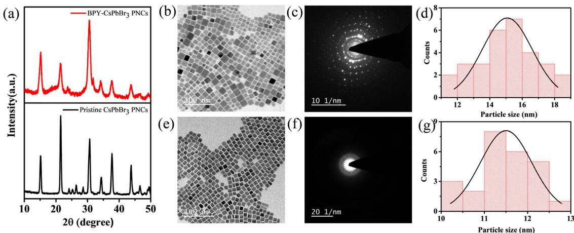
Fig. 1 (a) XRD pattern of BPY-CsPbBr<sub>3</sub> PNCs and pristine CsPbBr<sub>3</sub> PNCs; TEM images of (b) BPY-CsPbBr<sub>3</sub> PNCs, and (e) pristine CsPbBr<sub>3</sub> PNCs; SAED pattern of (c) BPY-CsPbBr<sub>3</sub> PNCs and (f) pristine CsPbBr<sub>3</sub> PNCs; particle size distribution curve of (d) BPY-CsPbBr<sub>3</sub> PNCs and (g) pristine CsPbBr<sub>3</sub> PNCs.
