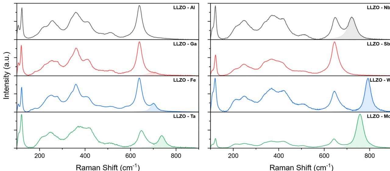
Fig. 5 Raman spectra of the supervalent doped LLZO pellets between 100–900  $\text{cm}^{-1}$ . The highlighted peaks at the high end of the spectrum are ascribed to the vibrational modes of the dopant–oxygen (M–O) bonds.
