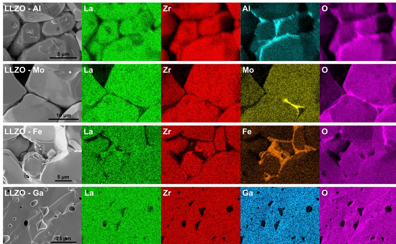
**Fig. 7** Cross-section EDS elemental maps of Al, Mo, Fe and Ga doped LLZO, showcasing the various distribution of doping elements.
