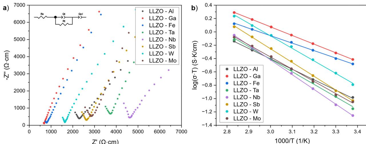
Fig. 8 (a) Nyquist plots of the supervalent doped LLZO pellets obtained at room temperature and (b) Arrhenius plots showing the temperature dependence on the total ionic conductivity of the LLZO pellets.
