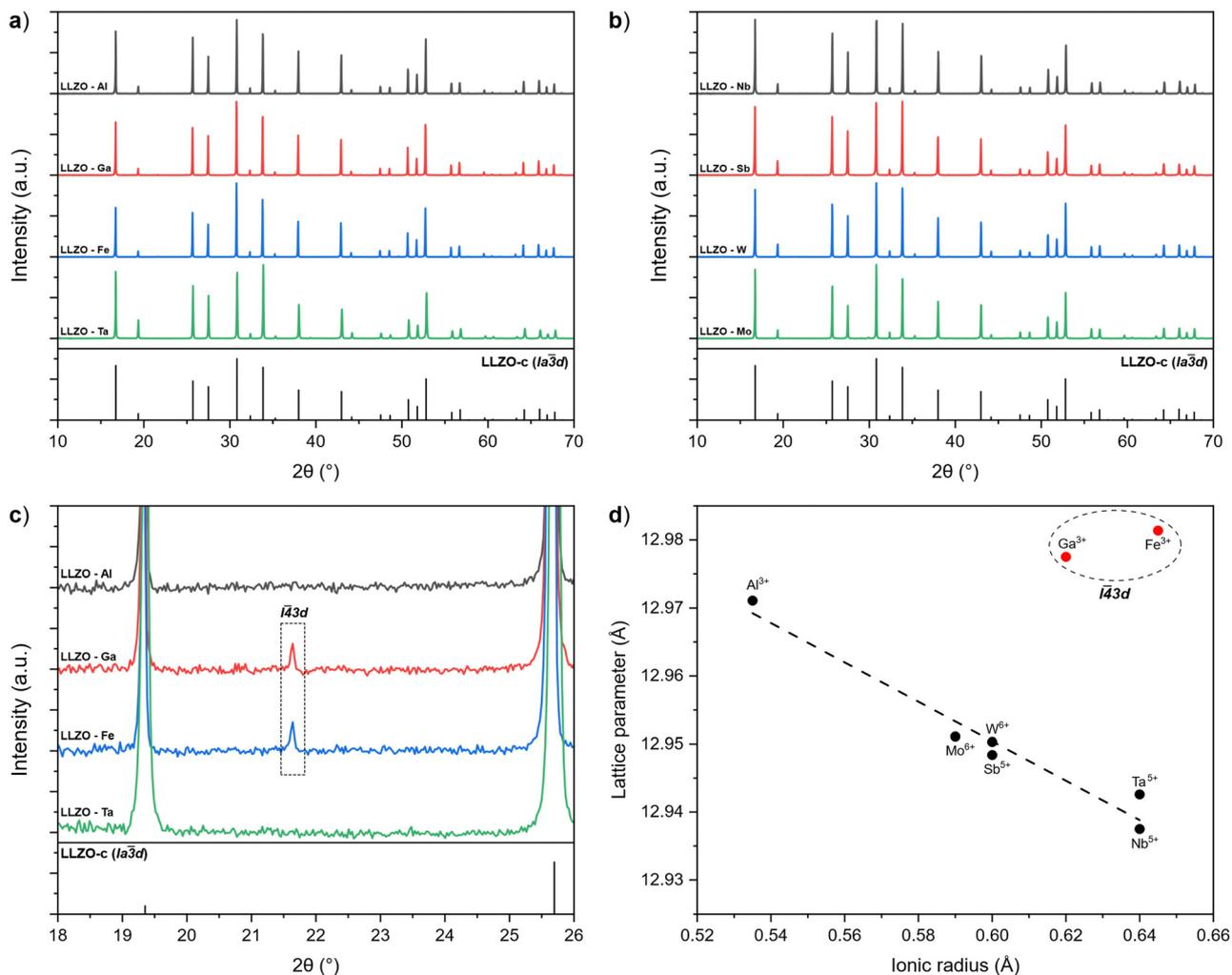
Fig. 3 (a) and (b) XRD patterns of supervalent doped LLZO pellets with the reference pattern for c-LLZO (ICDD #04-018-9023). (c) Partially enlarged XRD patterns showcasing the presence of a  $I\bar{4}3d$  symmetry peak for Ga and Fe doped LLZO. (d) Relationship between the lattice parameter of LLZO and the ionic radius of the corresponding dopant.<sup>60</sup>
