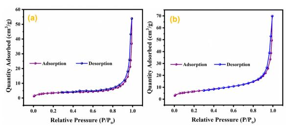
Fig. 9 BET isotherms of (a) MnO<sub>2</sub>, (b) Ag<sub>0.05</sub>MnO<sub>2</sub>.
