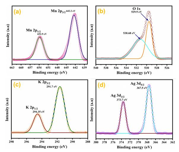
Fig. 7 XPS spectra of  $Ag_{0.05}MnO_2$  nanowires.
