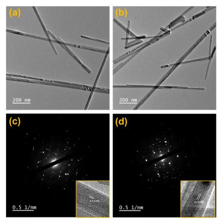
Fig. 5 (a) HRTEM image of MnO<sub>2</sub>, (b) HRTEM image of Ag<sub>0.05</sub>MnO<sub>2</sub>, (c) SAD pattern of MnO<sub>2</sub>, (d) SAD pattern of Ag<sub>0.05</sub>MnO<sub>2</sub>
