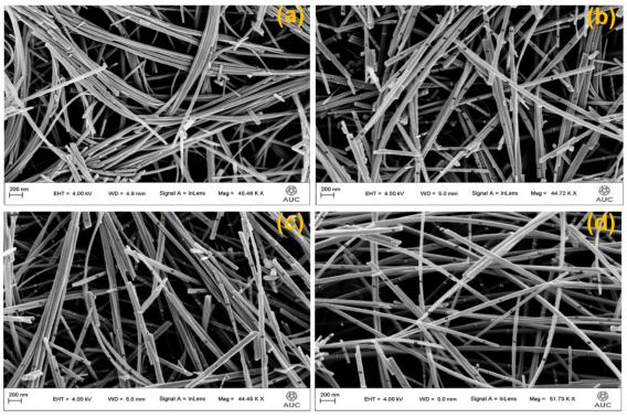
Fig. 4 FESEM images of (a) MnO<sub>2</sub>, (b) Ag<sub>0.05</sub>MnO<sub>2</sub>, (c) Ag<sub>0.10</sub>MnO<sub>2</sub>, (d) Ag<sub>0.15</sub>MnO<sub>2</sub>.
