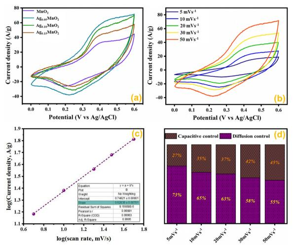
Fig. 10 (a) CV profile of  $Ag_xMnO_2$  NWs, (b) CV profile of  $Ag_{0.05}MnO_2$  at various scan rates, (c)  $\log i$  vs.  $\log \nu$  graph of  $Ag_{0.05}MnO_2$ , and (d) impact of the scan rate on the prominent charge storage process of  $Ag_{0.05}MnO_2$ .
