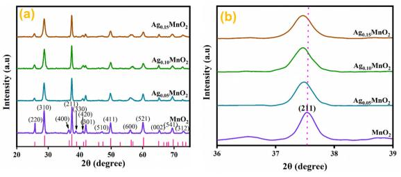
Fig. 2 (a) XRD patterns of bare and Ag doped MnO2 NWs, (b) enlarged view of diffraction peak from (211) diffraction plane
