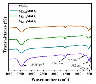
Fig. 3 FTIR spectra of Ag<sub>x</sub>MnO<sub>2</sub> NWs.
