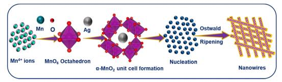
Fig. 1 A schematic illustration for the formation mechanism of Ag<sub>x</sub>MnO<sub>2</sub> NWs
