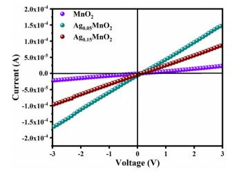
Fig. 8 I-V profiles of bare and doped MnO<sub>2</sub> NWs.
