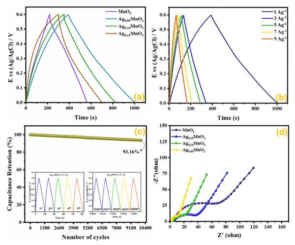
Fig. 11 (a) GCD curves of  $Ag_xMnO_2$ , (b) impact of varying current densities on GCD profile of  $Ag_{0.05}MnO_2$ , (c) capacitance retention after 10 000 GCD cycles (inset: first and last 5 cycles during cyclic test of  $Ag_{0.05}MnO_2$ ), and (d) EIS profile of  $Ag_xMnO_2$ .
