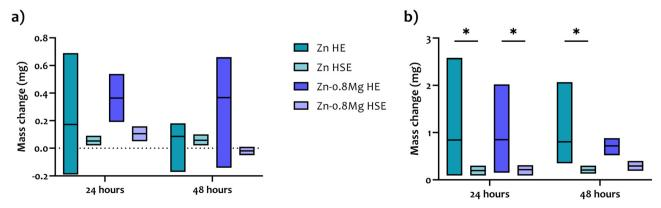
Fig. 3 Post-immersion mass change (a) with corrosion products and (b) after removal of corrosion products with chromic acid.
