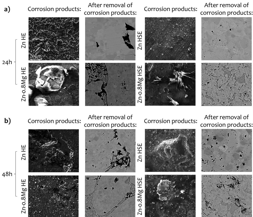
Fig. 4 SEM/BSE images of material surfaces with and without corrosion products observed after (a) 24 hours and (b) 48 hours of immersion in EBM. The scale bar, denoting 20  $\mu\text{m}$ , is inserted in the Zn HE 24 h image and remains consistent across all images.
