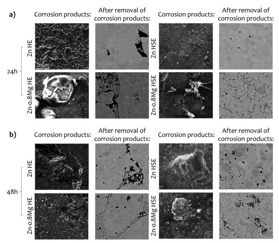
Fig. 4 SEM/BSE images of material surfaces with and without corrosion products observed after (a) 24 hours and (b) 48 hours of immersion in EBM. The scale bar, denoting 20 μm, is inserted in the Zn HE 24 h image and remains consistent across all images.
