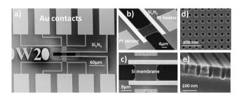
(a) Seebeck coefficient measurement device illustrating the Au pads connected to the heater/sensor and the 20  $\mu m$   $\times$  20  $\mu m$  Si membrane. (b) Close-up view of the suspended Si membrane and the Pt heater/sensor. (c) Top close-up view of the suspended PE Si membrane. (d) Details of the pore patterns on the Si membrane. (e) Cross-section view of the holes.
