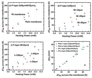
Fig. 6 Temperature difference across p-type silicon as a function of heating power for (a) P and PE membranes with dimensions 60  $\mu m$  in length and 10  $\mu m$  in width, (b) PE membranes with a fixed length of 60  $\mu m$ and varying widths, and (c) PE membranes with a fixed width of 10  $\mu$ m and varying lengths. (d) Absolute measured Seebeck voltage as a function of the temperature difference across different Si membranes
