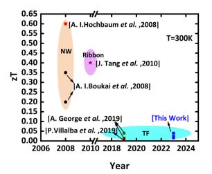
Fig. 1 Reported values of zT for crystalline nanostructure silicon planar configurations.
