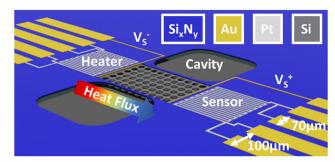
Fig. 2 Seebeck coefficient measurement device
