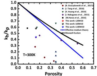
Fig. 9 The ratio of the phononic membrane to the thermal conductivity of the plain membrane as a function of the porosity. The graph includes experimental data from previous studies, as well as data from this current work, along with results obtained from effective medium theory and Maxwell-Fucken models
