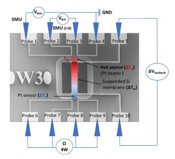
Fig. 5 Experimental setup for Seebeck coefficient measurement characterization
