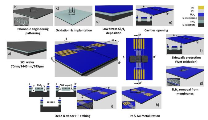
Fig. 3 Seebeck coefficient measurement device fabrication steps
