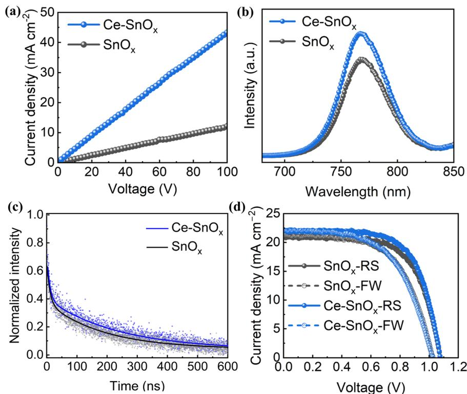
Fig. 3 (a) Current–voltage curves for calculating the conductivity of SnO<sub>x</sub> and 2.5 at% Ce-doped SnO<sub>x</sub>. (b) PL and (c) normalized TRPL spectra of FTO/SnO<sub>x</sub>/perovskite and FTO/Ce-SnO<sub>x</sub>/perovskite. (d)  $J$ - $V$  characteristics of the cells with pristine SnO<sub>x</sub> and 2.5 at% Ce-doped SnO<sub>x</sub> ETLs.
