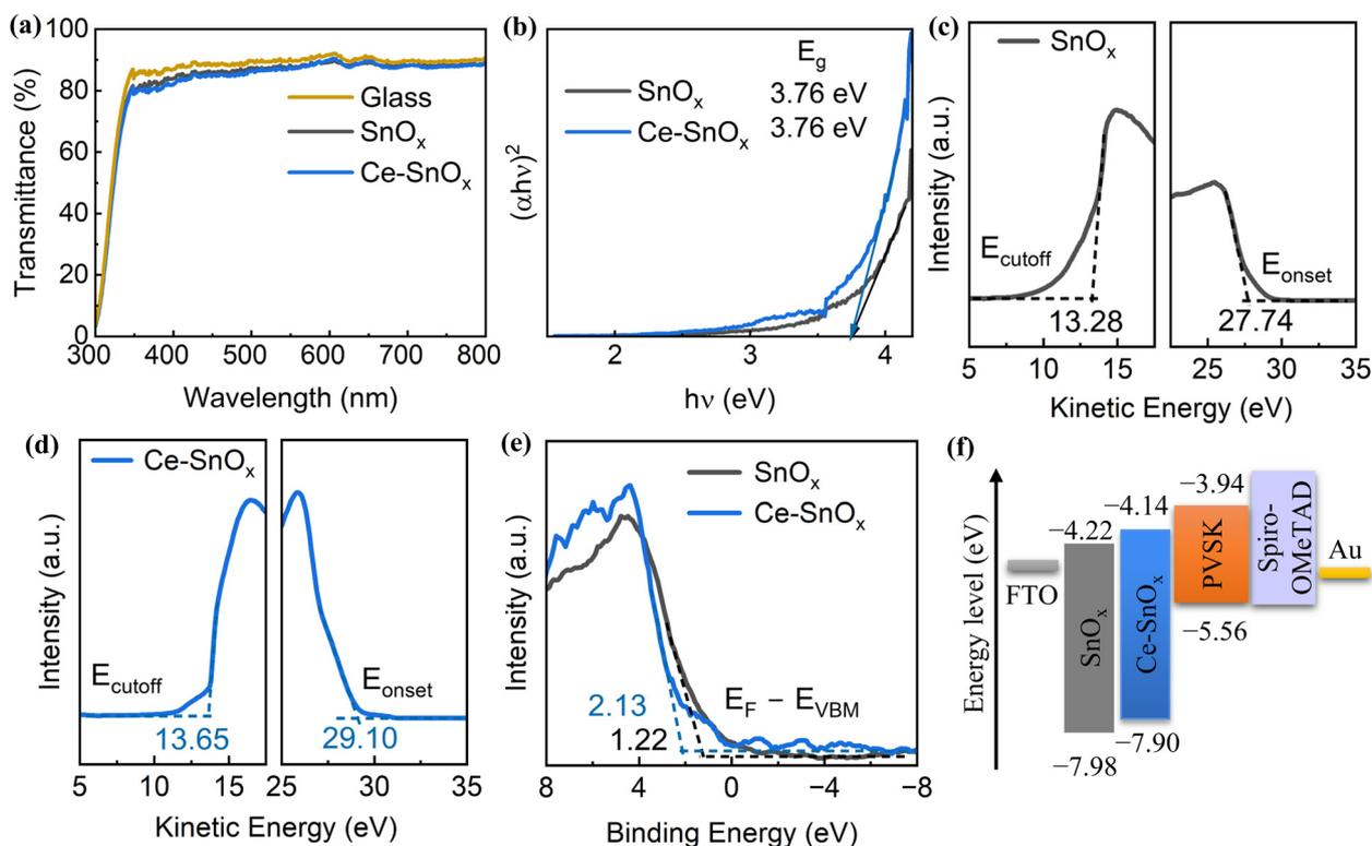
Fig. 2 (a) Transmittance, (b) Tauc's plots, (c) and (d) UPS spectra, and (e) valence band XPS spectra of pristine  $\text{SnO}_x$  and 2.5 at% Ce-doped  $\text{SnO}_x$ . (f) Energy band diagram of PSCs based on  $\text{SnO}_x$  and 2.5 at% Ce-doped  $\text{SnO}_x$  ETLs.
