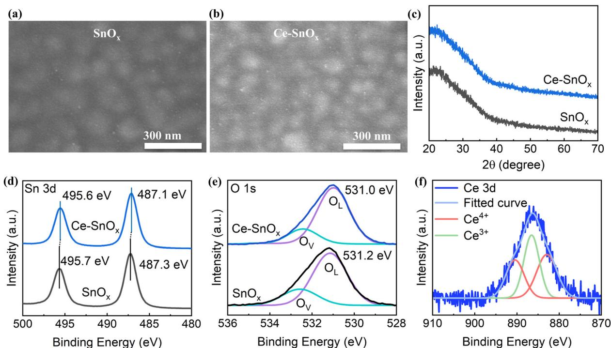
**Fig. 1** (a) and (b) Top-view SEM images, (c) XRD patterns, (d) Sn 3d XPS, and (e) O 1s XPS spectra of pristine and 2.5% Ce-doped  $\text{SnO}_x$ . (f) Ce 3d XPS spectra of 2.5% Ce-doped  $\text{SnO}_x$ .
