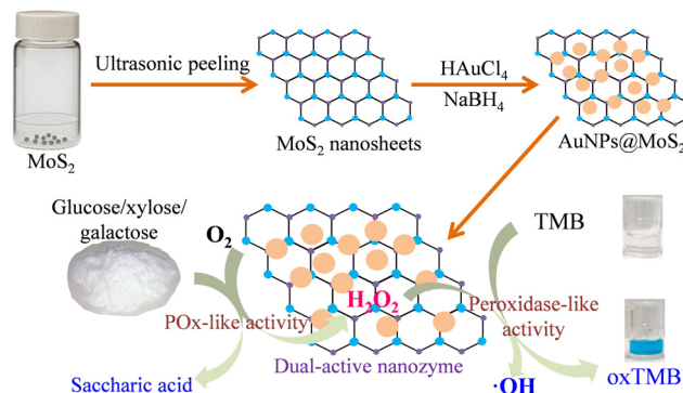
Scheme 1 Illustration of the experimental strategy for preparing AuNPs@MoS 2 with enhanced peroxidase-like and POx-like activities and the bio-enzyme-free colorimetric detection of glucose, xylose and galactose based on AuNPs@MoS 2 .
