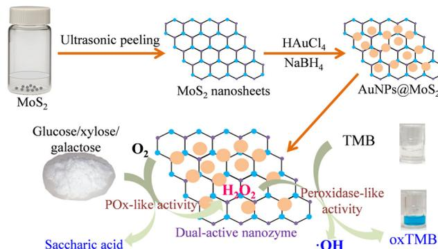
Scheme 1 Illustration of the experimental strategy for preparing AuNPs@MoS<sub>2</sub> with enhanced peroxidase-like and POx-like activities and the bio-enzyme-free colorimetric detection of glucose, xylose and galactose based on AuNPs@MoS<sub>2</sub>.
