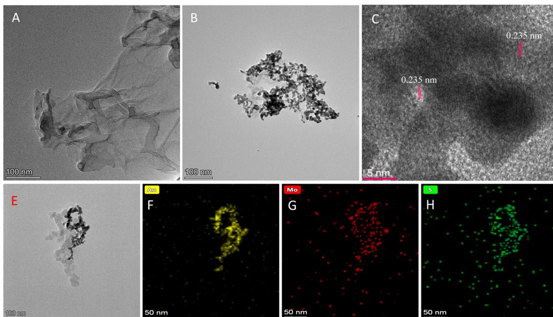
Fig. 1 The TEM image of the prepared MoS<sub>2</sub> nanosheets (A) and AuNPs@MoS<sub>2</sub> (B); the high-resolution TEM (HRTEM) image of AuNPs loaded on MoS<sub>2</sub> nanosheets (C); and the EDX mapping images of AuNPs@MoS<sub>2</sub> (E)–(H).
