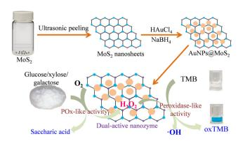
Scheme 1 Illustration of the experimental strategy for preparing AuNPs@MoS2 with enhanced peroxidase-like and POx-like activities and the bio-enzyme-free colorimetric detection of glucose, xylose and galactose based on AuNPs@MoS>
