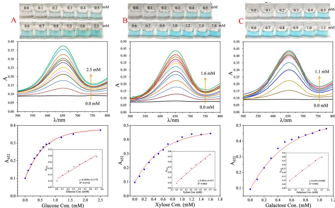
Fig. 3 Photographs, UV-visible spectra and linear relationships between  $A_{652}$  and analyte concentrations for detecting different concentrations of glucose (A), xylose (B) and galactose (C) with the corresponding colorimetric method. Data were obtained using the optimal selection described in the text.
