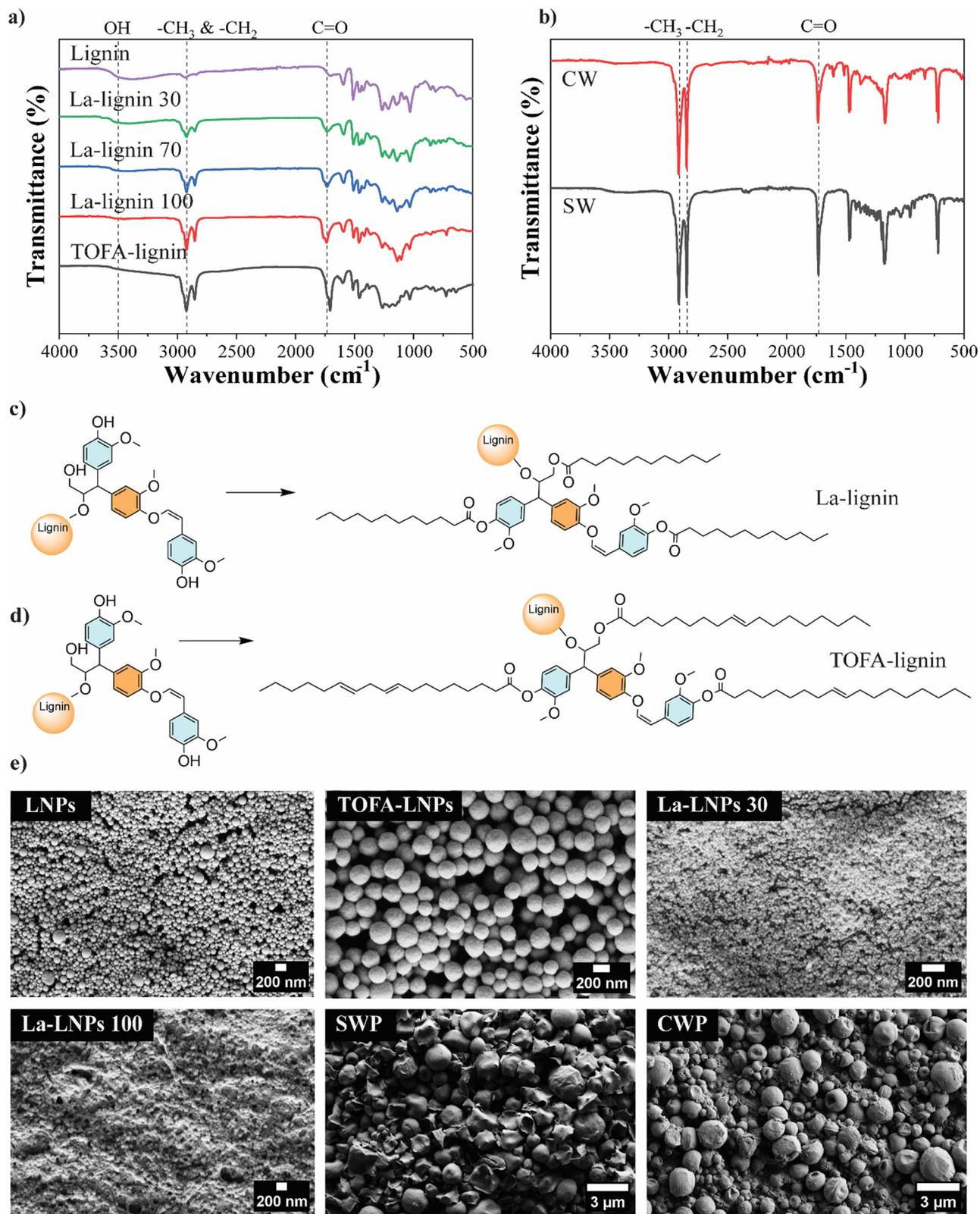
**Fig. 2** Chemical characterization of polyaromatic material and morphology of the respective nanoparticle coatings on CNF freestanding films. FTIR spectra of (a) unmodified, esterified lignins, and (b) carnauba and spruce needle waxes. A schematic presentation of lignin esterification by (c) lauric acid chloride and (d) TOFA-chloride. (e) SEM images of CNF freestanding films functionalized with LNPs, TOFA-LNPs, La-LNPs<sub>30</sub>, La-LNPs<sub>100</sub>, CWPs, and SWPs.
