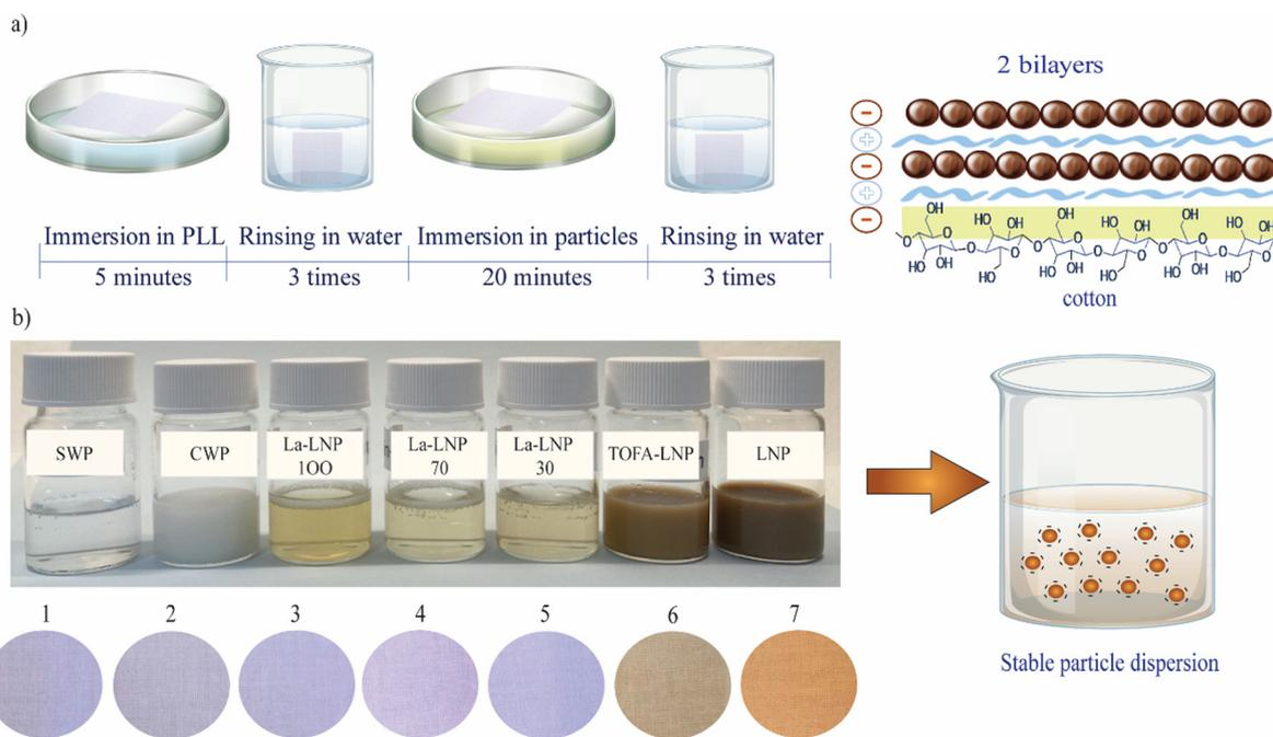
**Fig. 1** Illustration of the layer-by-layer procedure for functionalization of the cellulosic substrates. (a) Photographs of aqueous nanoparticle dispersions and cotton fabrics functionalized with the respective NP dispersions. (b) The NP samples from 1–7 are (1) SWPs, (2) CWPs, (3) La-LNPs<sub>100</sub>, (4) La-LNPs<sub>70</sub>, (5) La-LNPs<sub>30</sub>, (6) TOFA-LNPs and, (7) LNPs.
