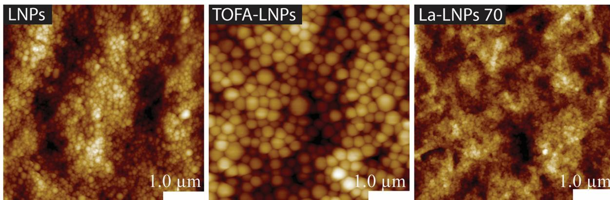
Fig. 4 AFM height images of functionalized freestanding films with LNP, TOFA-LNP, and La-LNP<sub>70</sub> coatings.
