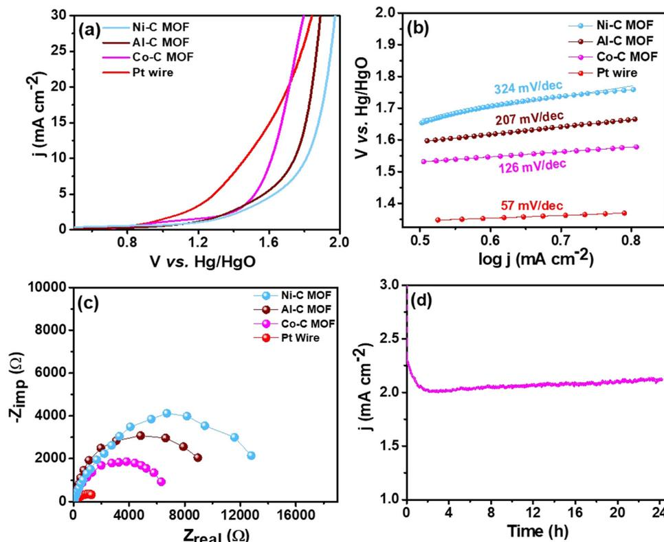
Fig. 9 (a) LSV curves of Al, Co and Ni-C MOFs and the Pt electrocatalyst at  $50 \text{ mV s}^{-1}$  in 10% acetonitrile with 2 mM dibenzothiophene, (b) and (c) Tafel slope and EIS spectra of the catalysts and (d) CA stability study.
