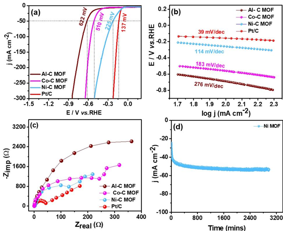
Fig. 10 (a) LSV curves of Al, Co and Ni-C MOFs and Pt-C at the scan rate of  $50 \text{ mV s}^{-1}$  in  $1 \text{ M KOH}$ , (b) and (c) Tafel slope and EIS spectra of the catalysts and (d) CA stability study.
