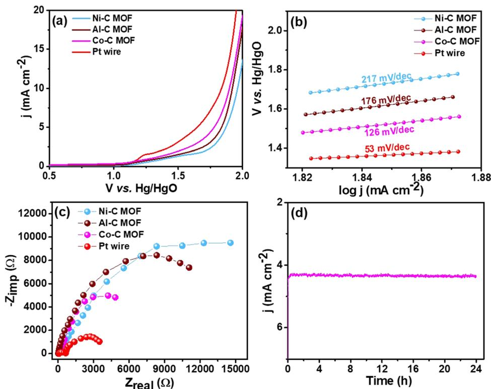
Fig. 8 (a) LSV curves of Al, Co and Ni-C MOF and the Pt electrocatalyst at the scan rate of  $50 \text{ mV s}^{-1}$  in  $0.5 \text{ M H}_2\text{SO}_4$  with  $2 \text{ mM BT}$ , (b) and (c) Tafel slope and EIS spectra of the catalysts and (d) CA stability study.
