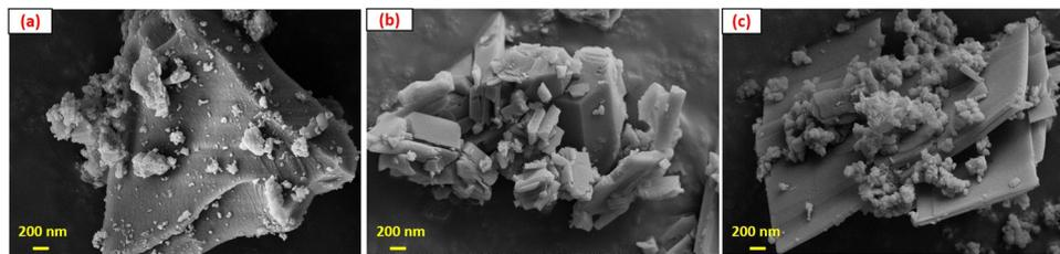
Fig. 3 FE SEM images of synthesized (a) Co, (b) Al and (c) Ni-C MOFs.
