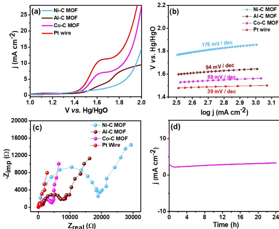
Fig. 7 (a) LSV curves of the Pt wire electrocatalyst, Al, Co and Ni-C MOF in  $0.5 \text{ M H}_2\text{SO}_4$  with  $2 \text{ mM TP}$  at a scan rate of  $50 \text{ mV s}^{-1}$ , (b) & (c) Tafel slope & EIS spectra and (d) CA stability study.
