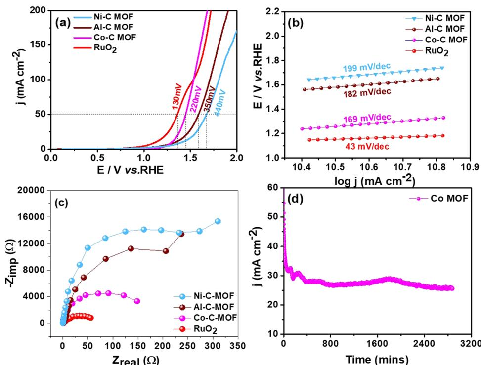
Fig. 11 (a) LSV curves of Al, Co and Ni-C MOFs and  $\text{RuO}_2$  at the scan rate of  $50 \text{ mV s}^{-1}$  in  $1 \text{ M KOH}$ , (b) and (c) Tafel slope and EIS spectra of the catalysts and (d) CA stability study.
