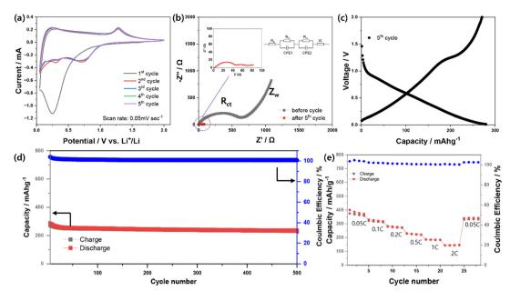
Fig. 3 (a) Cyclic voltammetry and (b) EIS characteristics of MSNC (Li/MSNC cell). (c) Discharge/charge profiles, (d) cyclability test cycled between 0.05 and 2 V versus Li<sup>+</sup>/Li with 0.2C, and (e) C-rate test from 0.05C to 2C.
