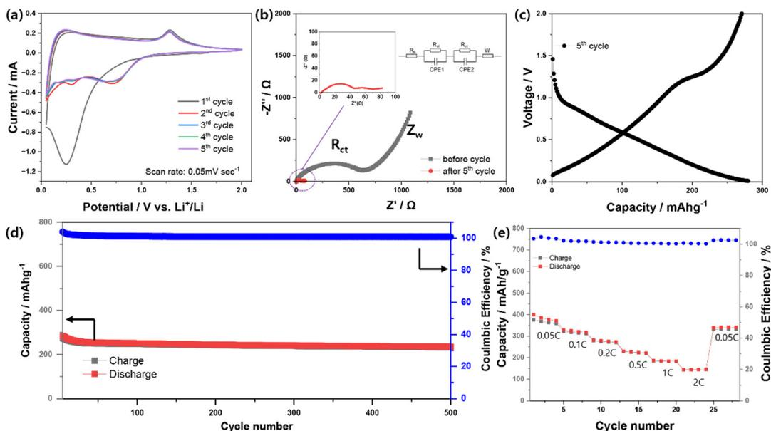
Fig. 3 (a) Cyclic voltammety and (b) EIS characteristics of MSNC (Li/MSNC cell). (c) Discharge/charge profiles, (d) cyclability test cycled between 0.05 and 2 V versus  $\text{Li}^+/\text{Li}$  with 0.2C, and (e) C-rate test from 0.05C to 2C.
